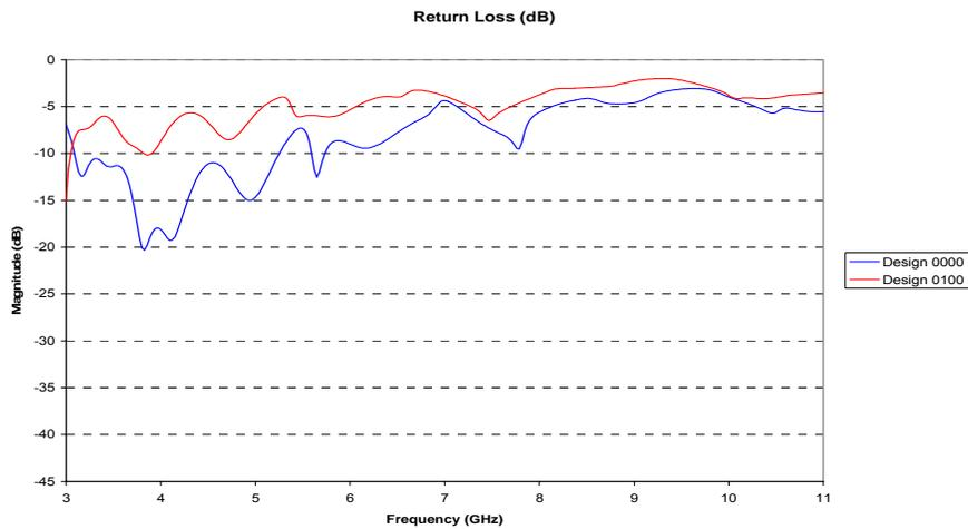
**Figure 4.3.9.** Return Loss Response for DOE III Design 0000 and Design 0100.
