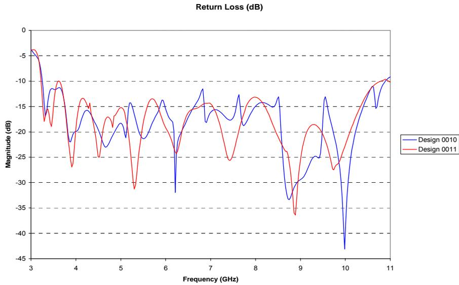
**Figure 4.4.8.** Return Loss Response for DOE IV Design 0010 and Design 0011.
