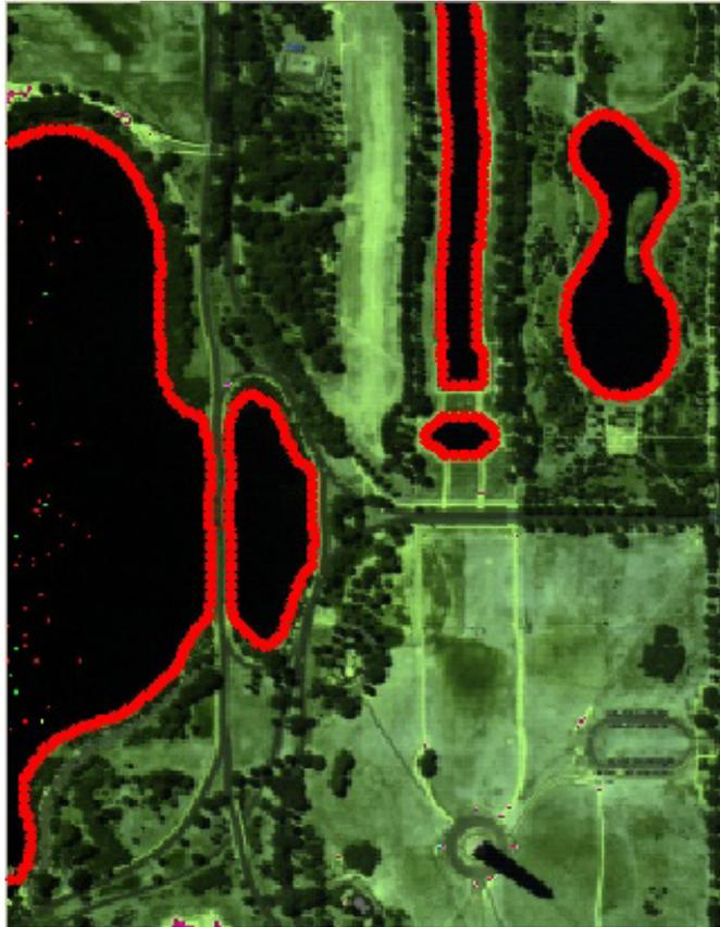
**Figure 4-10: Regions selected from Washington D.C. Mall. Segmentation generated (bands 177 171 136 RGB) using 15 points of the object of interest, threshold=16 and CN=3.**
