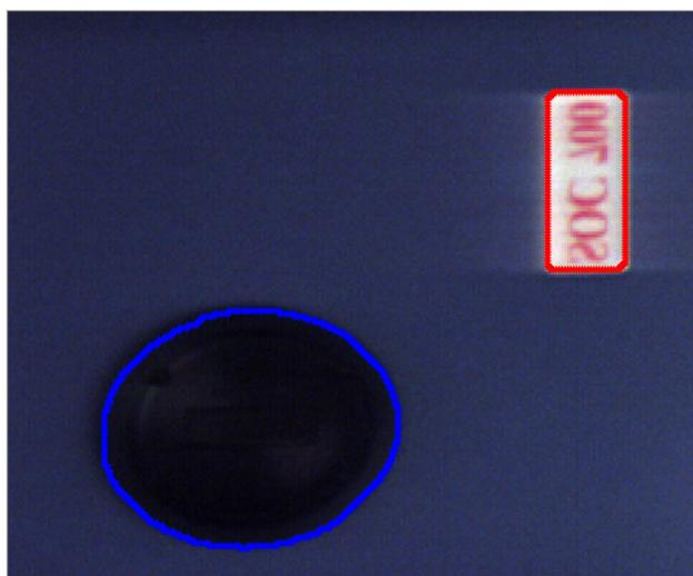
**Figure 4-5: Region selected from Fake Leaves hyperspectral image captured by SOC-700. Segmentation generated (bands 40 35 15 RGB) using 10 points for the first object(blue) and 5 point for the second object(red), for both threshold=10 and CN=3.**
