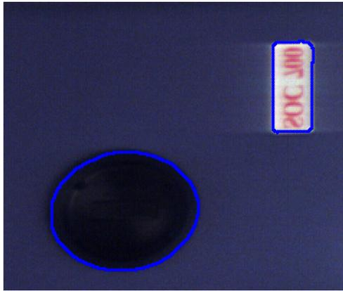
**Figure 4-25: Region selected from Fake Leaves hyperspectral image captured by SOC-700. Segmentation generated (bands 57 36 13 RGB) using 8 points for the first object(round) and 7 point for the second object(rectangular), for both threshold=10 and CN=3.**
