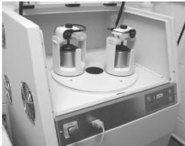
Figure 2.2 Fritsch Pulverisette P4™ Vario-planetary ballmilling machine with two vials mounted on supporting disk [9]
