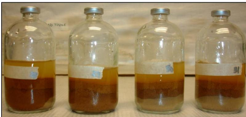
**Figure 3.5. Static batch reactors with clay during test.**
