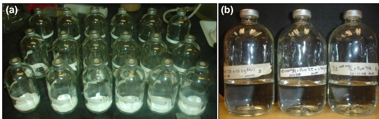
**Figure 3.4. Static batch reactors: Vials with measured amount of salt (a), reactors with three different sodium chloride concentrations during test (b).**
