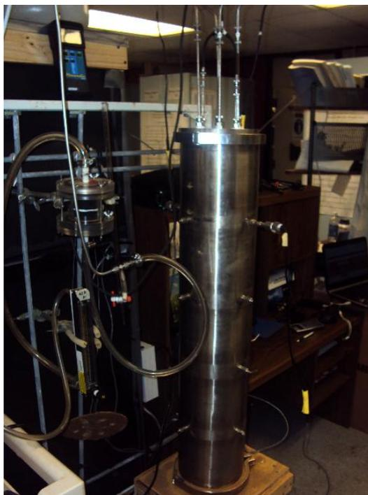
**Figure 3.13. Preliminary test bed setup: stainless steel column.**
