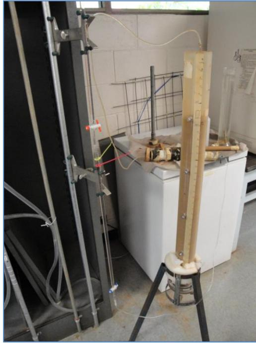
**Figure 3.7. Capillary-based delivery experimental setup.**
