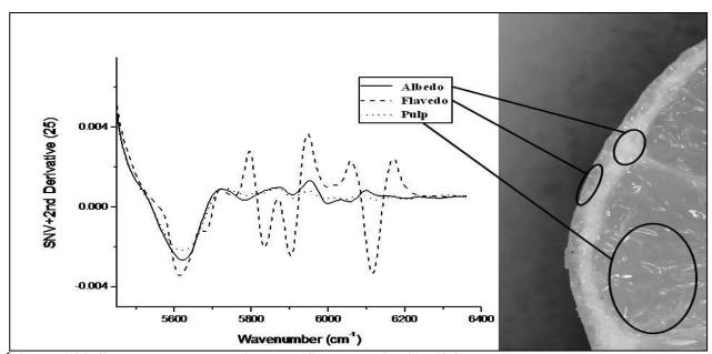
(Figure 6.4.2 Standard Normal Variate and Second Derivative of flavedo, albedo and pulp. In a second derivative the most intense peaks are actually lower and viceversa. The substance with the most intense peaks downwards is strongly suggesting a dominance in composition. The flavedo is showing an extraordinary dominance near 6100cm-1 were bond insaturation (as in terpenes) is expected to reflect.
