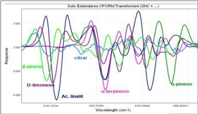
Figure 6.4.7 SNV and 2nd derivative treated terpene standard spectra.
