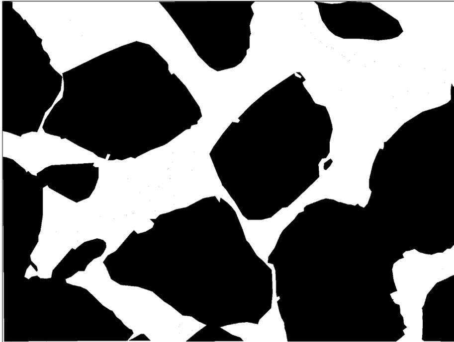
**Figure 4-14.** Surface micrograph classified using ImageJ
