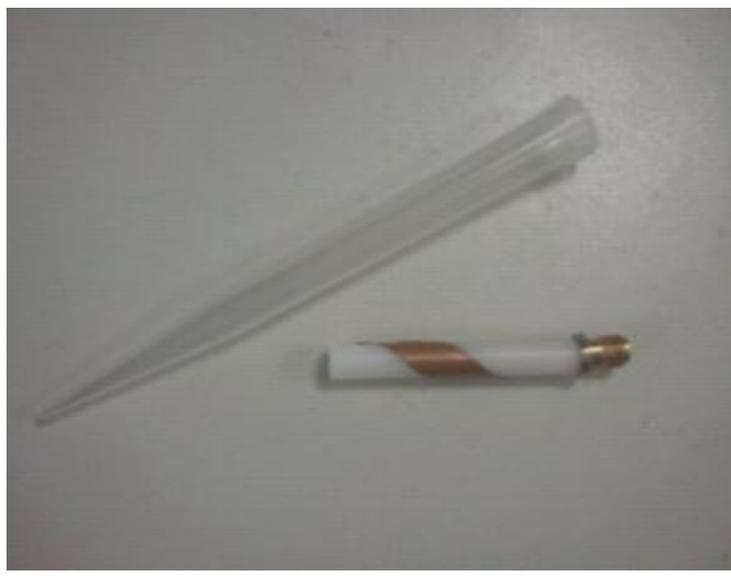
**Figure 4.19 Protective Well-Casing Pipe With the Constructed Helix Antenna Used in the S-parameters Measurements.**
