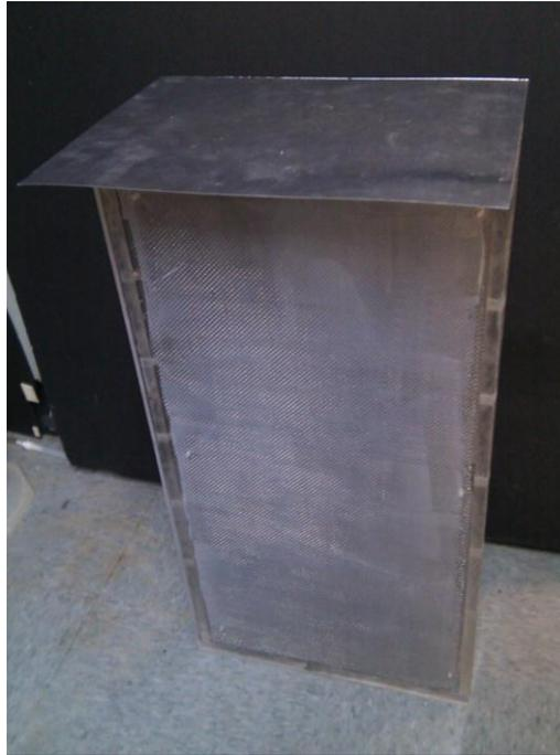
**Figure 3.16 Illustration of the Constructed Testbed With a Metal Plate Placed at Top of the Testbed Used for the S-parameters Measurements.**
