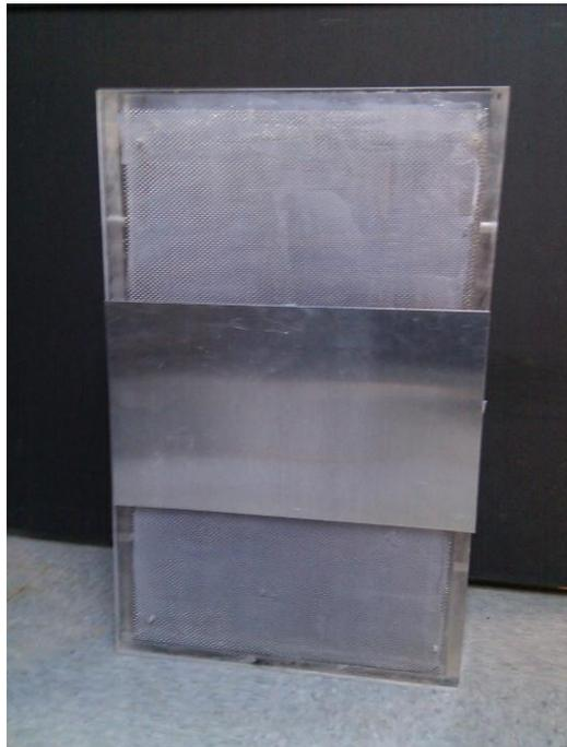
**Figure 3.17 Illustration of the Constructed Testbed With Horizontal Metal Plates Placed at the Faces of the Mesh Plates of the Testbed Used for the S-parameters Measurements.**
