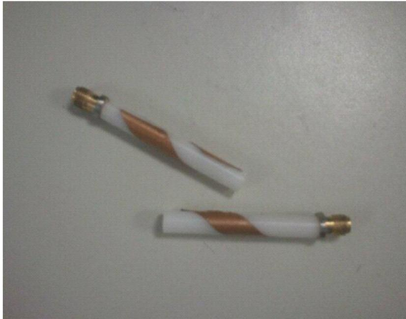
**Figure 3.7 Fabricated Helix Antennas Made With Delrin Rod, Copper Strip, and SMA Connectors.**
