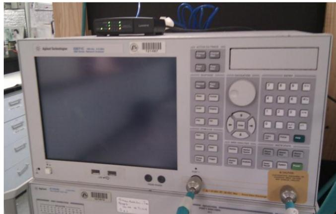
**Figure 3.9 Agilent's Vector Network Analyzer Model ENA 5071C.**
