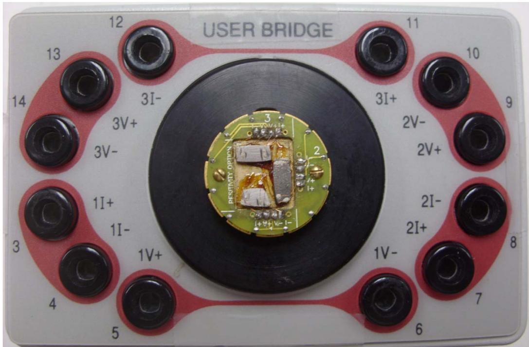
**Figure 3.6.** Sample puck used to resistivity measurement.
