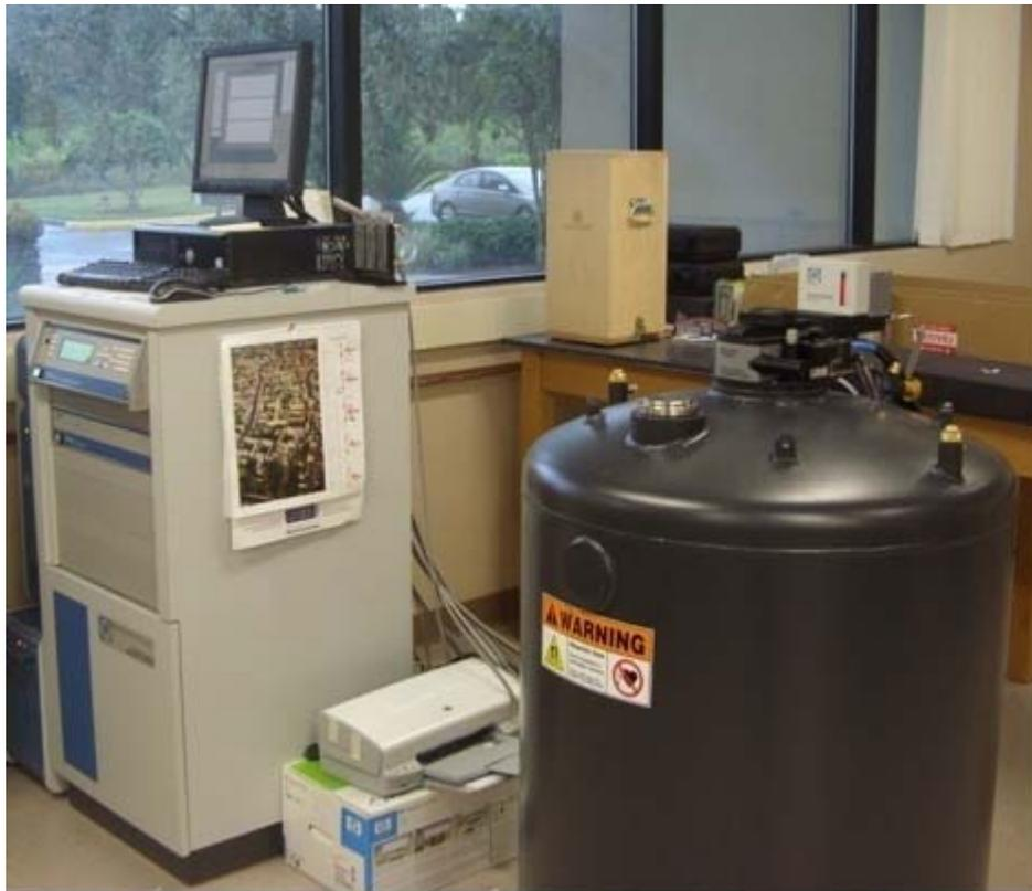
**Figure 3.5.** Physical Property Measurement System.
