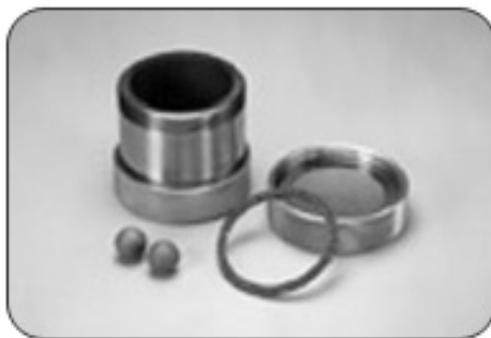
**Figure 3.1.** Jar and balls used in the ball milling process.
