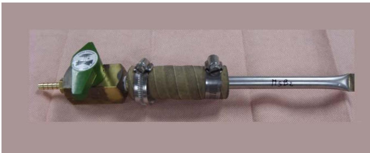
**Figure 3.3.** Mechanism to protect the sample and connect it with the vacuum system.
