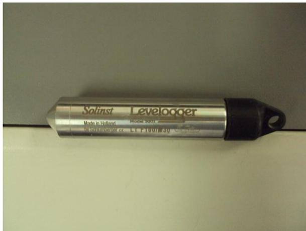
**Figure 51: Levelogger device**
