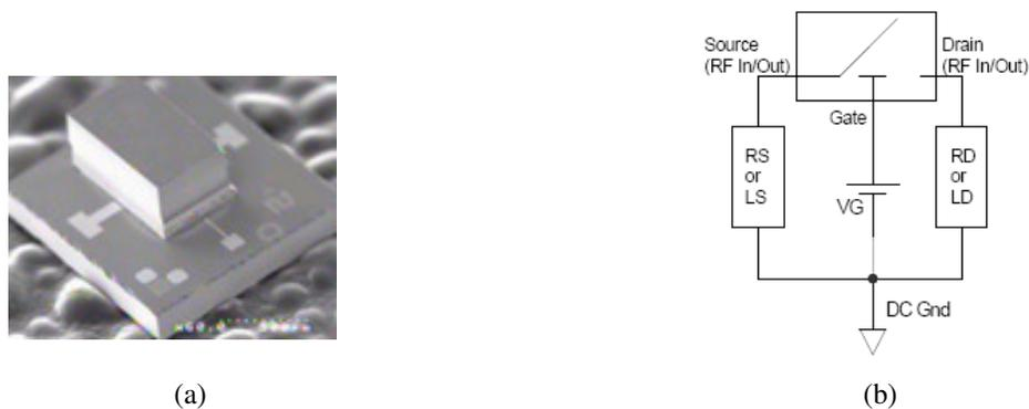
Figure 5.19 (a) RF-MEMS switch used in the antenna subsystem and (b) the protection circuit recommended for safe dissipation of the charge build-up [65].
