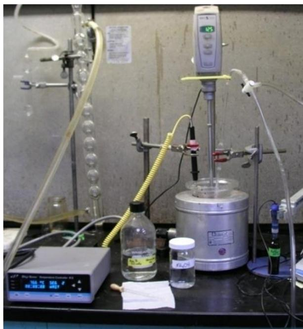
Figure 1. Co-precipitation synthesis setup under  $\text{N}_2$  controlled atmosphere.
