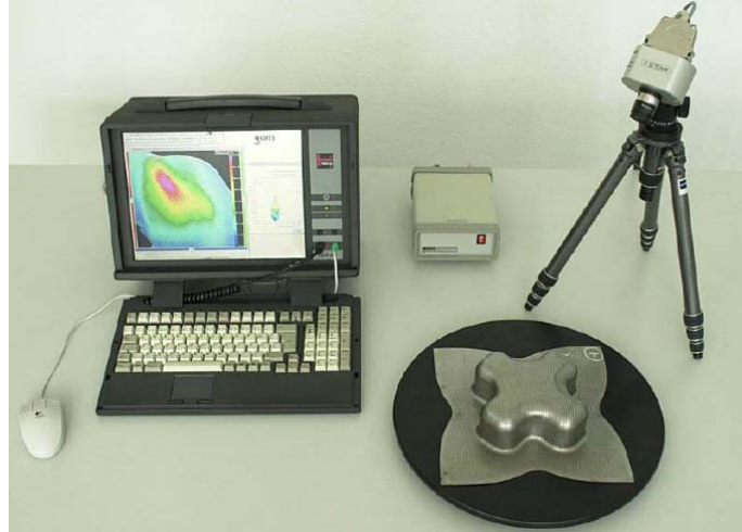
Figure 2.13 3-dimensional DIC surface strain measurement system [28].
