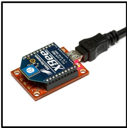
Figure 4-18 XBee Coordinator Node
