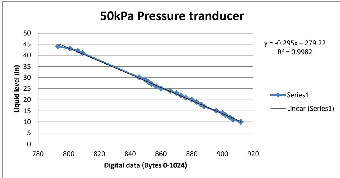
Figure 5-2 Experimental data for the 50kPa pressure transducer
