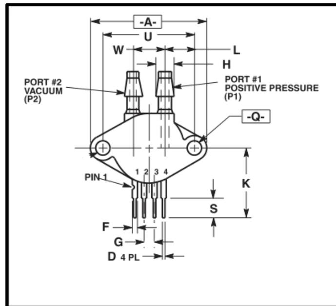
Figure 4-1 MPX2010DP Pressure Transducer Schematic
