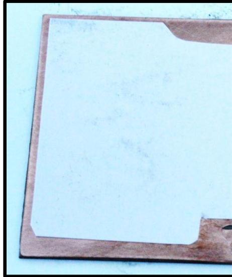
**Figure 4-10 Toner print aligned with Copper Board**
