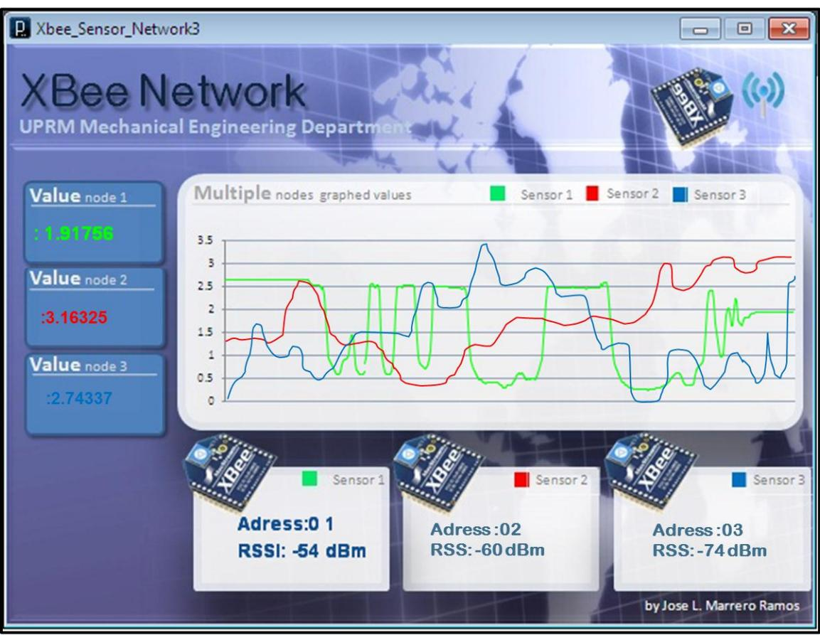
Figure 5-3 Wireless Sensor Network GUI, For 3 XBee Nodes
