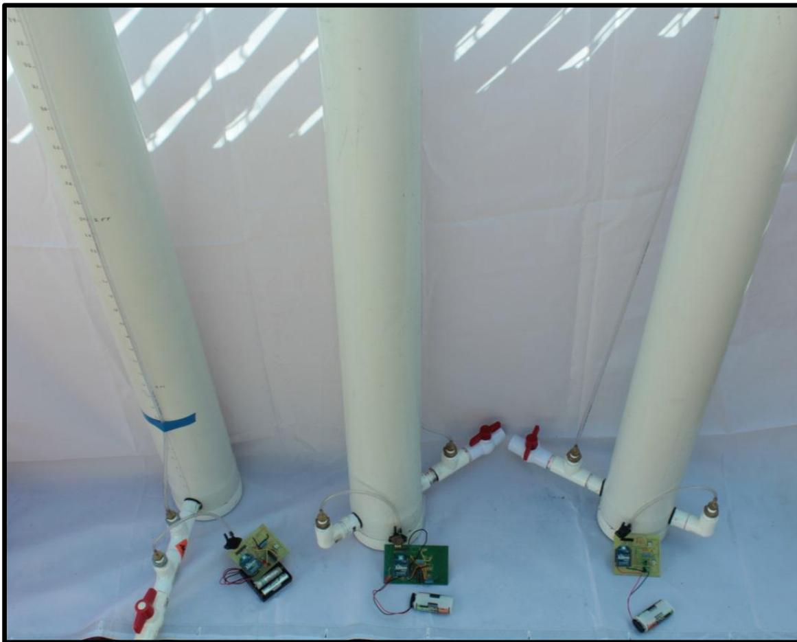
Figure 6-8 Experimental setup with 3 water tanks
