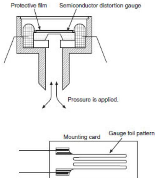
**Figure 4-3 Semiconductor Distortion Gauge Construction**
