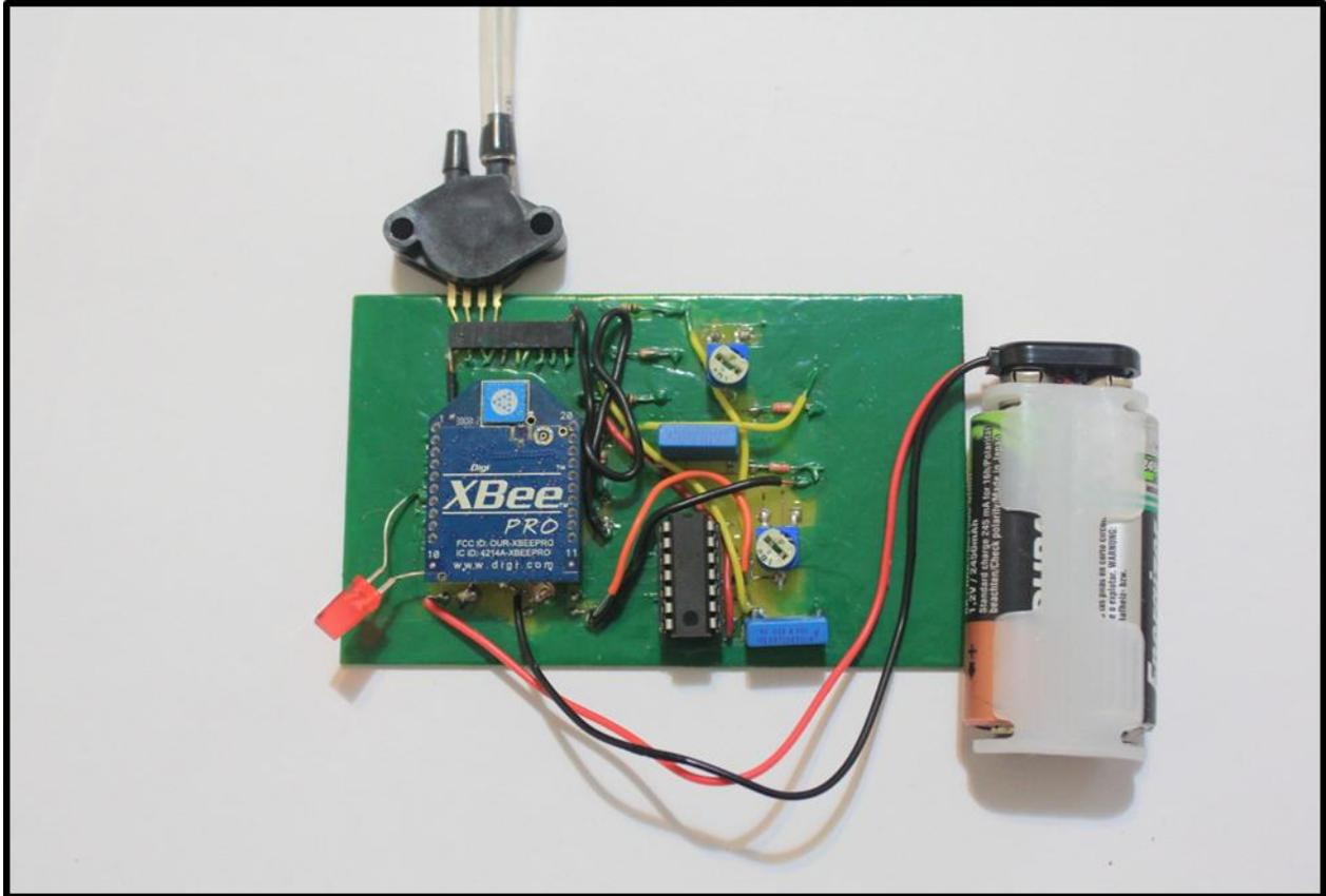
Figure 4-16 Wireless Node with AA Battery
