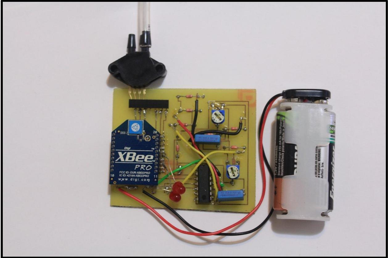
Figure 4-14 Wireless node setup with AA batteries
