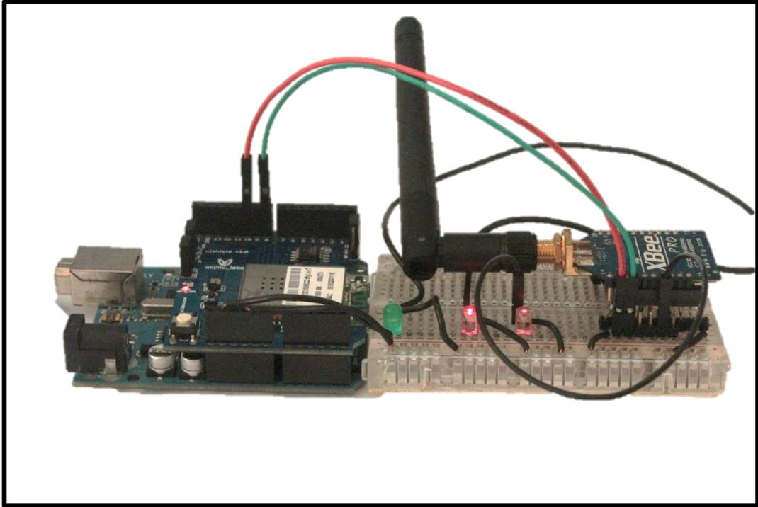
Figure 4-20 Arduino Coordinator Node
