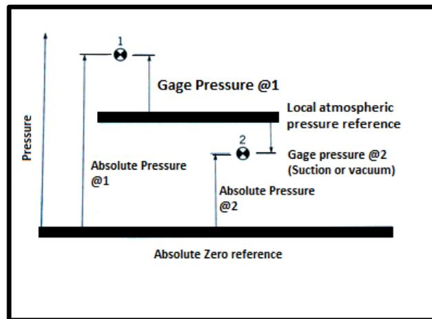
Figure 2-6 Graphical Representation of Gage and Absolute Pressure
