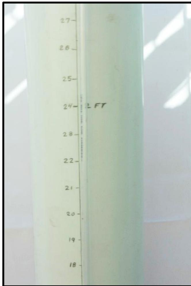
**Figure 6-9 Tank plastic tube for visual measures**
