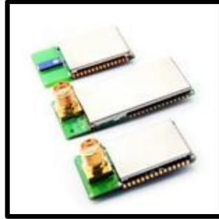
Figure 2-10 ZigBee / 802.15.4 Modules WIRELESS MCU IEEE802.15.4 TRNSCVR
