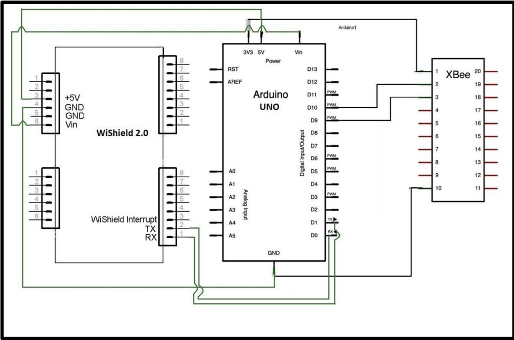
Figure 4-19 Arduino Coordinator Node Schematics
