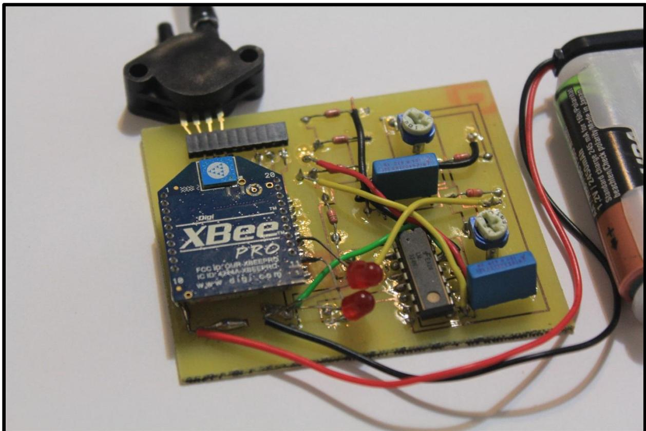
Figure 4-13 Wireless node without solder mask
