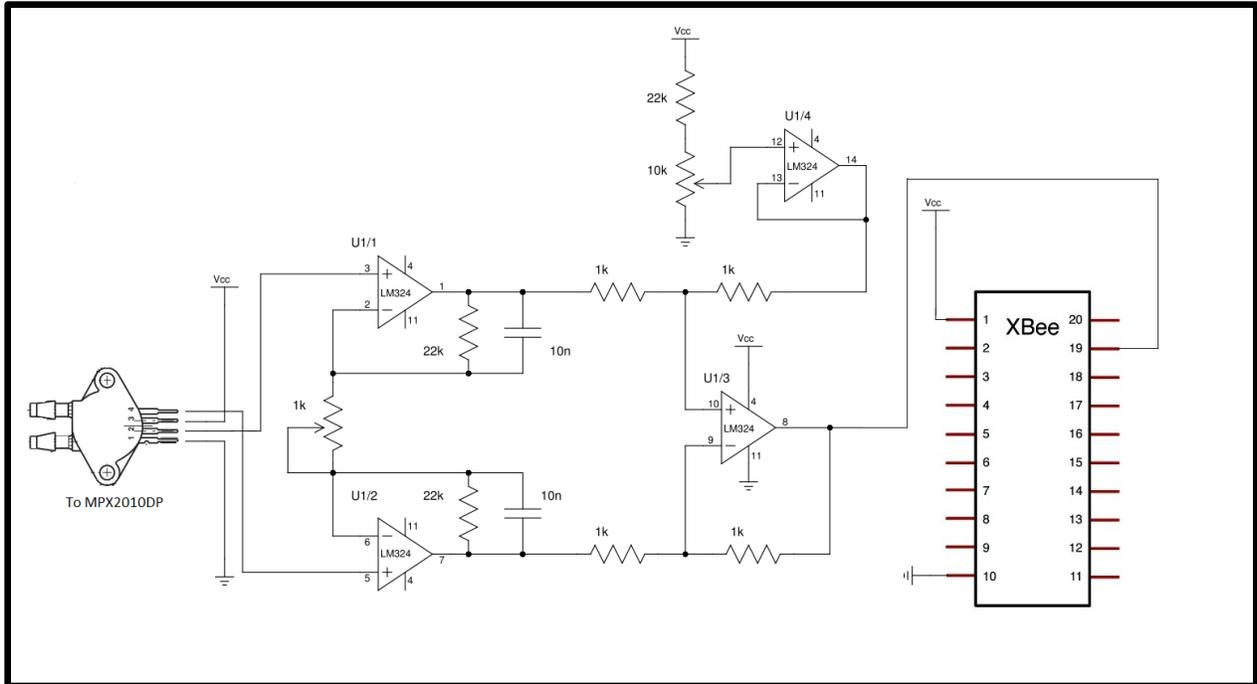
**Figure 4-7 Remote Node with Pressure Transducer and amplification circuit**
