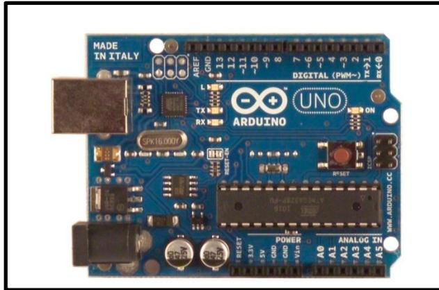
Figure 2-16 Arduino Microcontroller
