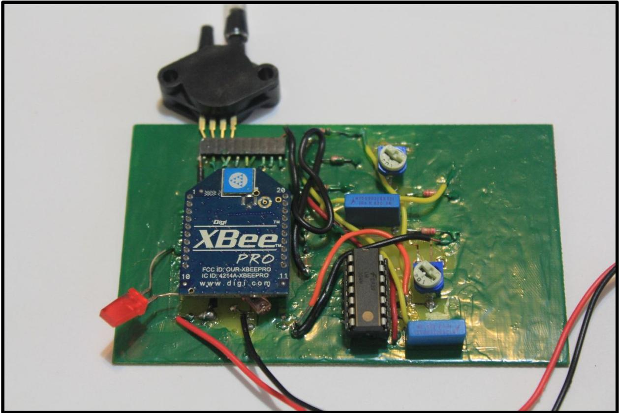
**Figure 4-15 XBee wireless node with solder mask**
