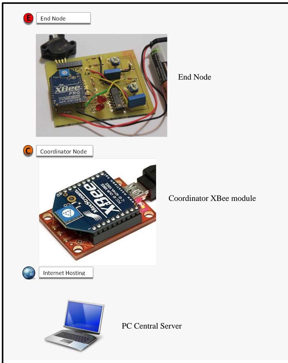
Figure 6-2 Wireless Sensor Network Components with PC-Based Central Server
