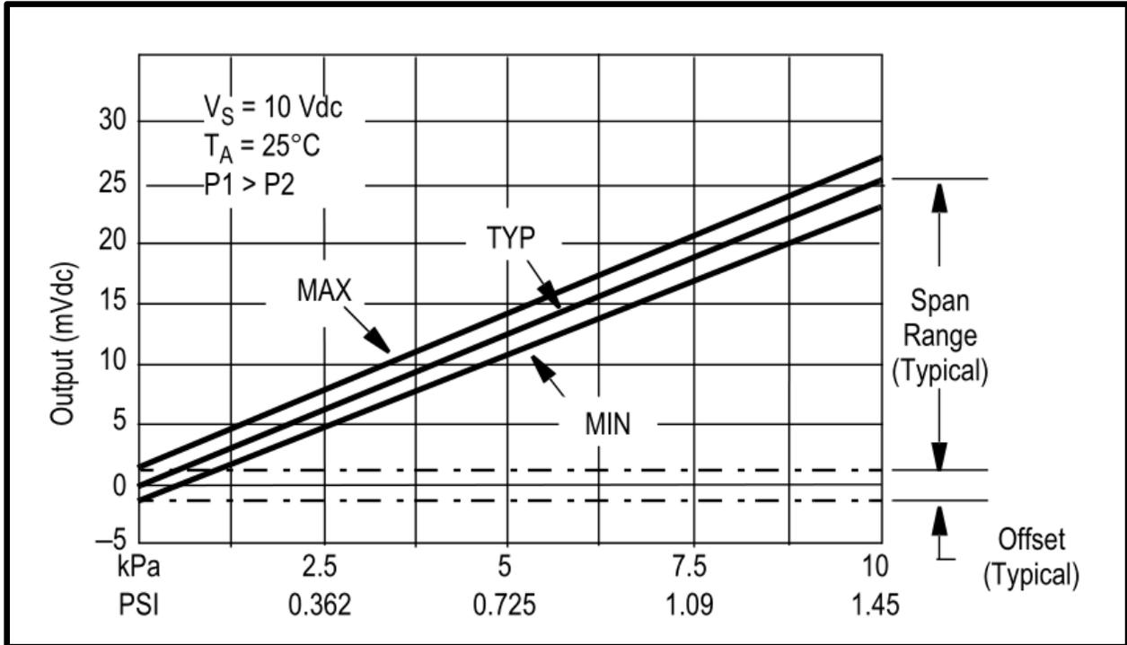
Figure 4-6 Output vs. Pressure Differential for Pressure Transceiver
