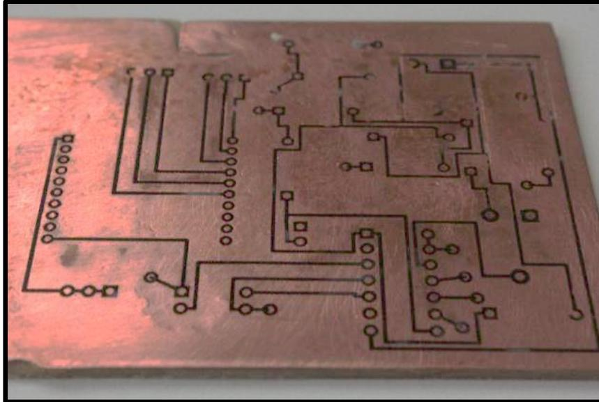
**Figure 4-12 Toner Routes Adhered to Copper Plate**
