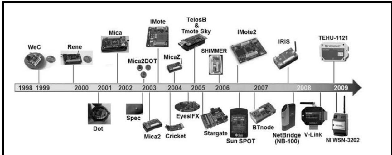
Figure 2-11 Timeline for wireless nodes platform [2]
