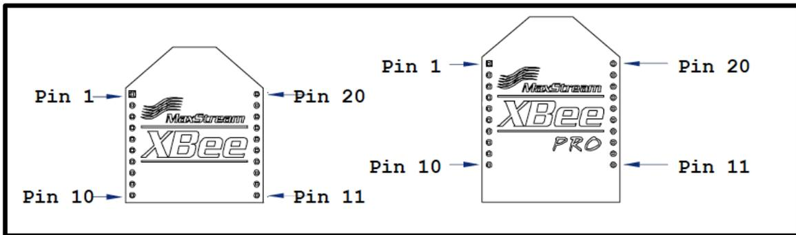
Figure 2-13 XBee and XBee-Pro Modules Pin Localization Diagram
