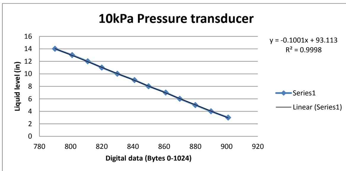
Figure 5-1 Experimental results for the 10kPa pressure transducer
