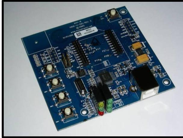
**Figure 2-15 MaxStream USB 2.0 board**
