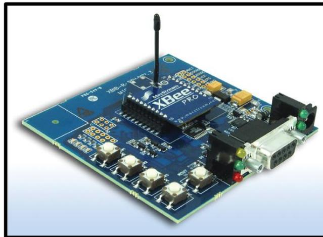
Figure 2-14 MaxStream RGB board
