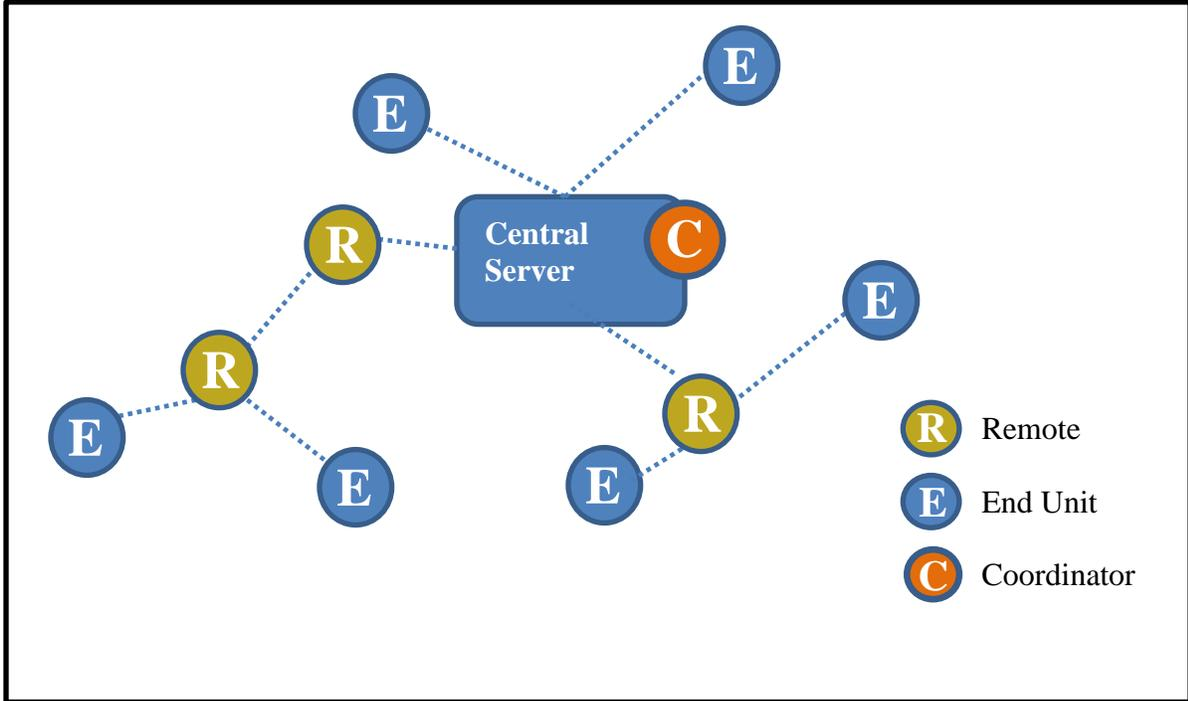
Figure 3-1 Multi-Hop Multi-Point to Point Network
