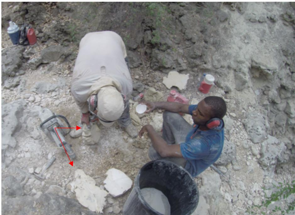
Figure 11: Cutting the sides of the coral with a portable saw and leaving a central core of the skeleton managed to volume and weight of the coral sample. The red arrows shows examples of processed coral samples. (Photo by: W. Ramirez, 2014).
