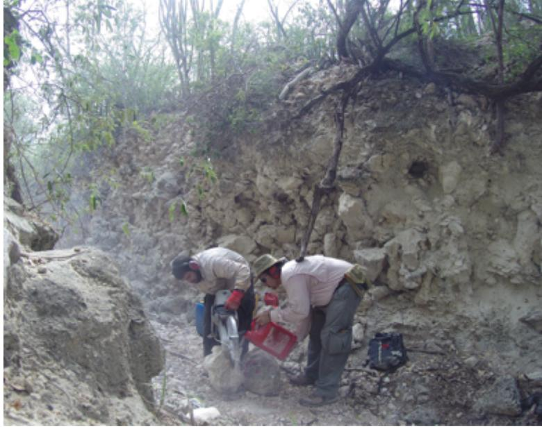
Figure 12: Cutting the coral heads with the portable saw at Cañada Honda. Large amounts of water were carried to the field to assist in the process. (Photo by: W. Ramirez, 2014)
