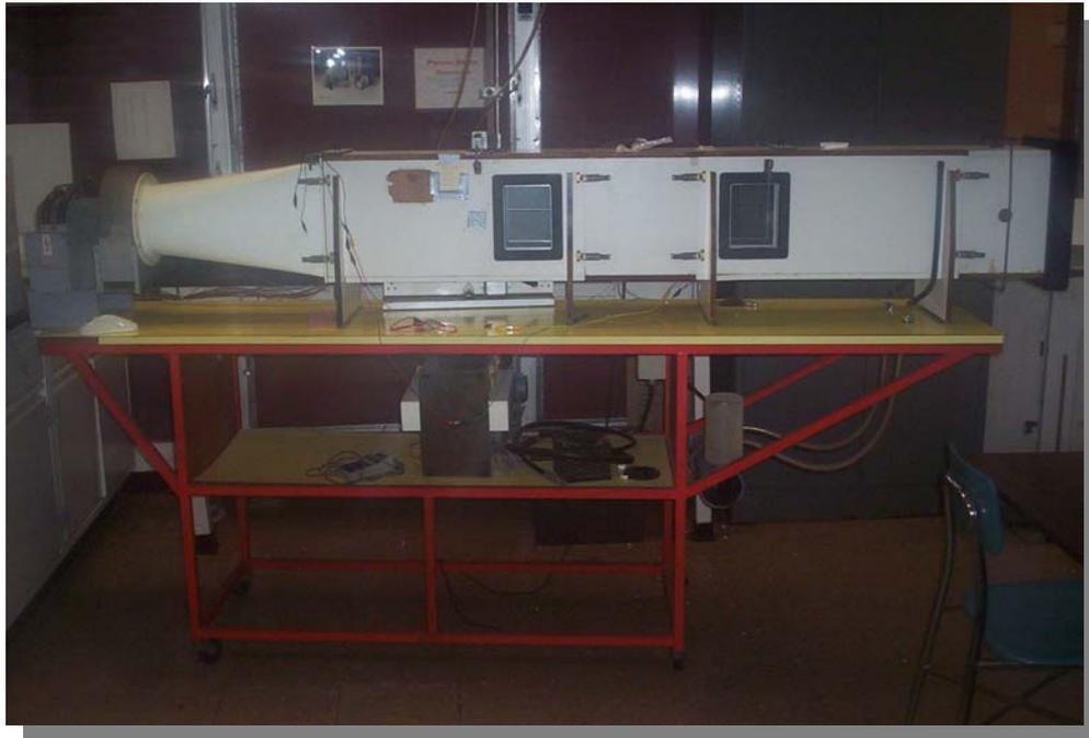
**Figure 4.3 Wind tunnel.**
