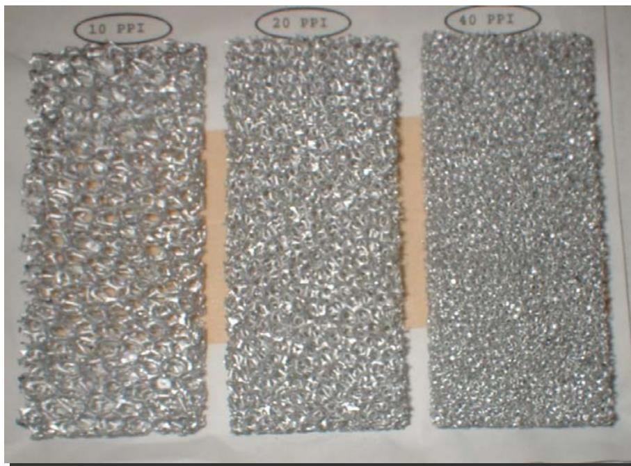
**Figure 1.3 10, 20 and 40 PPI metal foam samples.**
