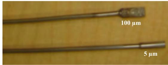
**Figure 7. Water and Gas Samplers**
