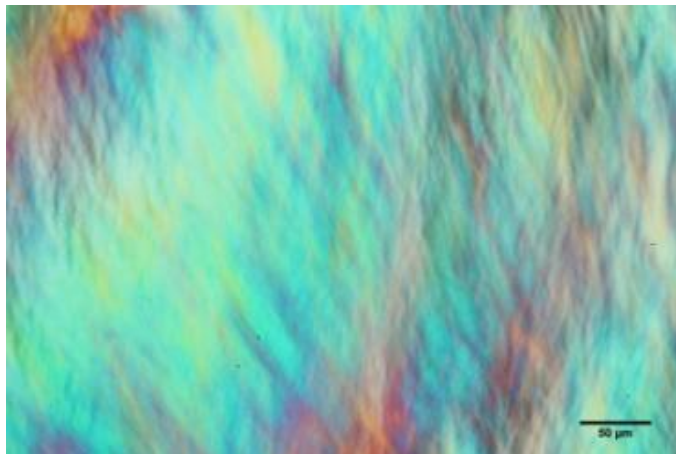
Figure 4.5 Liquid crystalline texture of a 45 wt% HPC/ m -cresol solution at room temperature
