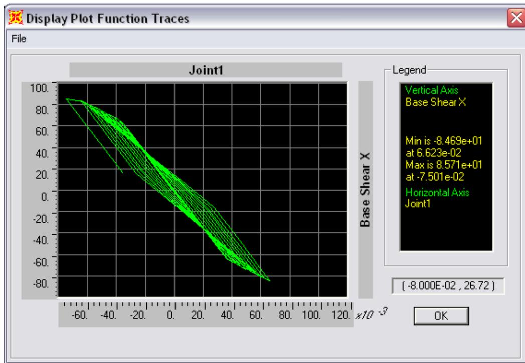
**Figure 2.13 - Displacement versus Shear Load for the Inverted-Y Steel Bracing System Loaded to 85 kips**
