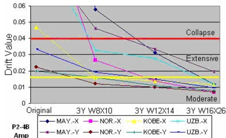
Figure 4.22 – Drift: P2-4B prototype with three inverted-Y braces – Amplified earthquakes
