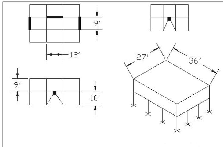
**Figure 4.9 - P1-3B prototype with three inverted-Y braces**
