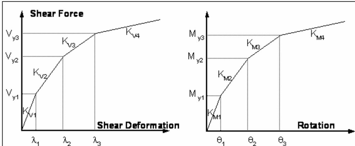
Figure 2.5 - Shear link multi-linear behavior
