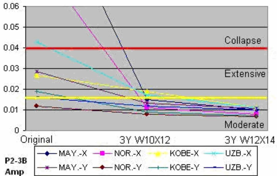
Figure 4.18 - Drift: P2-3B prototype with three inverted-Y braces – Amplified earthquakes
