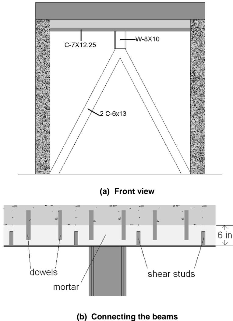
**Figure 4.2 - Proposed retrofit using inverted-Y braces**
