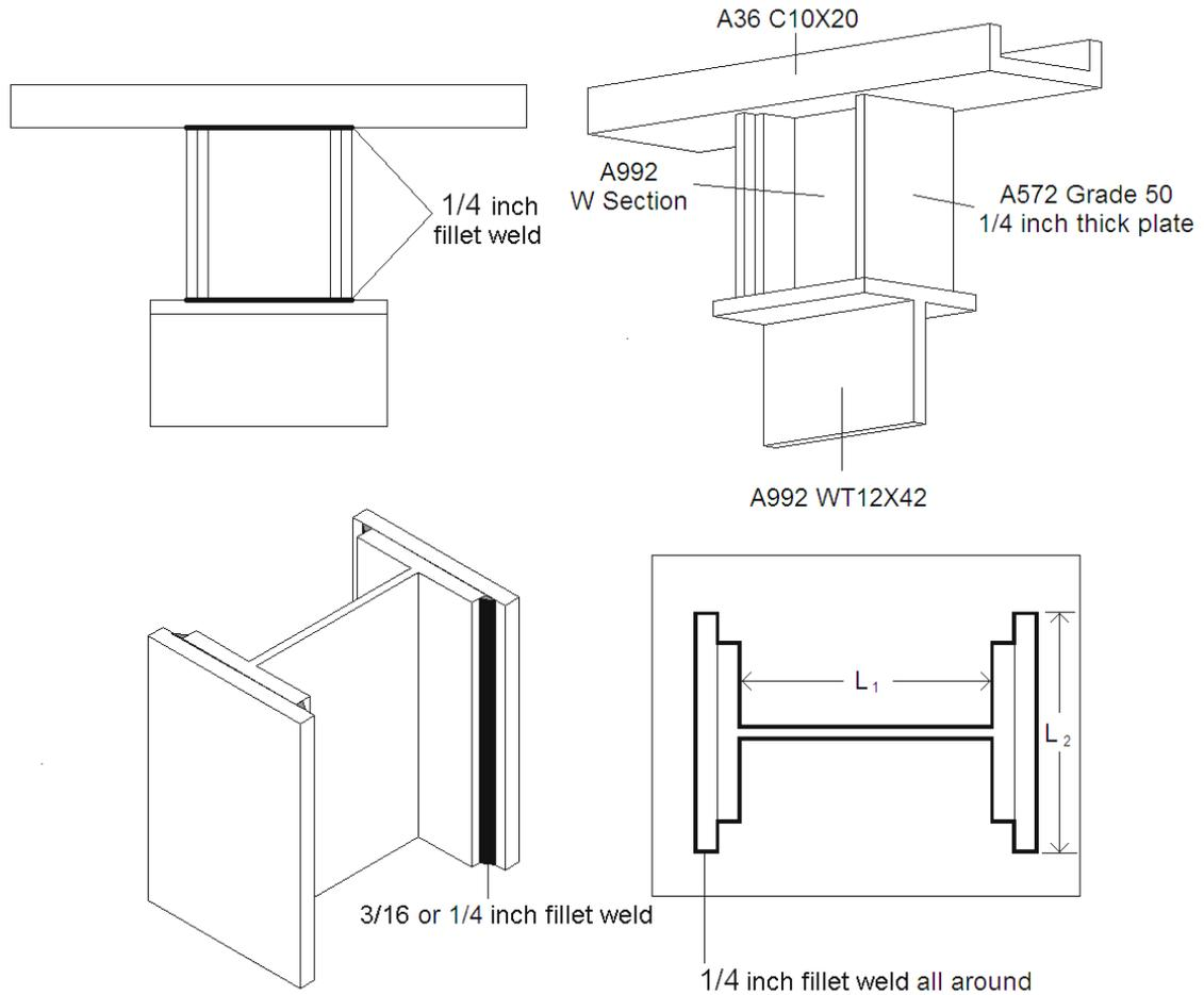
**Figure 4.4 - Shear link connection details**
