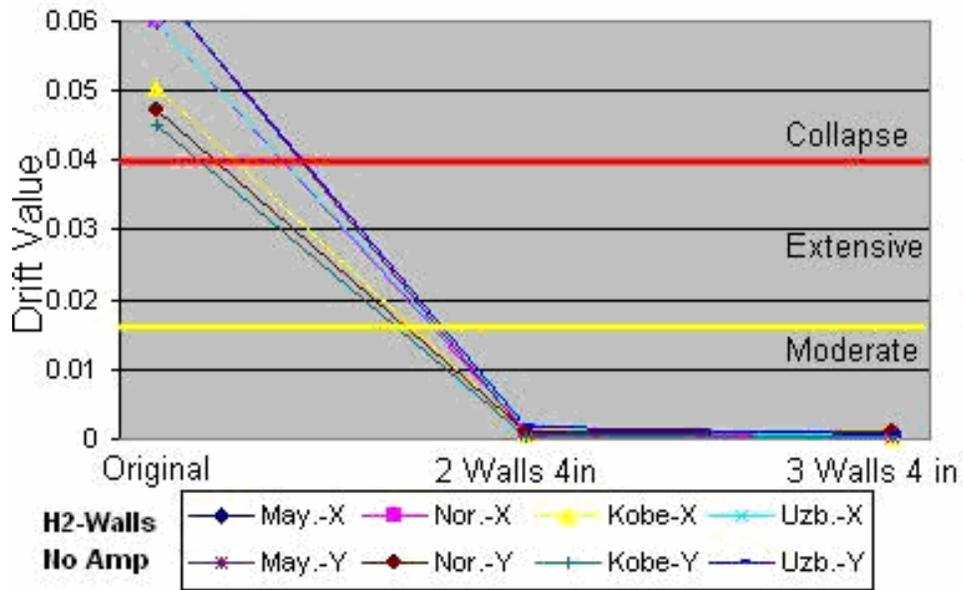
Figure 5.25 - Drift: House Model 2 retrofitted with two and three shear walls – No amplifications
