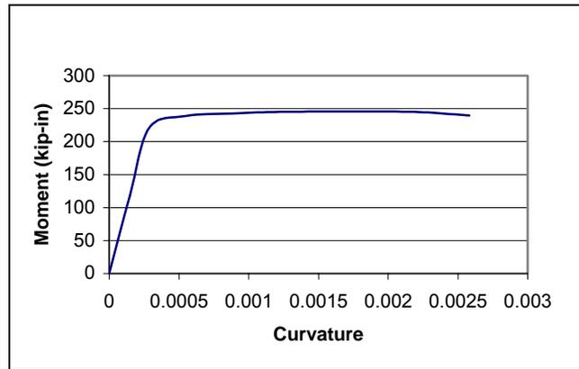
Figure 2.8 - Moment-curvature relationship for columns in Model frame
