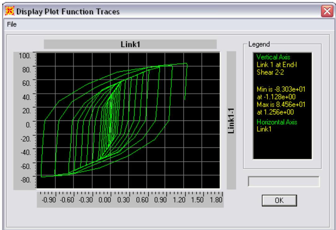
**Figure 2.15 - Lateral deformation vs. shear force in the shear link – Frame loaded to 100 kips**
