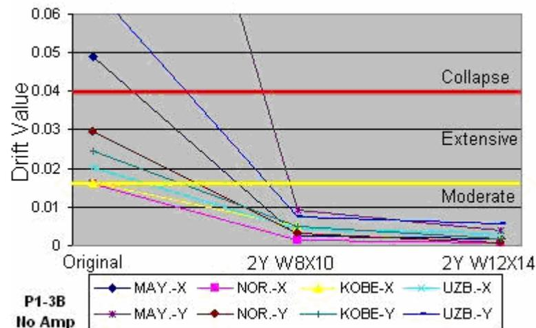
**Figure 4.6 Drift - P1-3B prototype with two inverted-Y braces – No amplification**
