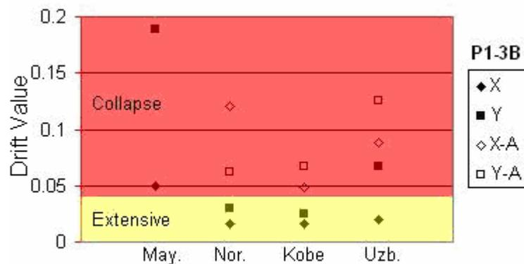
**Figure 3.15 - Drift: Prototype I Model with three bays (P1-3B)**
