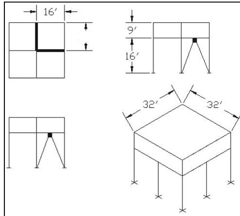
**Figure 4.23 - P3-2B prototype with two inverted-Y braces**
