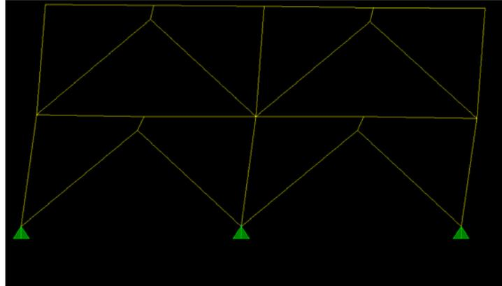
**Figure 2.4 - Deformation diagram. 2D frame with vertical shear links**
