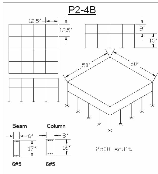
**Figure 3.4 - Prototype II Model with four bays**
