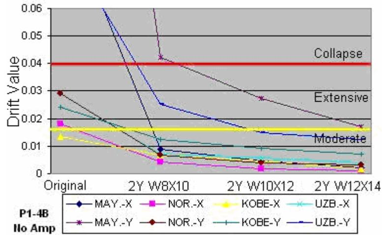
**Figure 4.12 - Drift: P1-4B prototype with two inverted-Y braces – No amplification**
