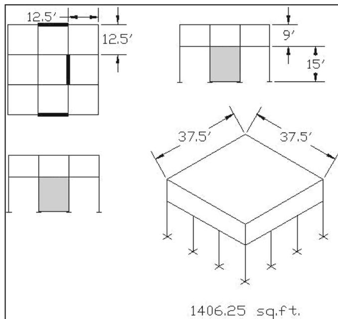
Figure 5.11 – P2-4B prototype with three shear walls
