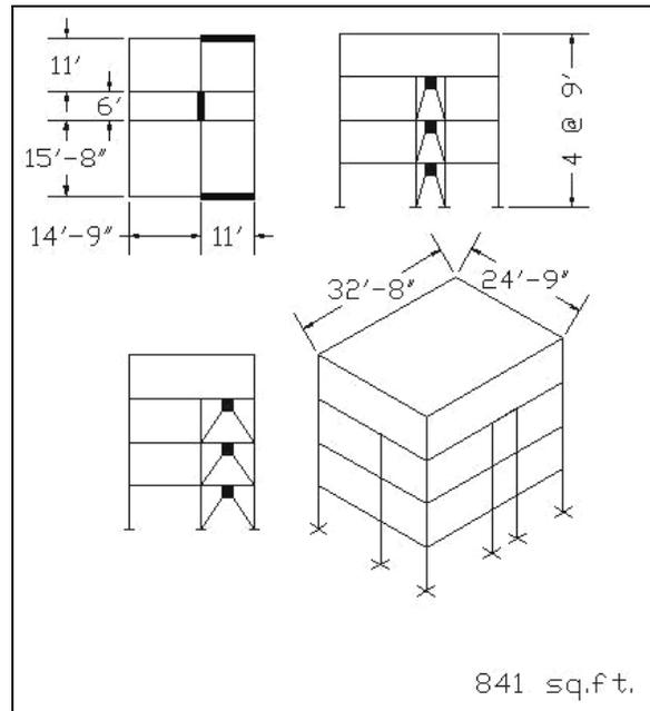
**Figure 4.31 - House Model 1 retrofitted for amplified earthquakes**
