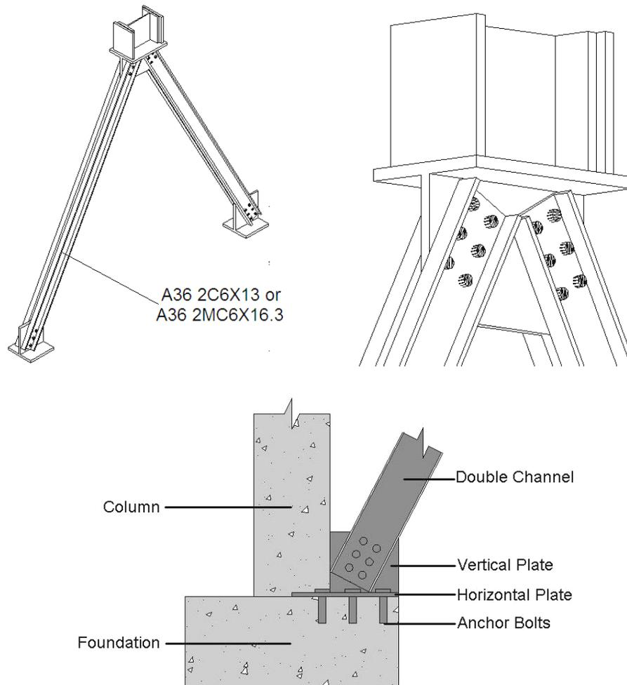
**Figure 4.3 - Connection details for diagonal braces**
