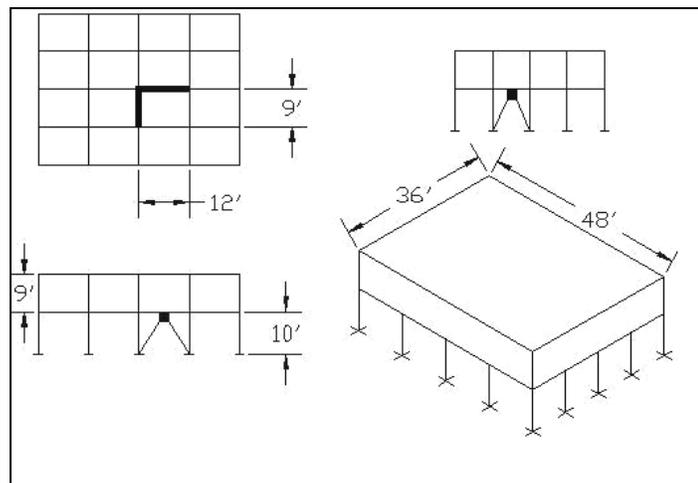
**Figure 4.11 - P1-4B prototype with two inverted-Y braces**
