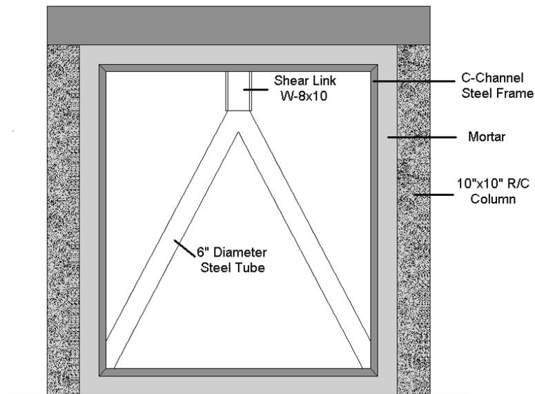
**Figure 4.1 - Steel frame retrofit with inverted-Y bracing**
