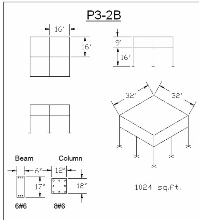
**Figure 3.5 - Prototype III Model with two bays**
