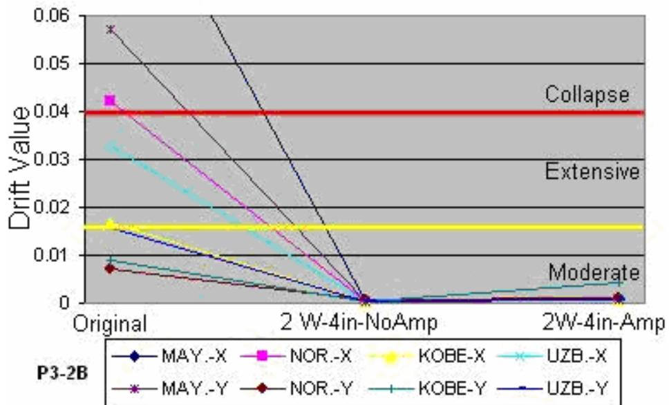
Figure 5.14 – Drift: P3-2B prototype with two shear walls
