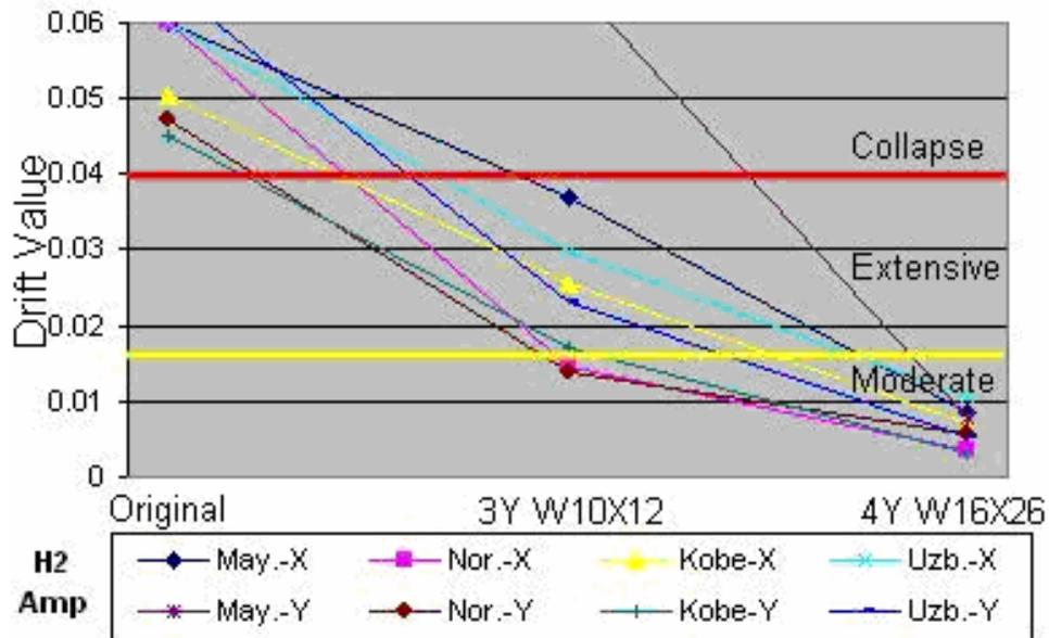
Figure 4.39 - Drift: House Model 2 - Amplified earthquakes
