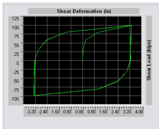
Figure 2.7 - Shear link hysteretic diagram
