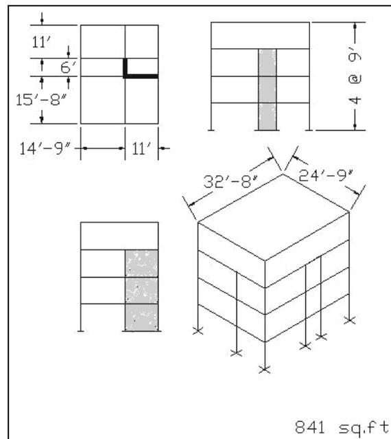
**Figure 5.19 – House Model 1 retrofitted with two shear walls**
