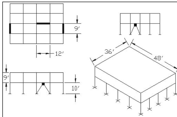
**Figure 4.13 - P1-4B prototype with three inverted-Y braces**
