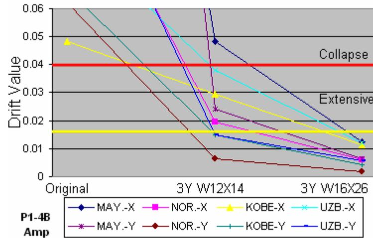
**Figure 4.14 - Drift: P1-4B Prototype with Three Inverted-Y braces – Amplified earthquake**
