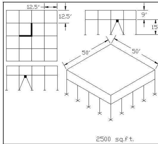
Figure 4.19 - P2-4B prototype with two inverted-Y braces
