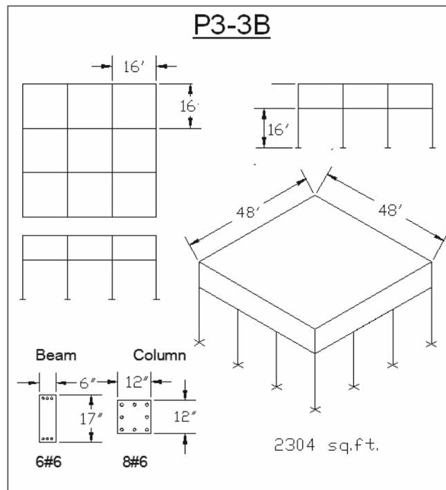
**Figure 3.6 - Prototype III Model with three bays**
