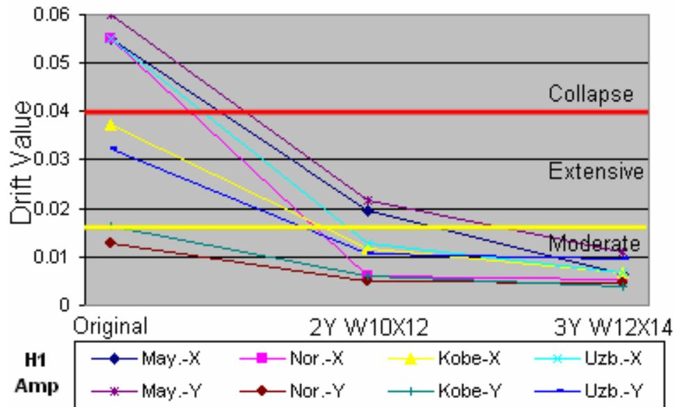
**Figure 4.37 - Drift: House Model 1 - Amplified earthquakes**
