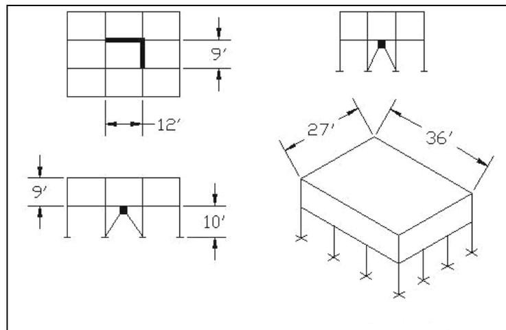
**Figure 4.5 - P1-3B prototype with two inverted-Y braces**
