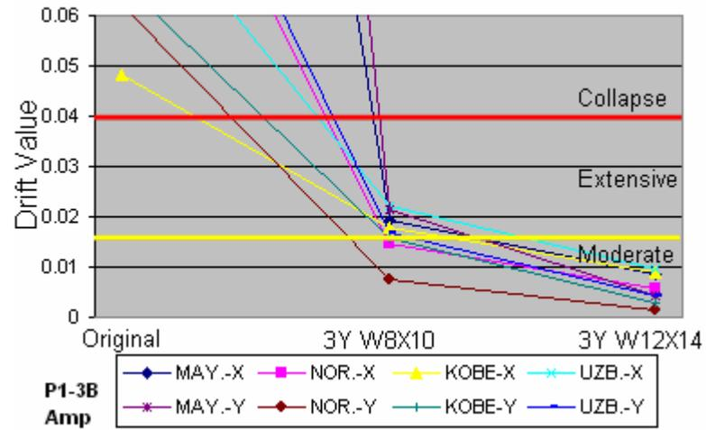
**Figure 4.10 - Drift: P1-3B prototype with three inverted-Y braces – Amplified earthquakes**
