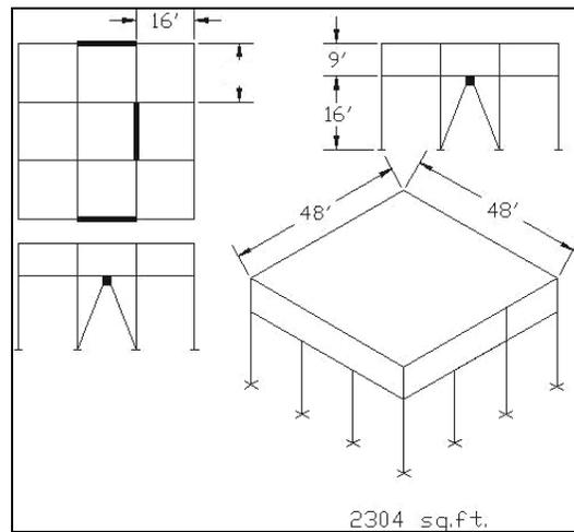
Figure 4.26 - P3-3B prototype with three inverted-Y braces
