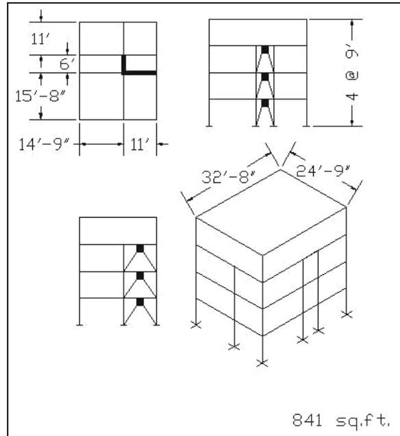
**Figure 4.30 - House Model 1 retrofitted for earthquakes without amplification**
