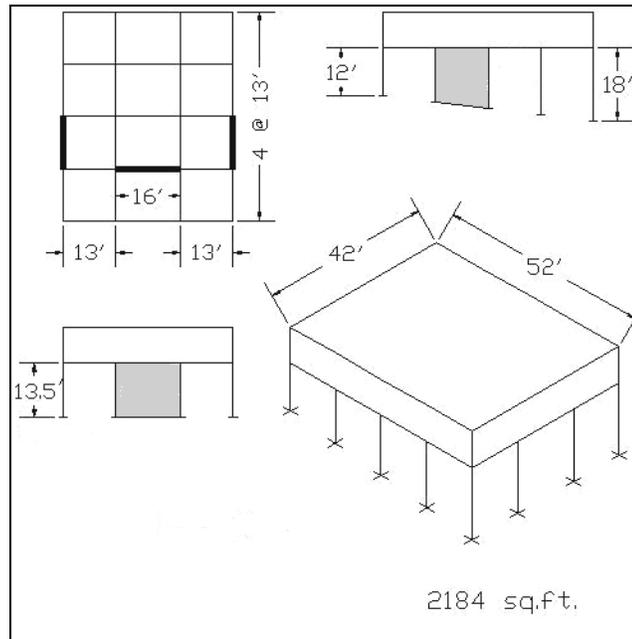
Figure 5.24 - House Model 2 retrofitted with three shear walls
