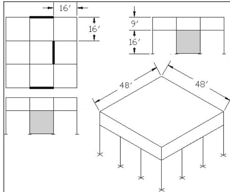
Figure 5.17 - P3-3B prototype with three shear walls
