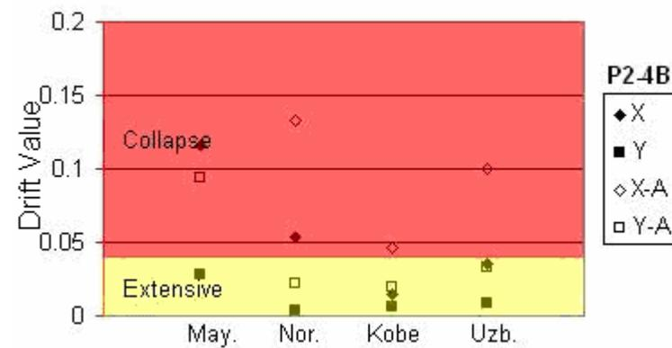
Figure 3.18 - Drift: Prototype II Model with four bays (P2-4B)
