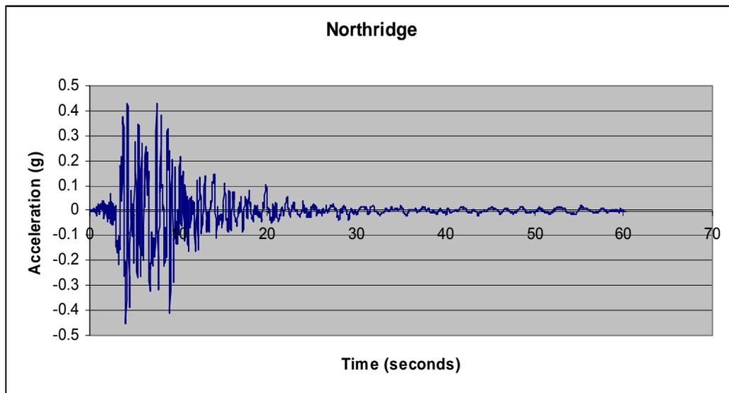
**Figure 3.11 - Northridge Earthquake Accelerogram**
