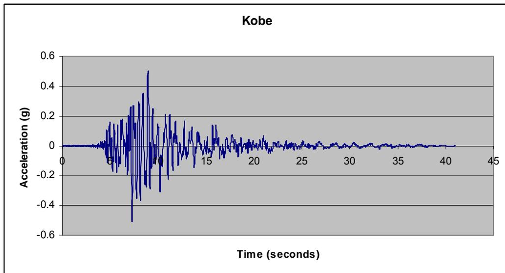
**Figure 3.12 – Kobe Earthquake Accelerogram**
