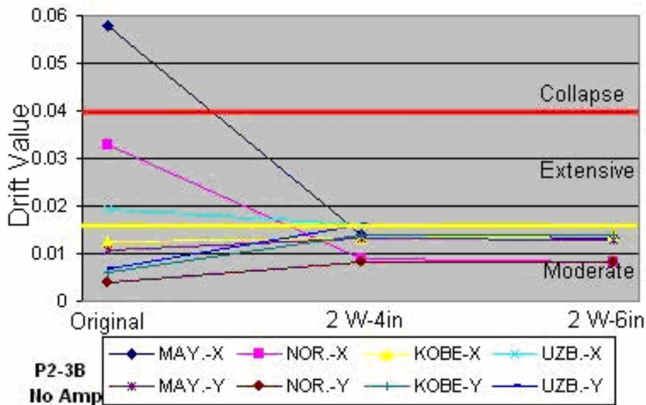
Figure 5.9 – Drift: P2-3B prototype with two Shear Walls – No amplifications
