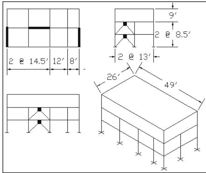
Figure 4.35 - House Model 3 retrofitted for amplified earthquakes
