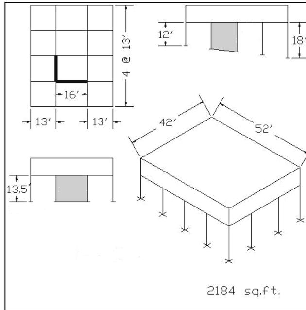
Figure 5.20 - House Model 2 retrofitted with two shear walls
