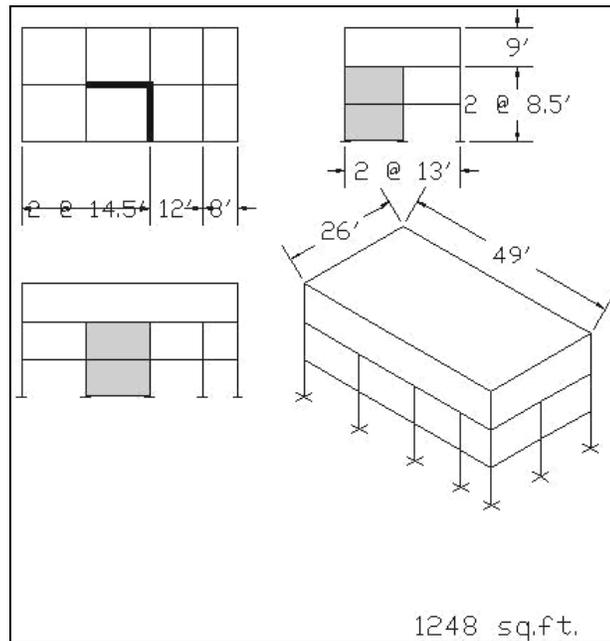
Figure 5.21 - House Model 3 retrofitted with two shear walls
