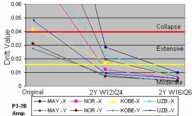
**Figure 4.25 - Drift: P3-2B prototype with two inverted-Y braces – Amplified earthquakes**
