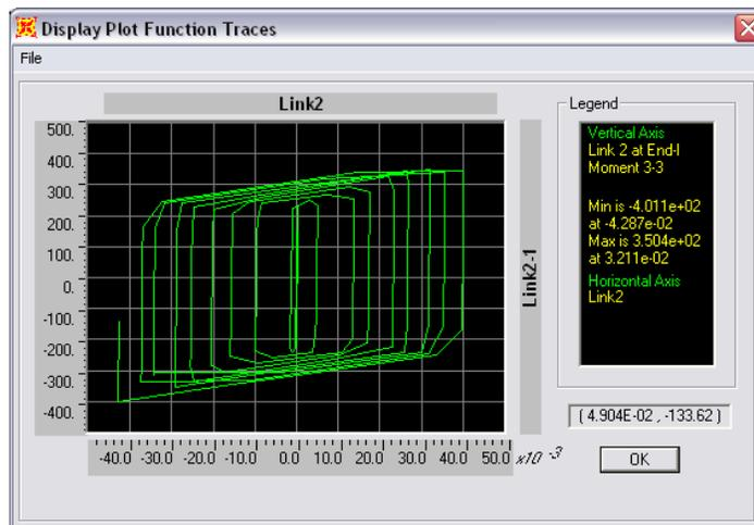
Figure 2.9 - Moment-curvature link Model without degradation
