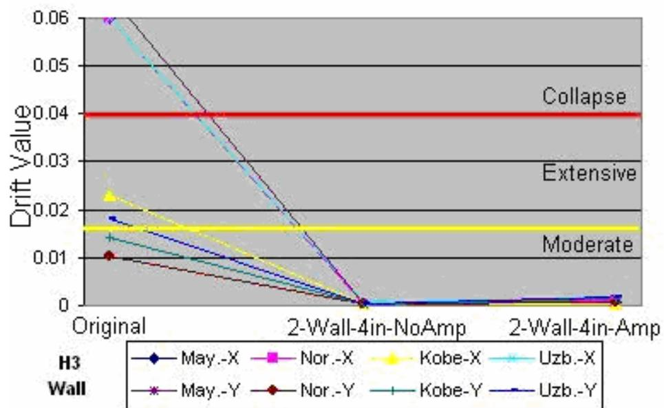
Figure 5.23 - Drift: House Model 3 retrofitted with two shear walls
