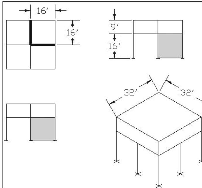
Figure 5.13 – P3-2B prototype with two shear walls
