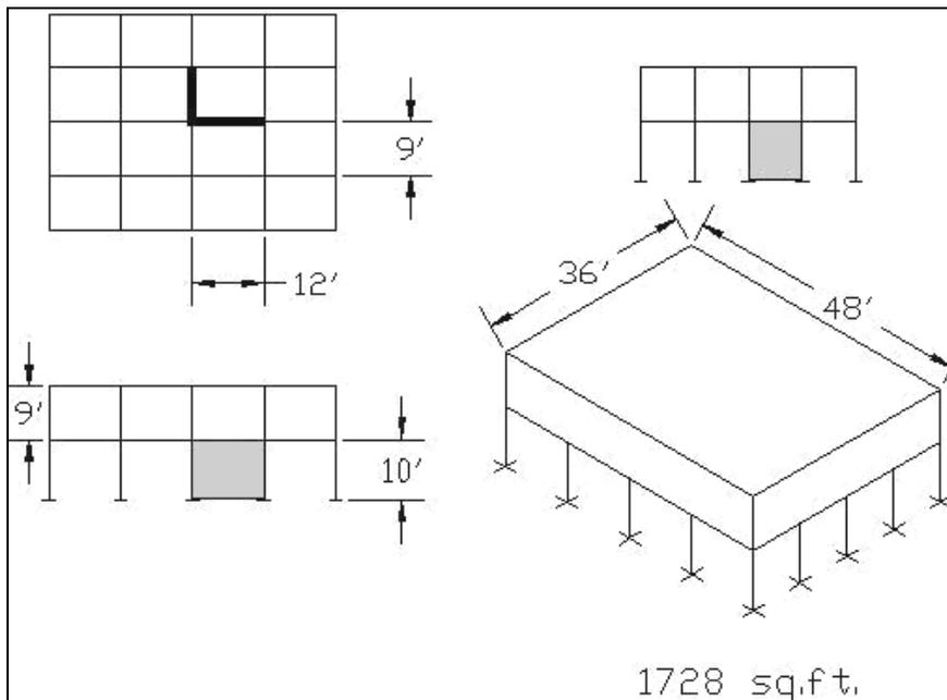
Figure 5.5 - P1-4B prototype with two shear walls
