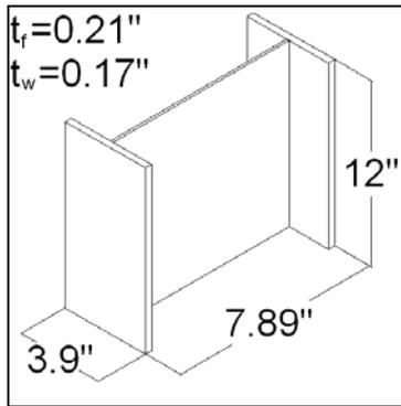
Figure 2.6 - W8x10 steel section utilized as a shear link
