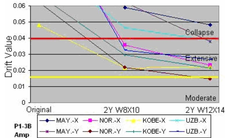
**Figure 4.7 - Drift: P1-3B prototype with two inverted-Y braces –Amplified earthquakes**
