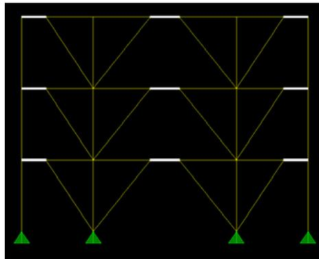
**Figure 2.2 - Two dimensional frame with horizontal shear links**
