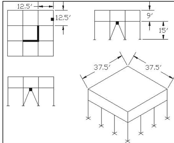
Figure 4.15 - P2-3B Prototype with two inverted-Y braces
