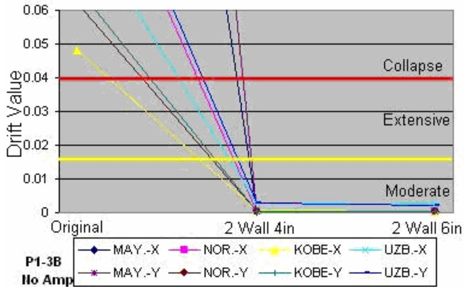
Figure 5.2 - Drift- P1-3B prototype with two shear walls - No Amplification
