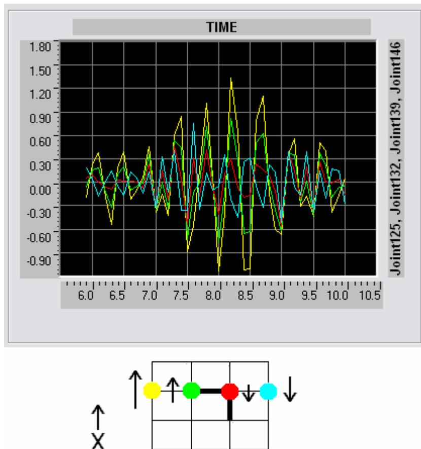
**Figure 4.8 – Displacements: P1-3B prototype with two inverted-Y braces**
