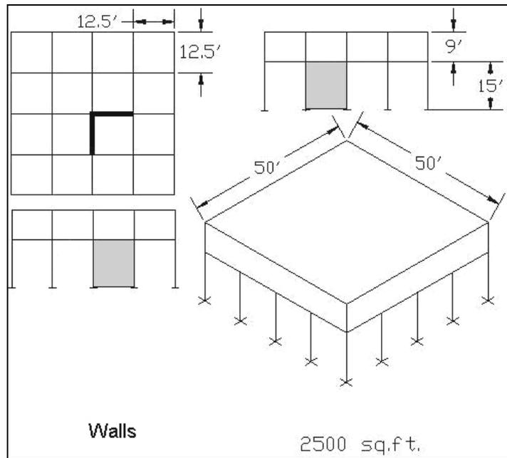
Figure 5.8 – P2-4B prototype with two shear walls
