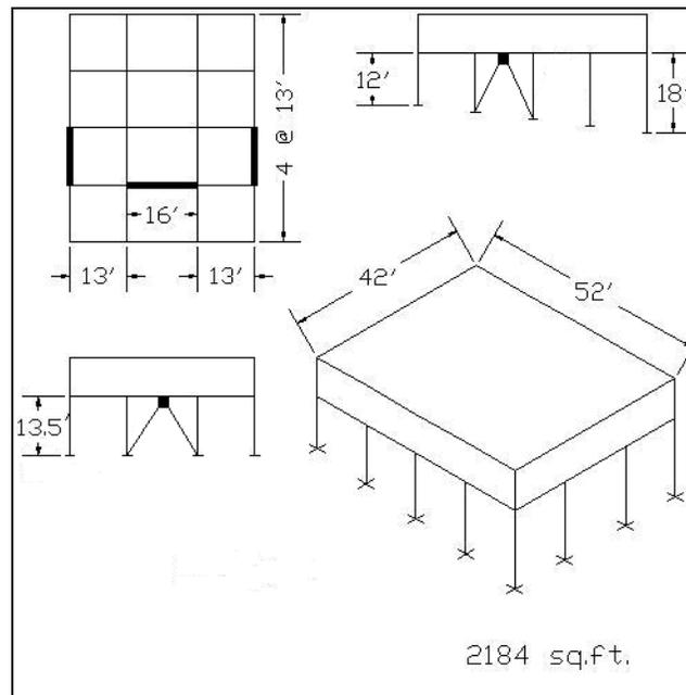
**Figure 4.32 - House Model 2 retrofitted for earthquakes without amplification**
