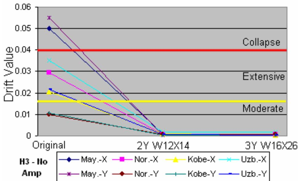
Figure 4.40 - Drift: House Model 3 – No amplifications
