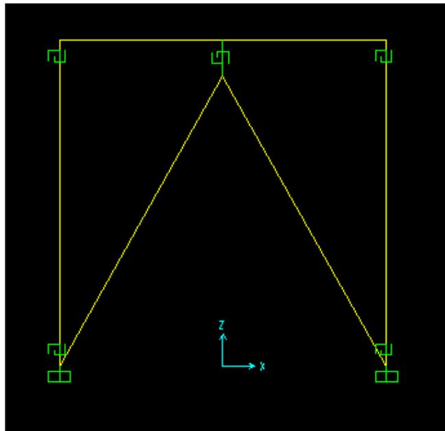
Figure 2.12 – SAP2000 Model for inverted-Y bracing system
