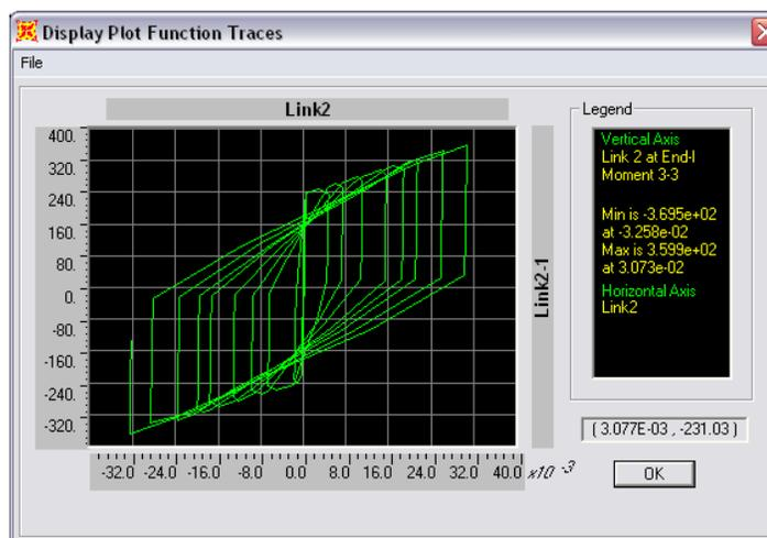
Figure 2.10 - Moment-curvature link Model with degradation
