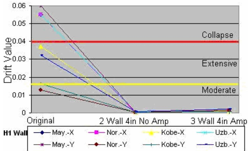
Figure 5.22 – Drift: House Model 1 retrofitted with two shear walls
