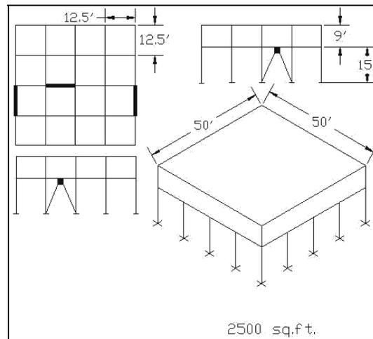
Figure 4.21 - P2-4B prototype with three inverted-Y braces
