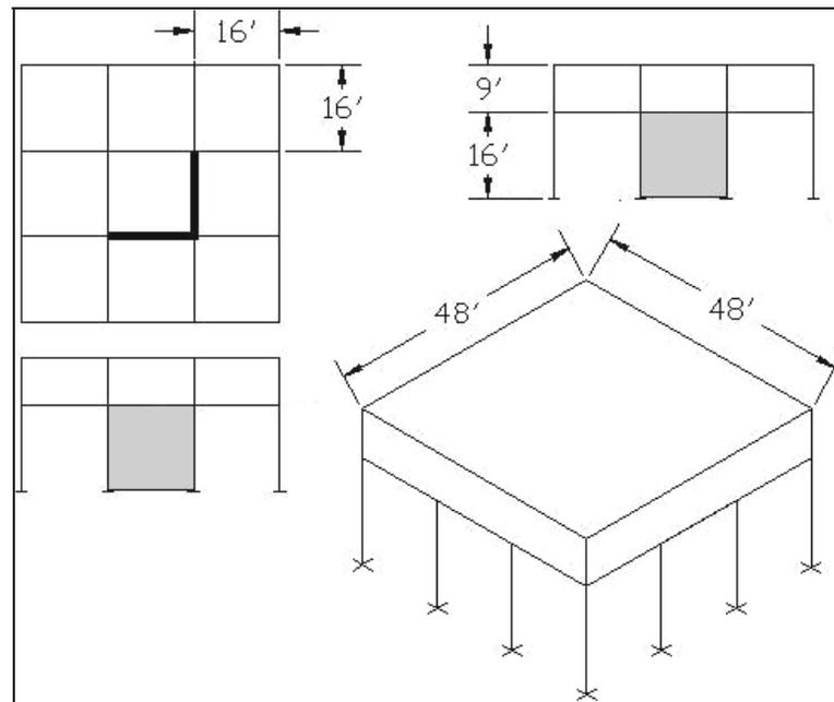
Figure 5.15 - P3-3B prototype with two shear walls
