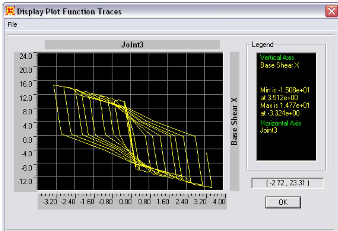
**Figure 2.11 - Base shear force vs. lateral displacements – R/C Frame**
