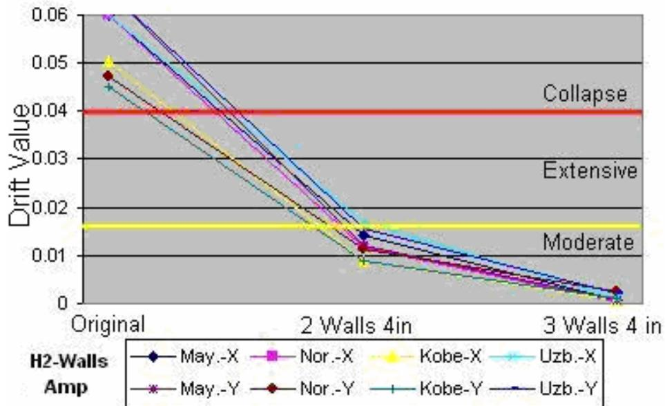
**Figure 5.26 - Drift: House Model 2 retrofitted with two and three shear walls –Amplified earthquakes**
