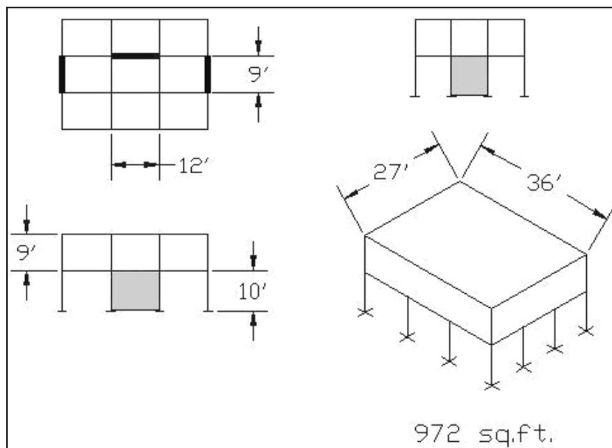
Figure 5.3 - P1-3B prototype with two shear walls
