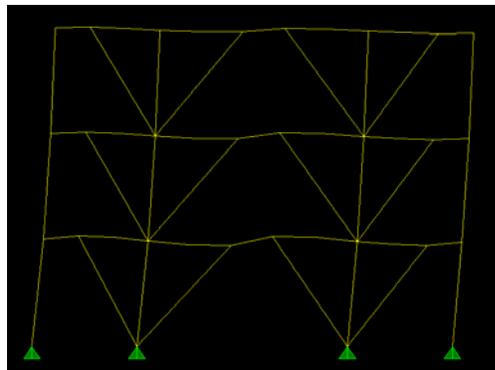
**Figure 2.3 - Deformation Diagram. 2D Frame with horizontal shear links**
