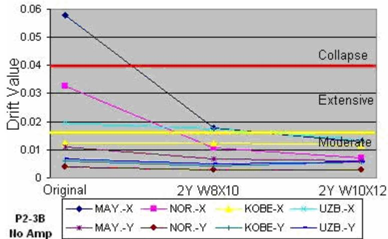
Figure 4.16 Drift: P2-3B prototype with two inverted-Y braces – No amplification
