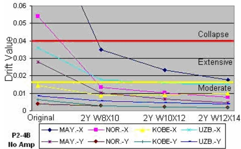
Figure 4.20 - Drift: P2-4B prototype with two inverted-Y braces – No amplification
