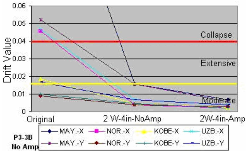
Figure 5.16 - Drift: P3-3B prototype with two shear walls – No amplification
