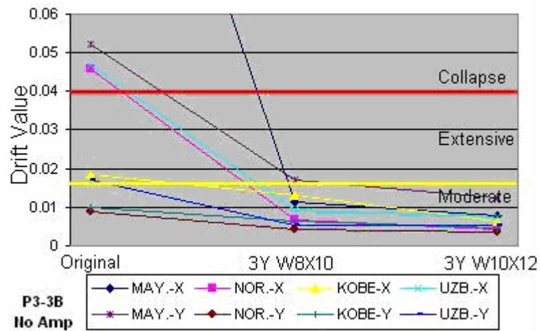
Figure 4.27 - Drift: P3-3B prototype with two inverted-Y braces – No amplification
