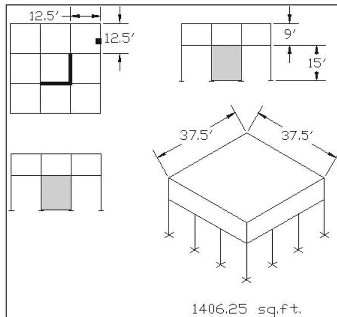
**Figure 5.7 – P2-3B prototype with two shear walls**
