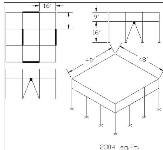
Figure 4.28 - P3-3B Prototype with Four inverted-Y braces
