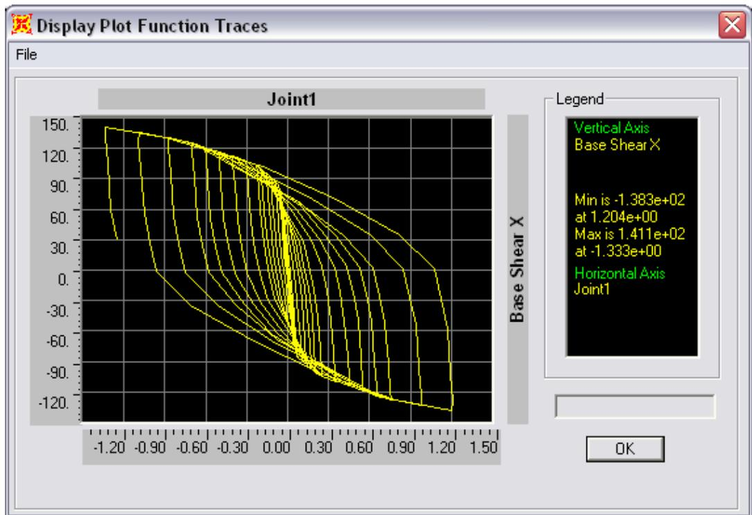
**Figure 2.14 - Displacement versus shear load for the Inverted-Y steel bracing system loaded to 145 kips**
