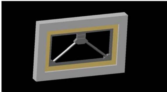
**Figure 2.1 - Concrete Frame with Inverted-Y Bracing Steel System**
