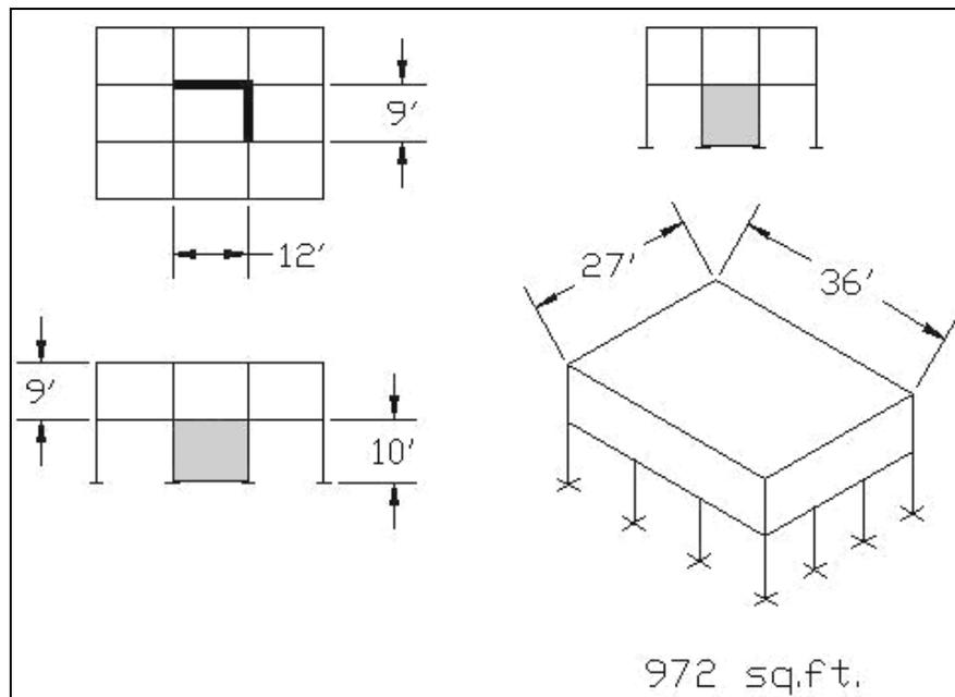
**Figure 5.1 - P1-3B prototype with two shear walls**
