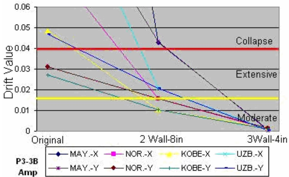
Figure 5.18 - Drift: P3-3B prototype with three shear walls – Amplified Earthquakes
