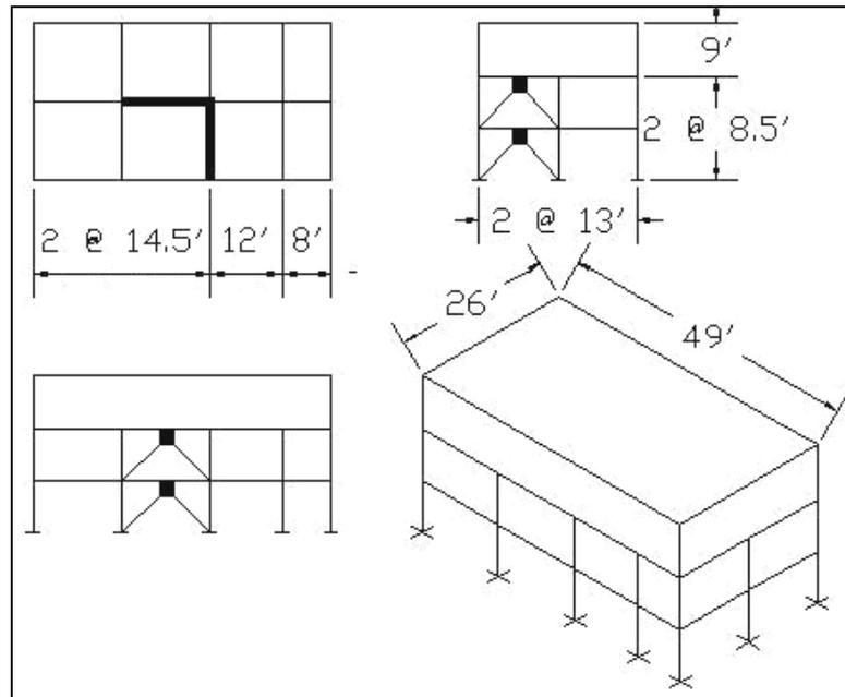
**Figure 4.34 - House Model 3 retrofitted for earthquakes without amplification**
