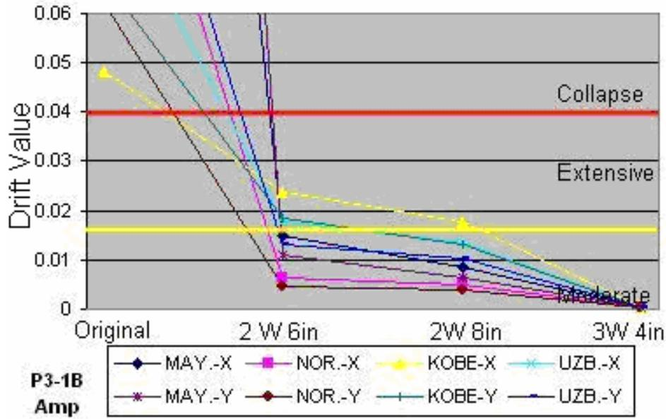
Figure 5.4 - Drift- P1-3B prototype with three shear walls – Amplified earthquakes
