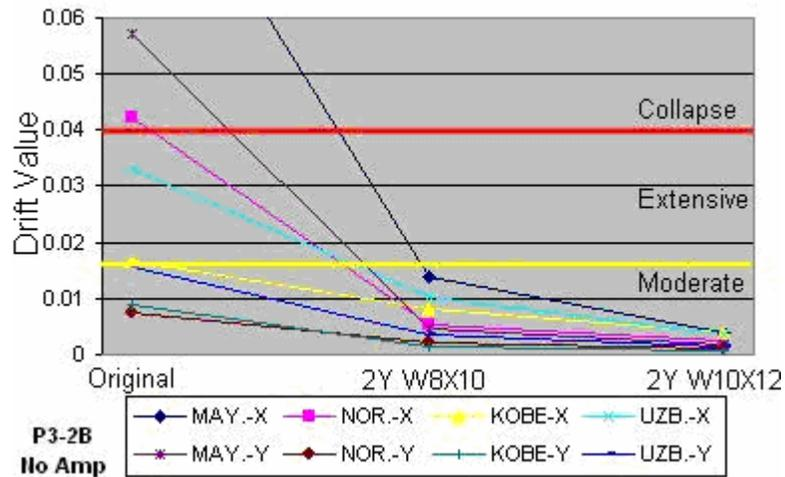
**Figure 4.24 - Drift: P3-2B prototype with two inverted-Y braces – No amplification**
