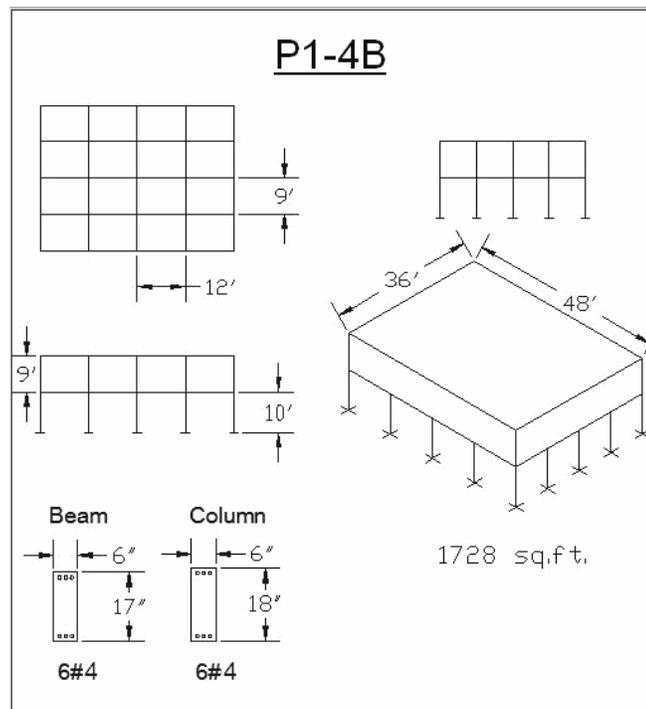
**Figure 3.2 - P1-4B: Prototype I Model with four bays**
