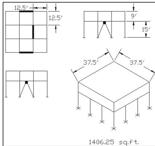
Figure 4.17 - P2-3B prototype with three inverted-Y braces
