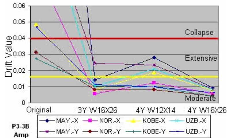
Figure 4.29 - Drift: P3-3B prototype with four inverted-Y braces – Amplified earthquakes
