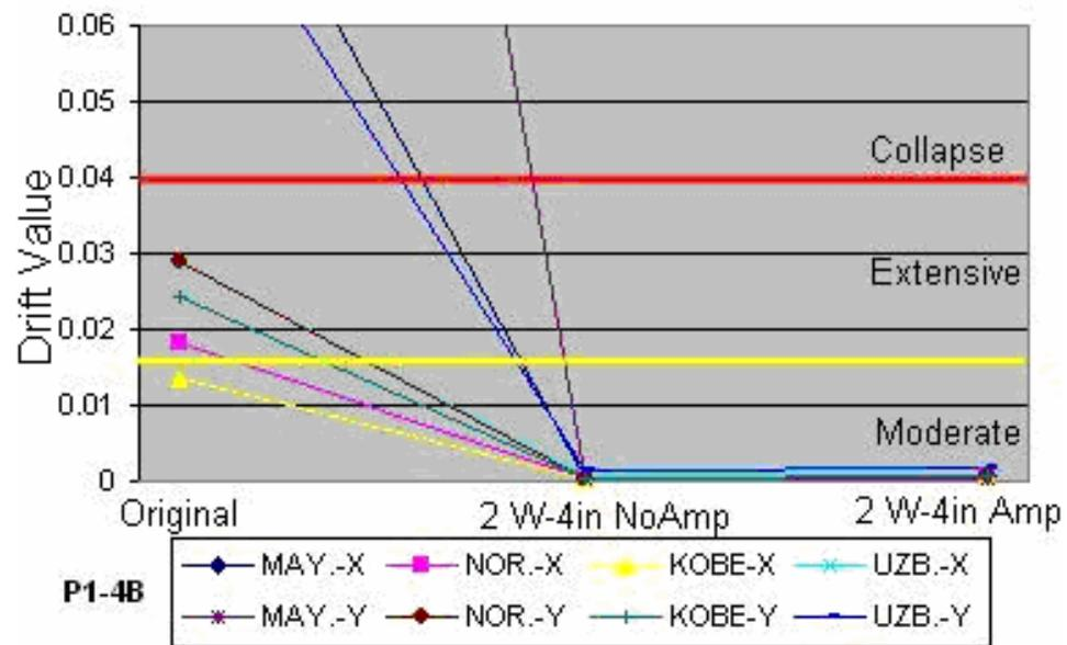
**Figure 5.6 – Drift: P1-4B prototype with two Shear Walls**
