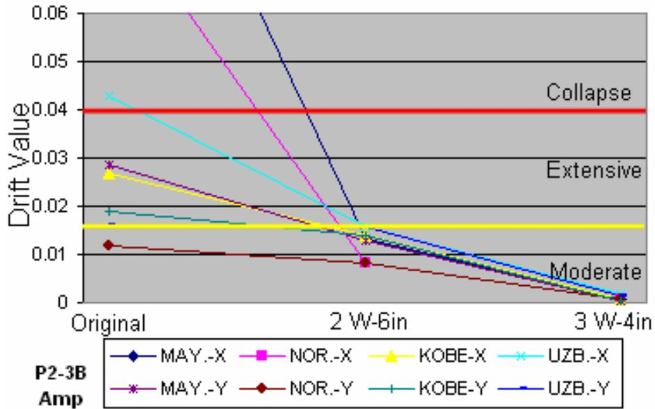
Figure 5.10 – Drift: P2-3B prototype with two Shear Walls – Amplified earthquakes
