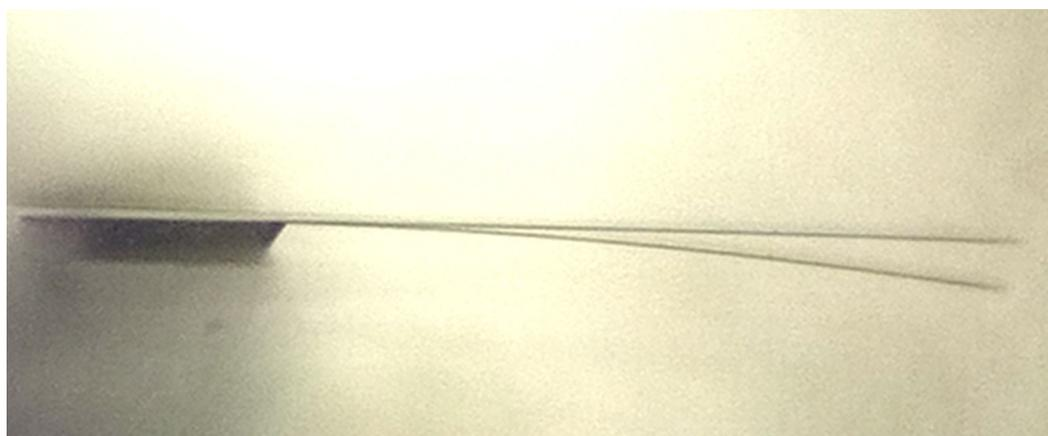
Figure 4-1. Side View of the 350  $\mu\text{m}$  Cantilever (30° C and 90° C).
