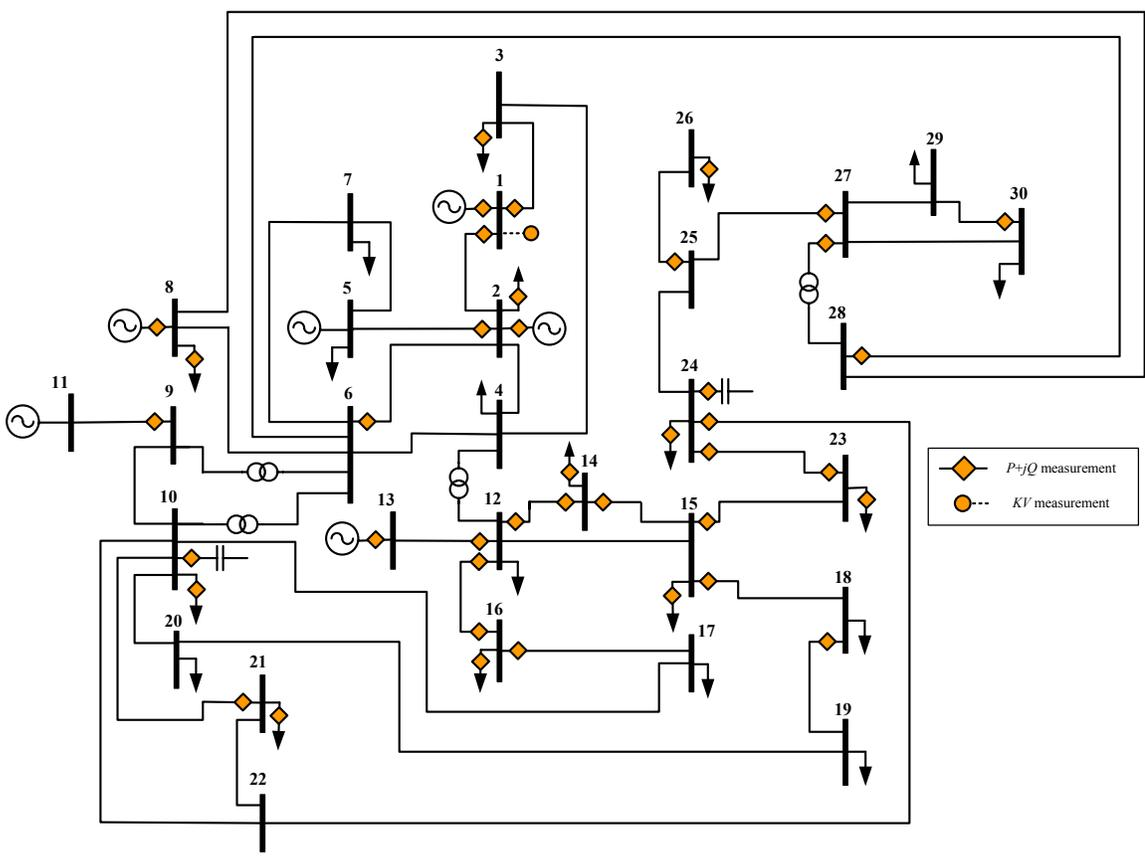
**Figure 4.4.2:** IEEE 30 Bus Test System with Measurement Locations
