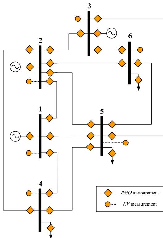
**Figure 4.4.1:** Six Bus Test System with Measurement Locations
