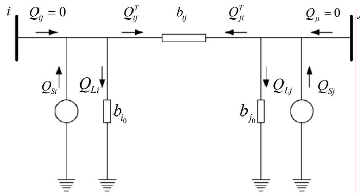
**Figure 3.2.2:** Simulated Post-Outage for Reactive Power.
