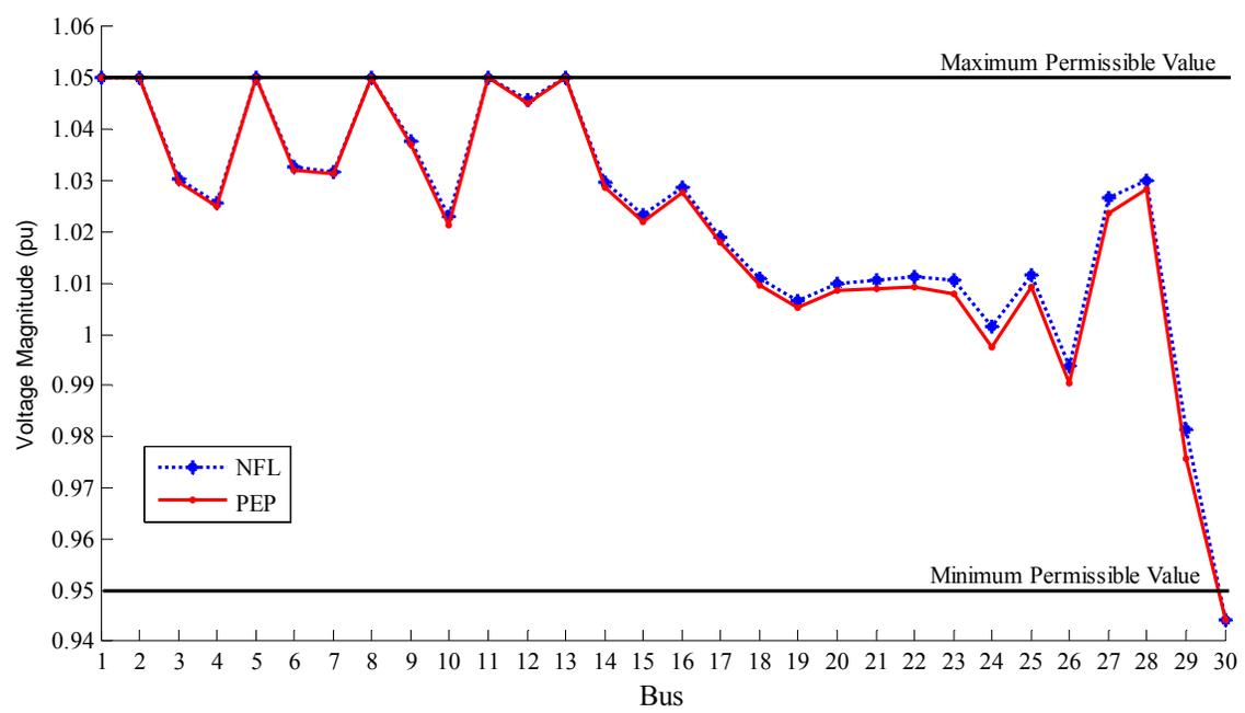
Figure 3.4.6: Post-outage Bus Voltage Magnitude Profile. Outage in Line 27-30
