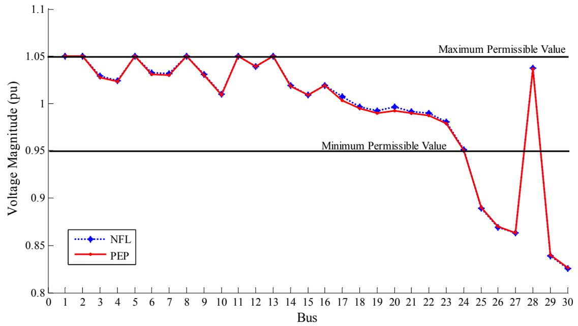
Figure 3.4.5: Post-outage Bus Voltage Magnitude Profile. Outage in Line 27-28
