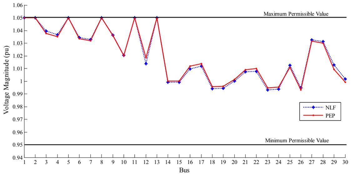
**Figure 3.4.2:** Post-outage Bus Voltage Magnitude Profile. Outage in Transf. 4-12.
