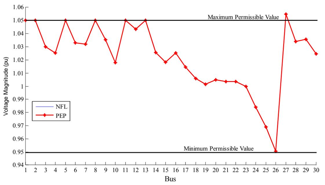
Figure 3.4.4: Post-outage Bus Voltage Magnitude Profile. Outage in Line 25-27
