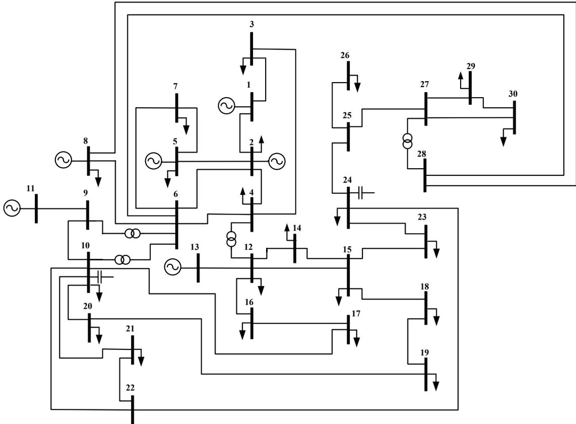
**Figure 3.4.1:** Modified IEEE 30 Bus Test System
