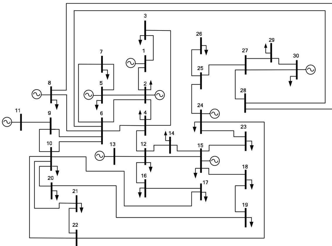
**Figure 5.3.3:** Modified IEEE 30 Bus Test System
