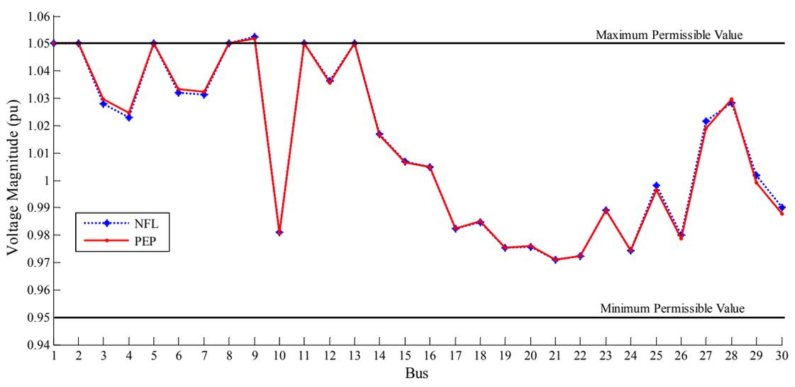
Figure 3.4.3: Post-outage Bus Voltage Magnitude Profile. Outage in Line 9-10
