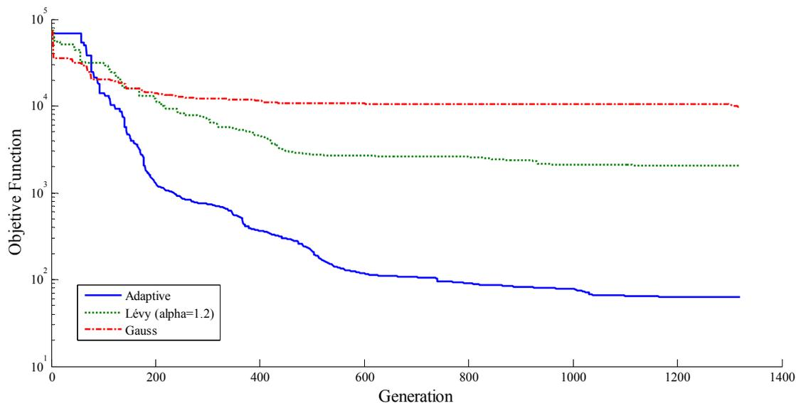
**Figure 4.4.3:** Convergence rate of EP with several mutation operators.
