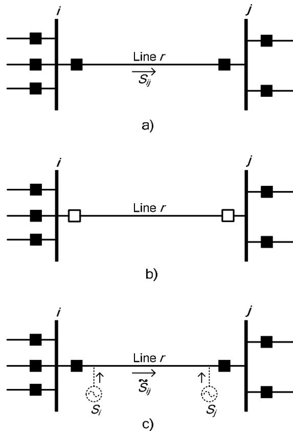
**Figure 3.2.1:** Line Outage Modeling Using Fictitious Injections. a) Pre-outage Condition. b) Post-outage Condition. c) Simulated Post-outage Condition.
