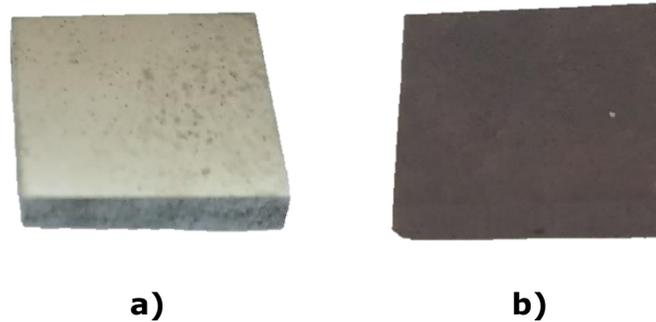
**Figure 33: Photographs of a HC-2 sample, a) before and b) after corrosion in 10 vol% NaOH for 24 hours.**
