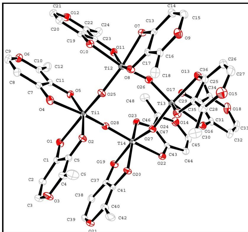
Figure 3-11: Solid state structure of  $[\text{Ti}_4(\text{maltolato})_8(\mu\text{-O})_4]$
