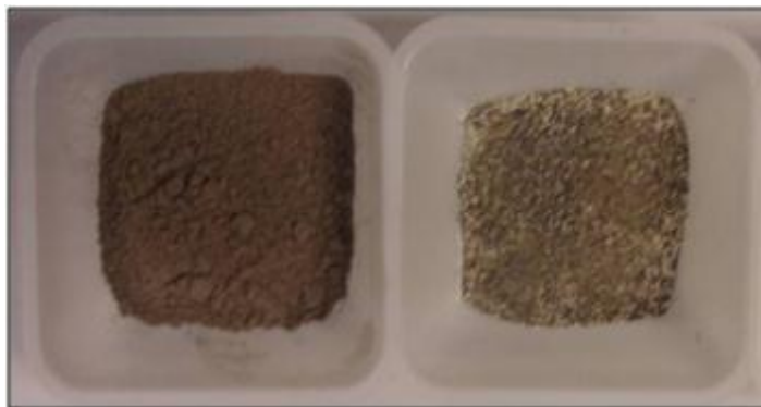
Figure 3. Fly Ash (left) and Bottom Ash (right) Acquired from AES.
