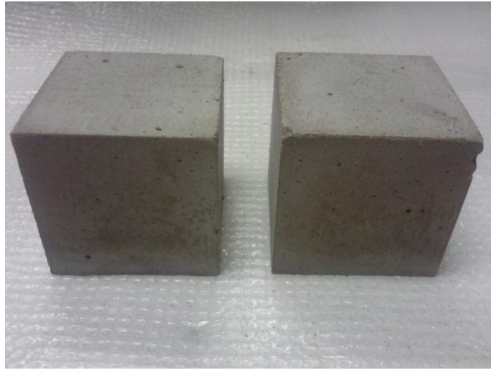
Figure 14. Compressive Test Specimens with 33% Bottom Ash.
