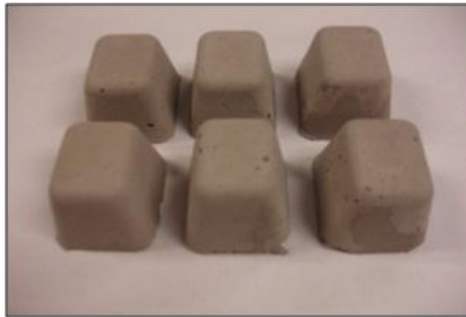
Figure 4. Shape and Appearance of the CAAM Blocks.
