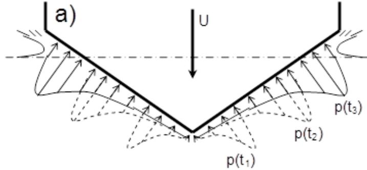
Figure 2: Wave slamming pressure distribution along V shape Wedge
