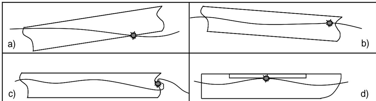
Figure 1: Basic slamming classification, a) Bottom slamming b) Bow-flare slamming c) Breaking wave impact d) Wetdeck slamming (Catamaran)
