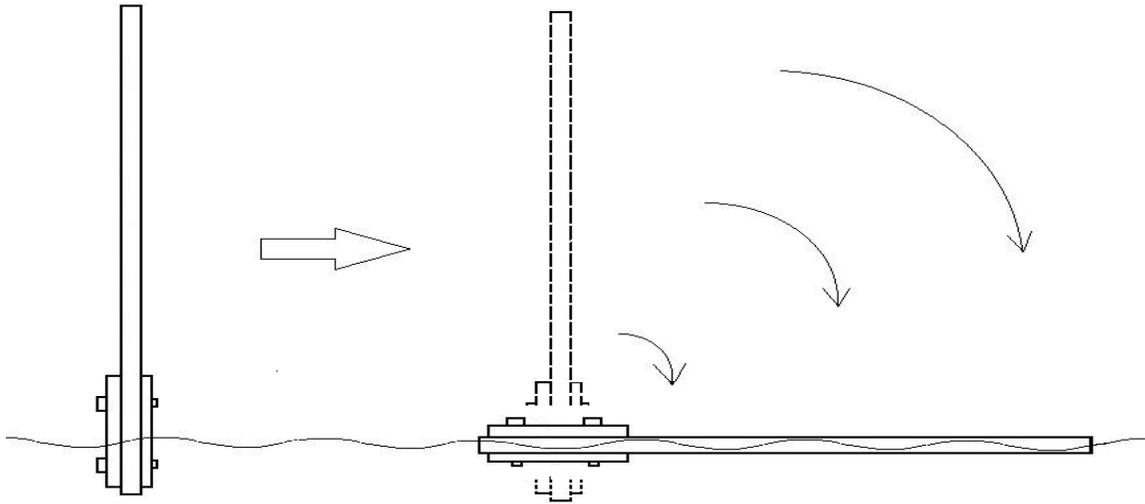
Figure 4: Repeated slamming apparatus and specimen
