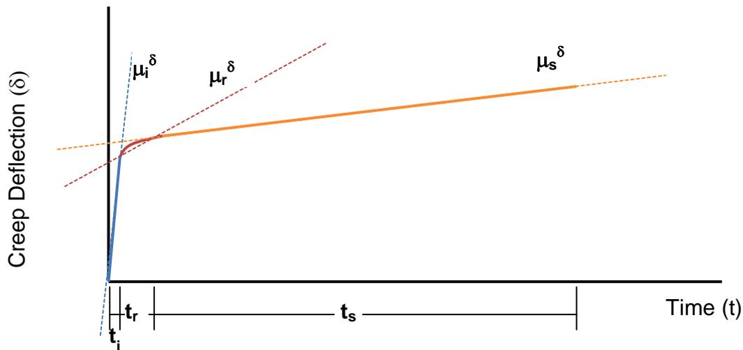
Figure 12: (a) Burger's model illustrating various stages of creep, (b)  $\delta$ -t curve and corresponding slopes.
