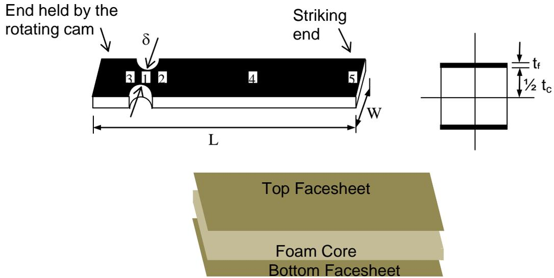
Figure 3: Specimen Configuration. [1] to [5] represent the locations of the strain gauges while pressure transducers were placed at locations [3] to [5] on model specimens
