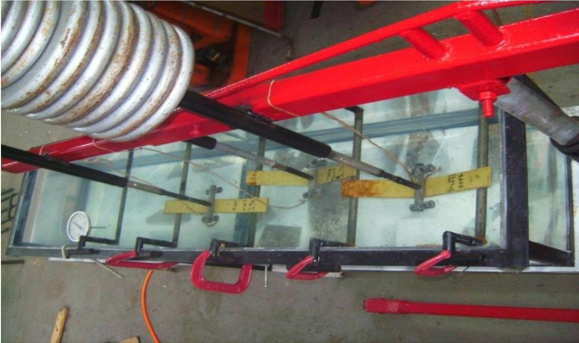
Figure 10: Creep testing apparatus
