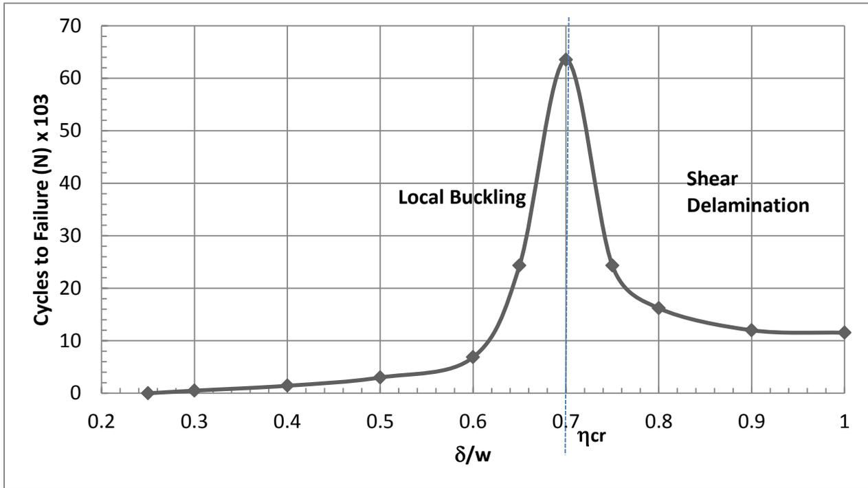
Figure 7: Average number of cycles to failure as a function of flaw size for *Type 2* specimens. Shift in mode and site of failure at the transition point  $\delta_{cr}/w$
