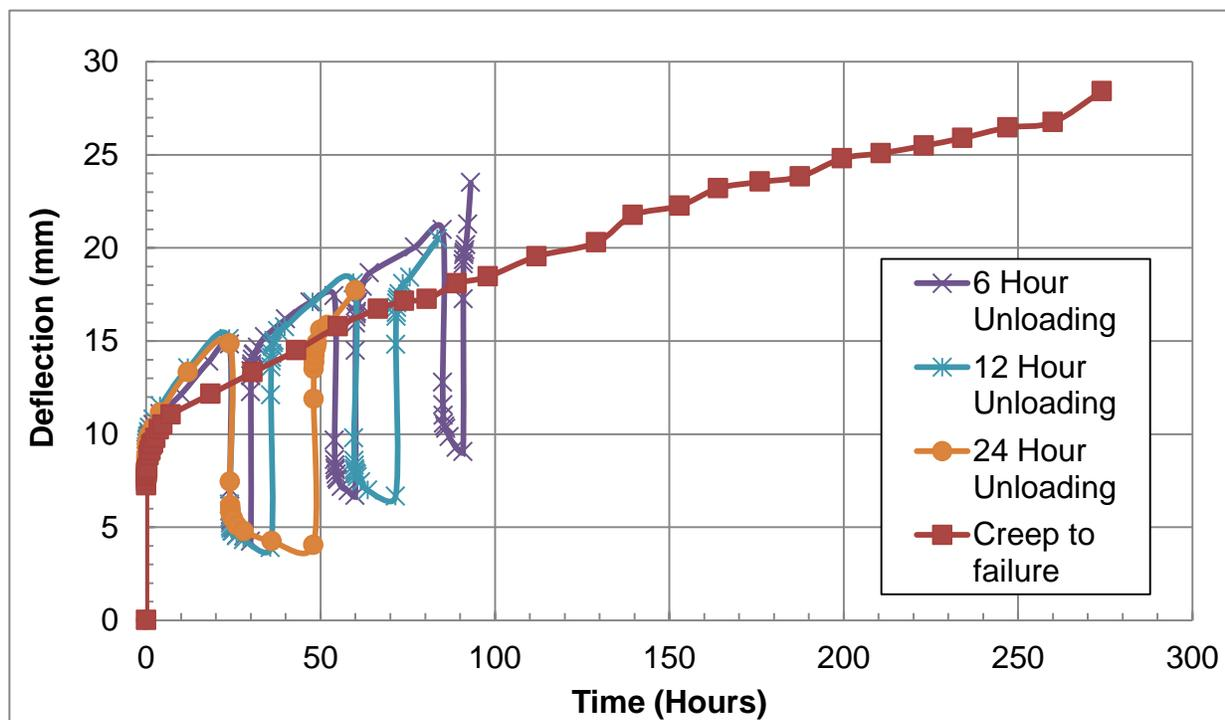
Figure 17: Comparison of typical creep to failure and cyclic creep
