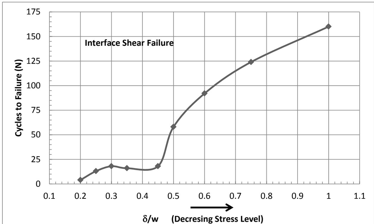
Figure 6: Average number of cycles to failure as a function of flaw size for *Type I* specimens. No shift in modes of failure
