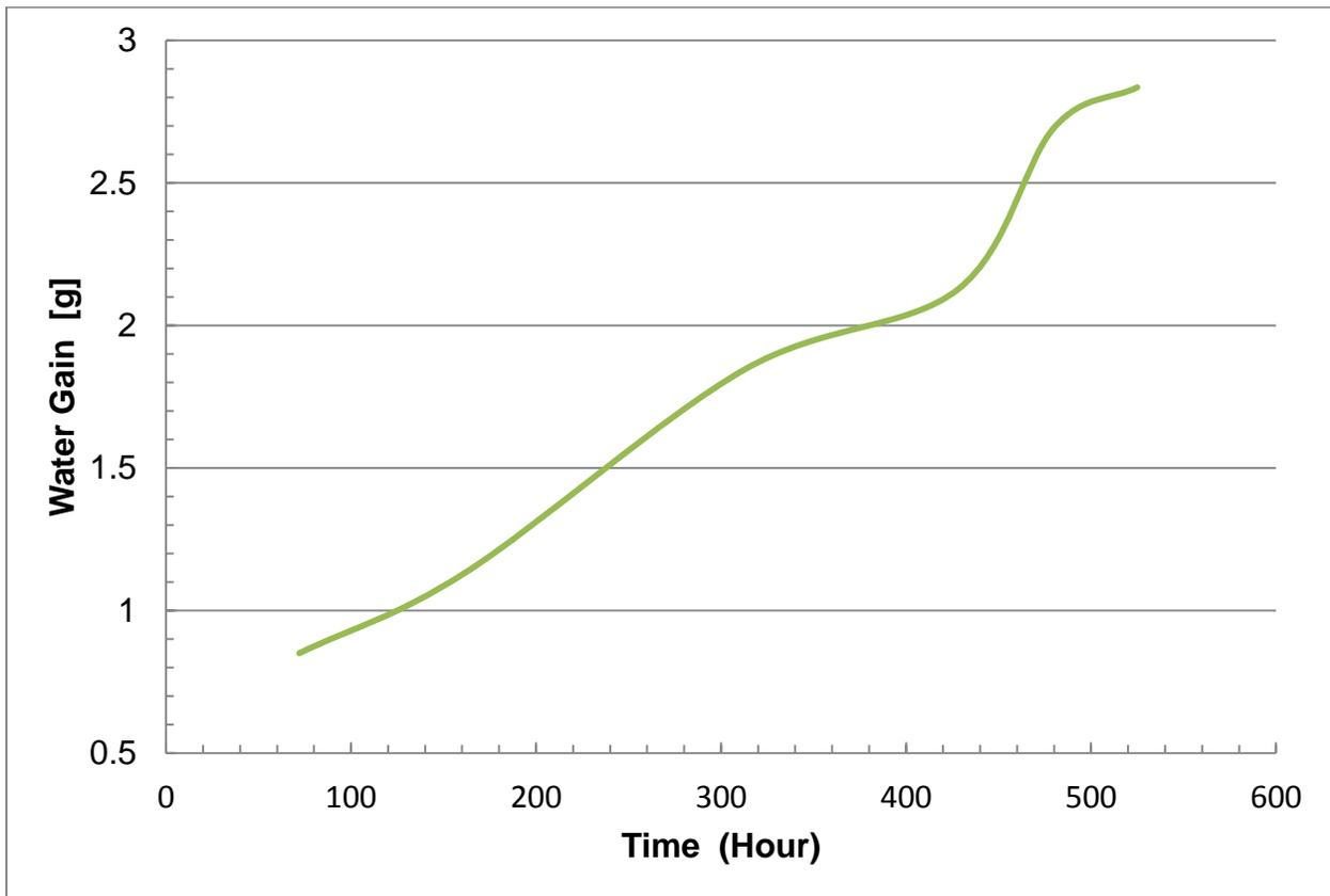
Figure 13: Typical water absorption as a function of time
