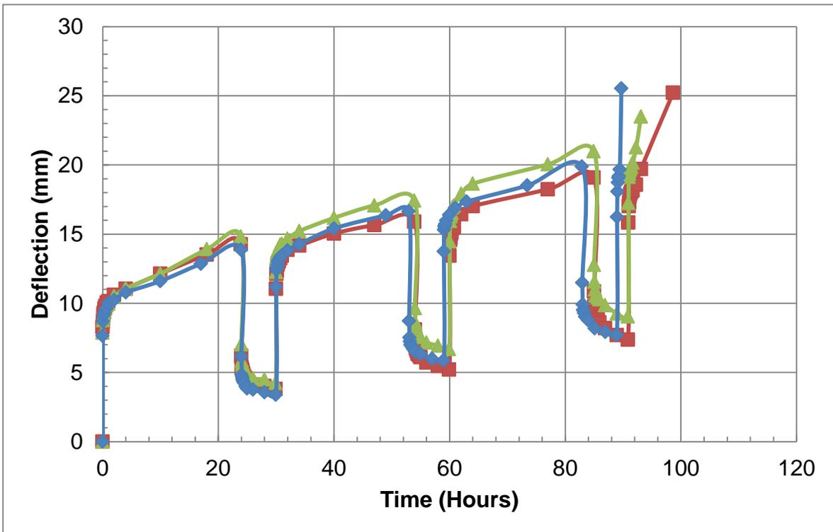
Figure 16: 24 hour loading and 6 hour unloading cyclic creep results
