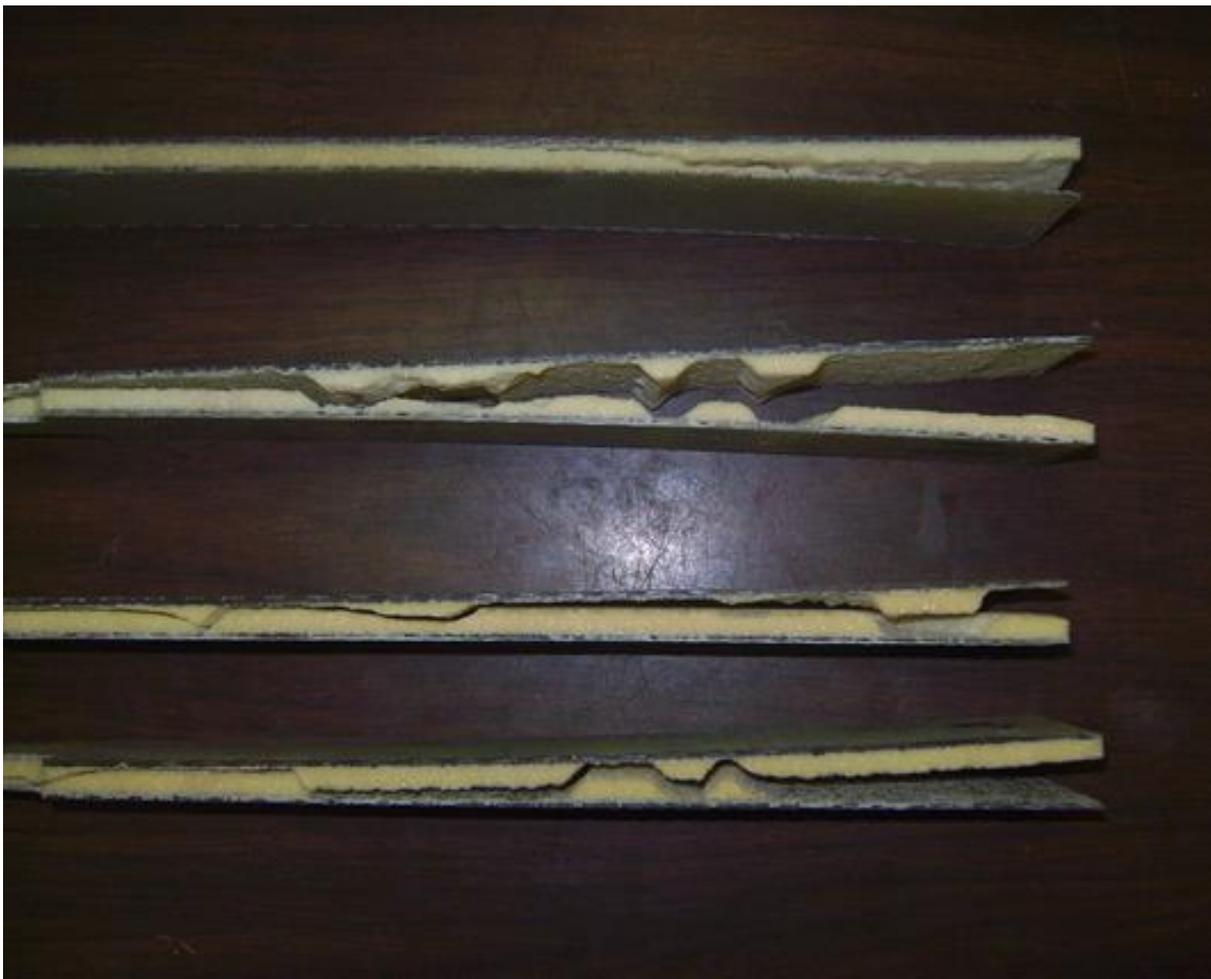
Figure 5: Typical interface and through the thickness shear failure in *Type 1* Specimens
