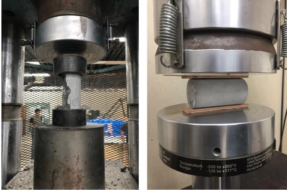
Figure 3.6: Compressive Strength Test (Left) and Tensile Strength Test (Right)
