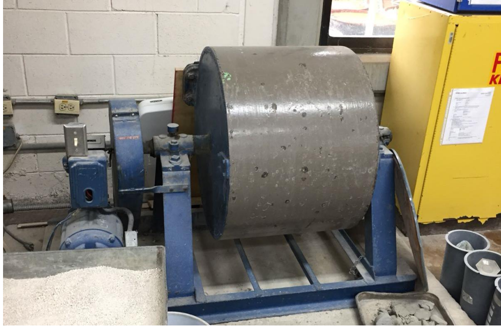
Figure 4.2: LA Abrasion Machine
