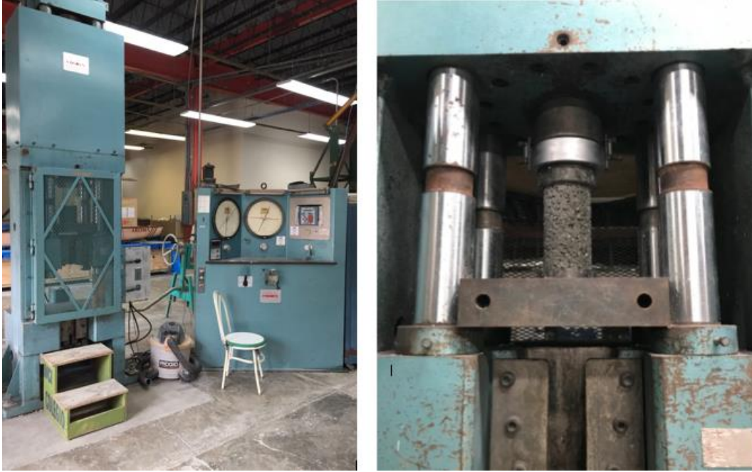
Figure 4.1: Forney universal testing machine (left), Compressive strength test on pc specimen (right)
