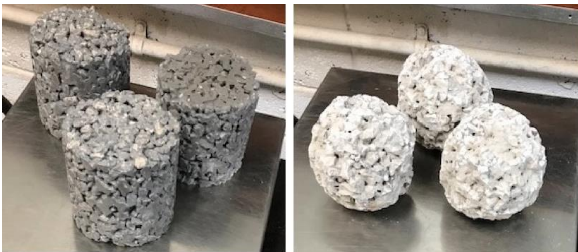
Figure 4.3: PC specimen before (left) and after (right) the LA abrasion test
