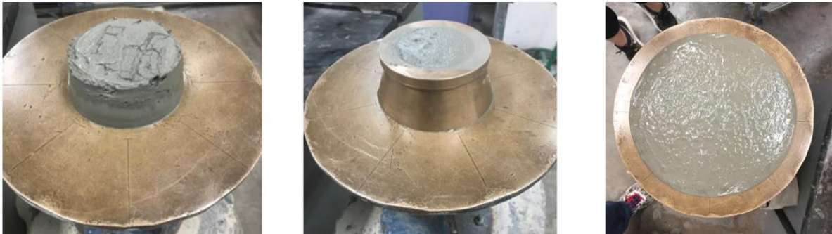
Figure 3.7: Spread percentage test
