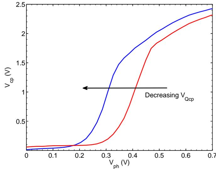
Figure 3.17 : Output voltage of the start-up circuit for two different programmed voltages.
