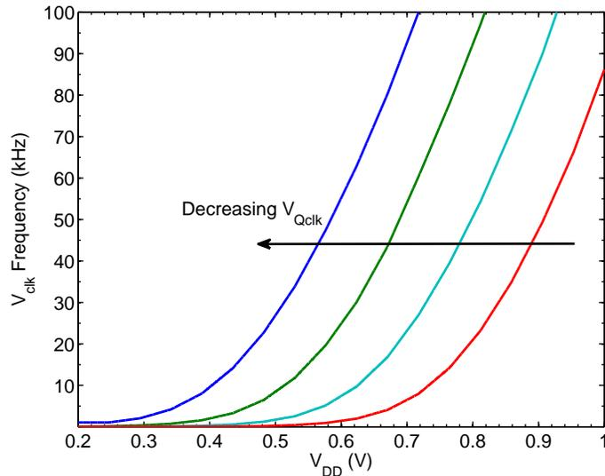
Figure 3.14 : Simulated results demonstrating the frequency of the oscillator with respect to  $V_{DD}$  for different  $V_{Qclk}$  values.
