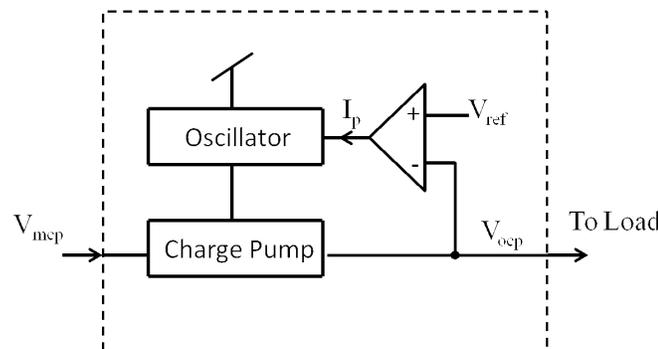
Figure 3.6 : Block diagram of the DC-DC conversion stage.
