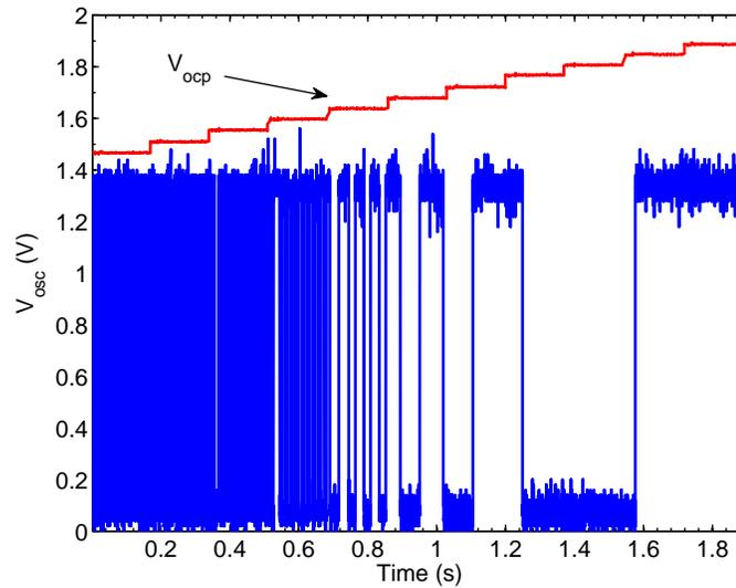
Figure 3.8 : Frequency variation change with a sweep of  $V_{ocp}$  in the feedback circuit.
