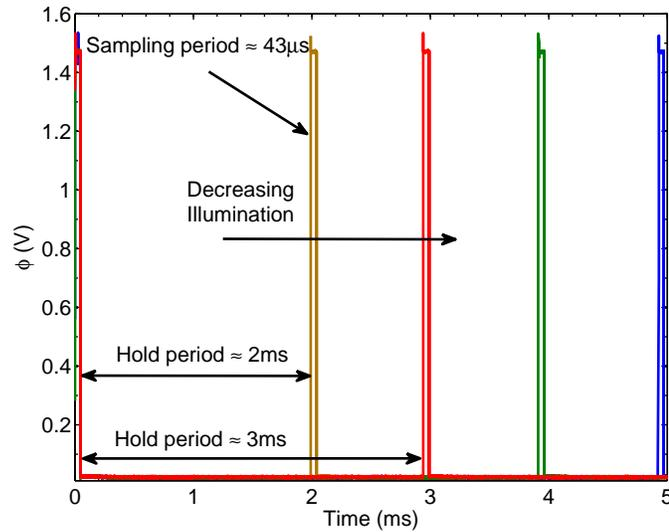
Figure 3.3 : Measured integrate and fire oscillator signal period for different illuminations.
