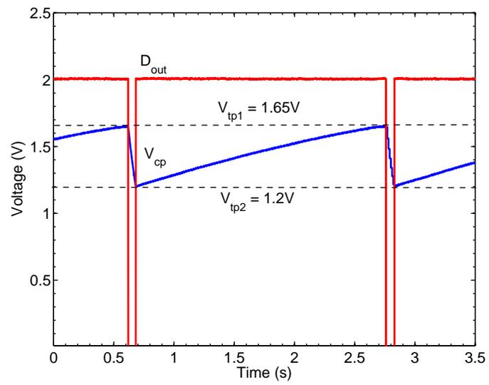
Figure 3.19 : Output voltage of the start-up ( $V_{cp}$ ) circuit and  $D_{out}$ .
