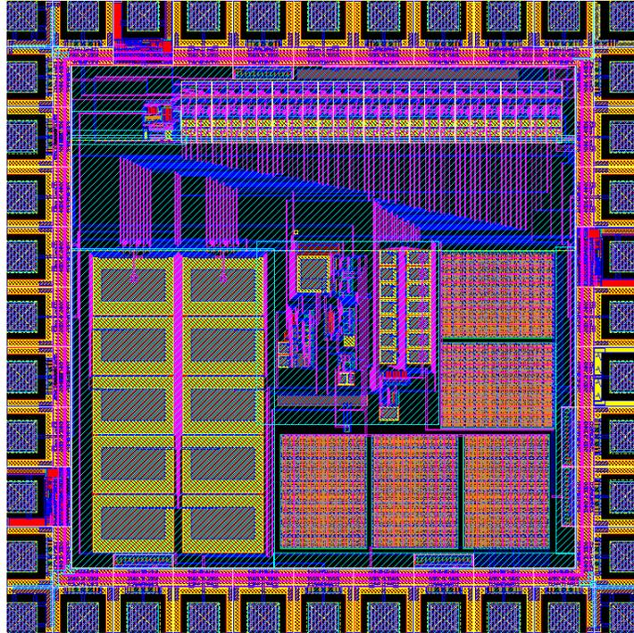
Figure 4.1 : Layout of the solar scavenging system sent to fabrication.
