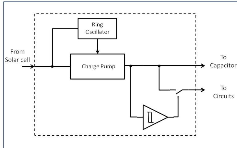
Figure 3.12 : Block diagram of the start-up circuit.
