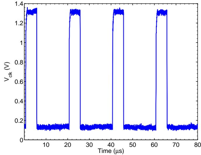
Figure 3.15 : Measured signal of the ring oscillator with respect a  $V_{DD}$  voltage of 1.5V and  $V_{Qclk}$  value of approximately -0.6V.
