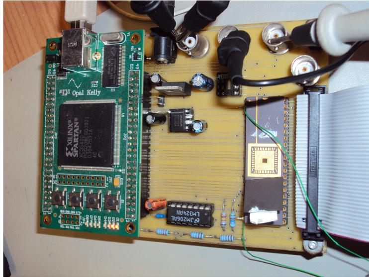
Figure 4.3 : Test board including the Spartan FPGA and the fabricated ASIC.
