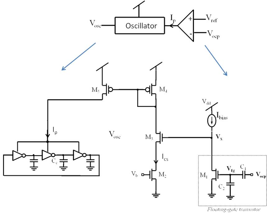
Figure 3.7 : Main oscillator feedback circuit
