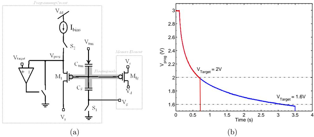
Figure 2.5 : Modified programming circuit for a solar powered system: (a) Schematic of a single programming unit (PU) for the solar energy scavenging system. (b) Programming of a single PU for different two different target voltages.
