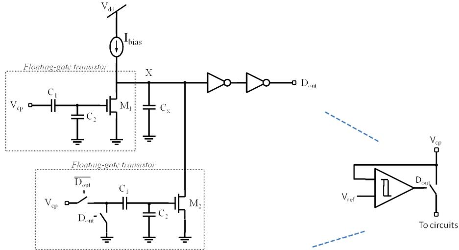
Figure 3.18 : Schematic of the hysteresis comparator.
