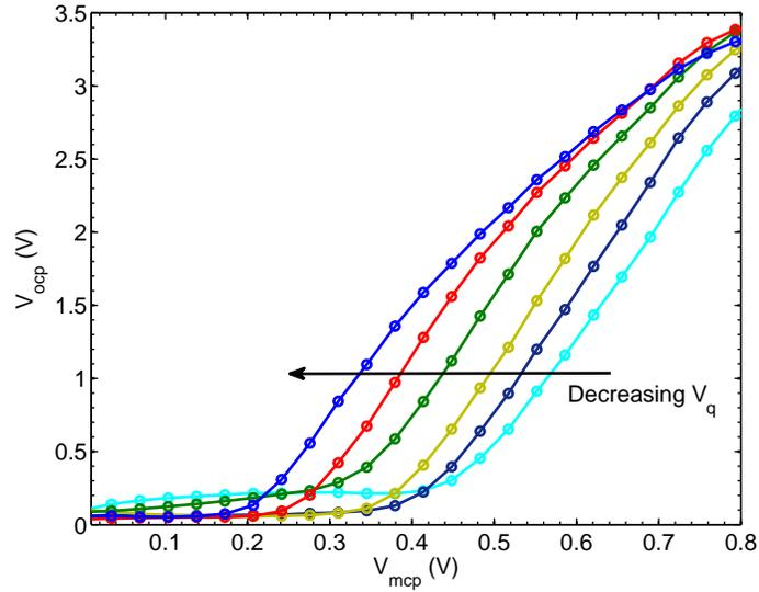
Figure 3.11 :  $V_{ocp}$  for an input voltage sweep for different  $V_q$  values.
