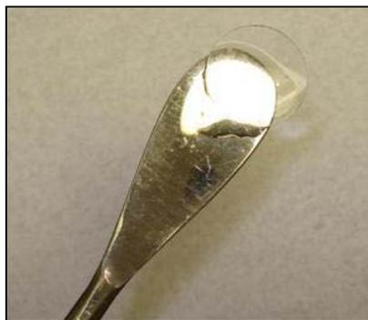
Figure 27: Hydrogels after circular disks have been sliced in order to equilibrate them in glutaric acid hydroxide buffer at several pH values.
