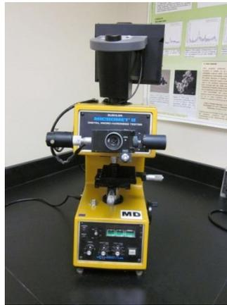
Figure 19 Microhardness Tester.
