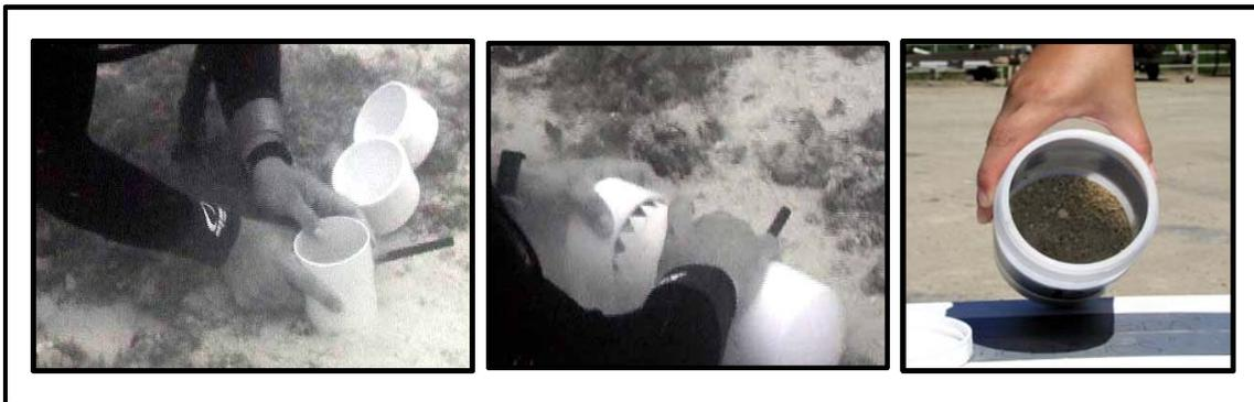
Figure 7. Process for taking core samples sediments. Note: the core sampler in this photo is larger than the actual core samplers used to take the sediment samples in this paper.
