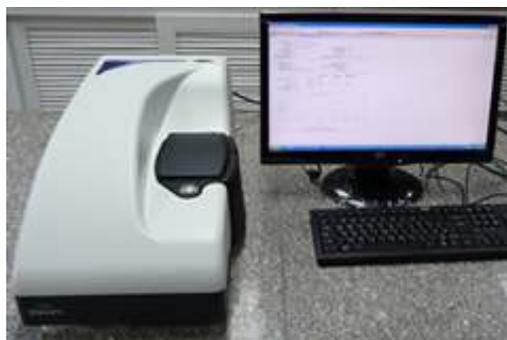
Figure 6. NanoS90 to measure of Z size and Z potential of Ag nanoparticles
