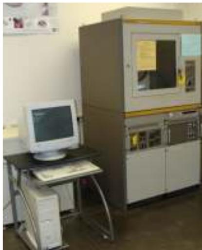
Figure 8. X- Ray Diffractometer Siemens D50
