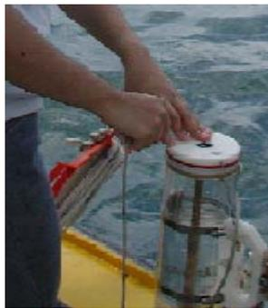
***Figure 4. Bailer sampler used for water collection at 10 ft.***
