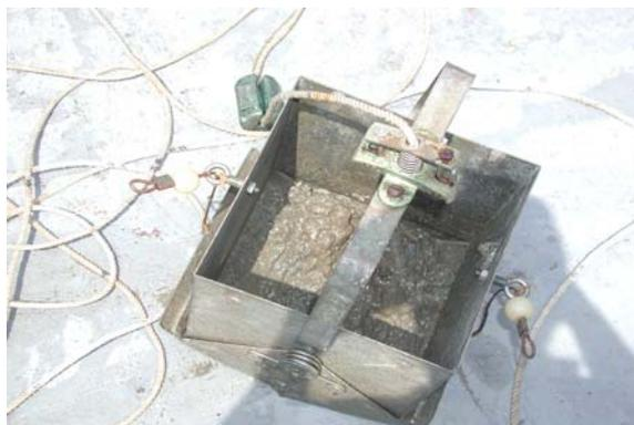
**Figure 2. Ekman sampler. This instrument was used to take samples of sand at 600 ft.**
