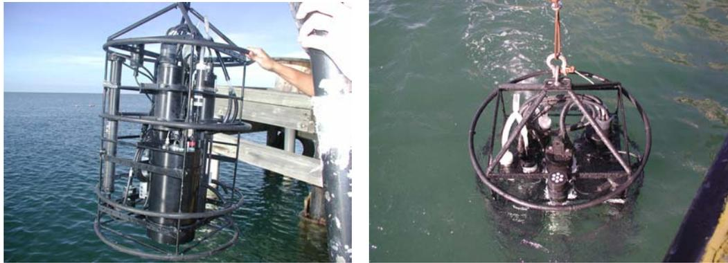
***Figure 3. CTD/rosette instrument to measure temperature, conductivity, fluorescence, transmissivity, and water samples for pH, salinity, and dissolved oxygen.***
