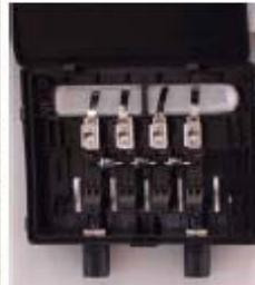
Tyco junction box with anti-error + and - connector. It is possible to connect cables up to 6 mm<sup>2</sup> (AWG 8). Includes three bypass diodes, these can easily be replaced. The SOLARLOK System does not use welded junctions, to minimise possible welding errors.
