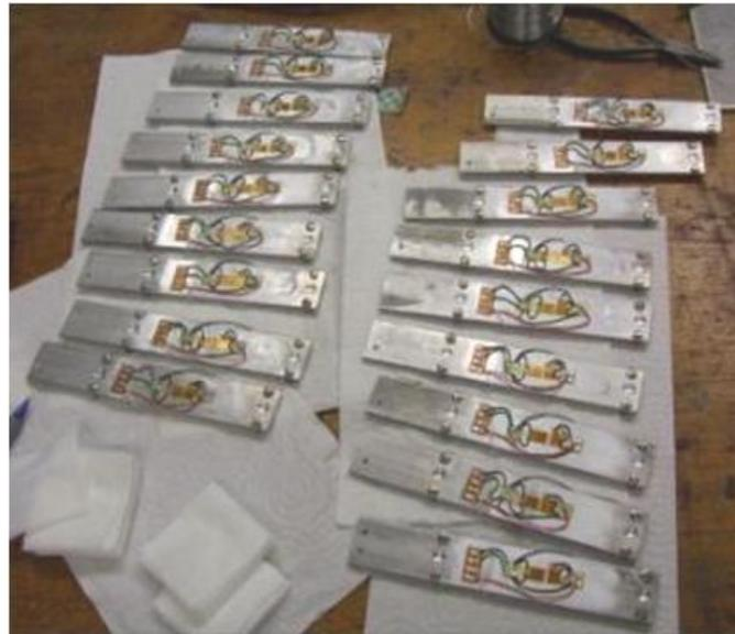
**Figure 27: Clamp-on transducers placed in the gate for strain measurements. Picture from Dr. Gopalaratnam's presentation "Strain Measurements and Numerical Investigation of Tainter Gate Operations".**
