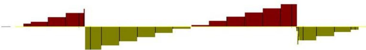
Figure 18: Shear diagram for girder W36x170. Drawing from ETABS v9.1.4.
