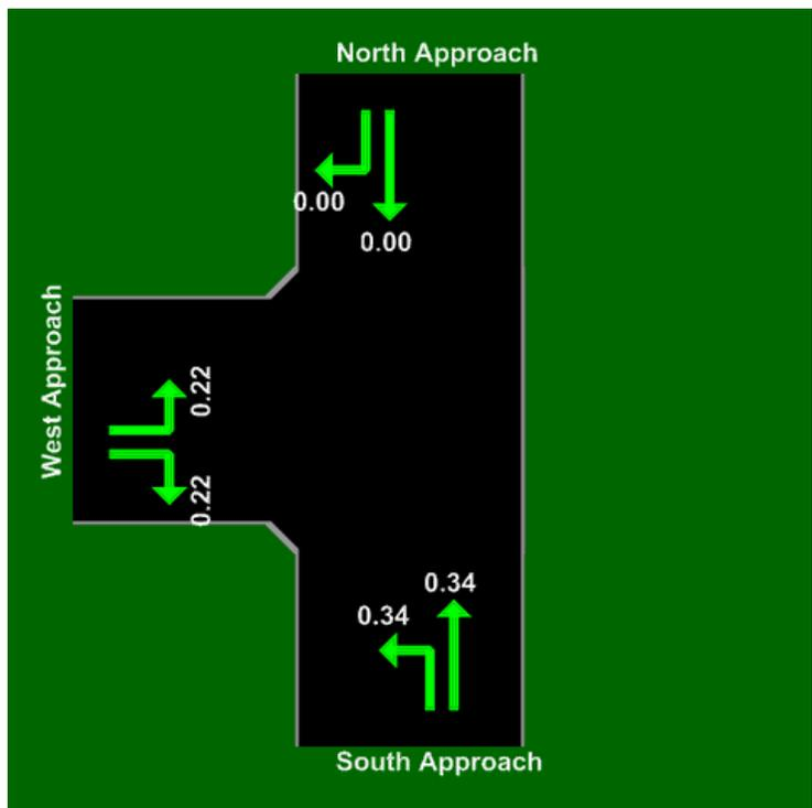
Figure 6-8 Queue Storage Ratio for Critical Gaps Found in the Field.
