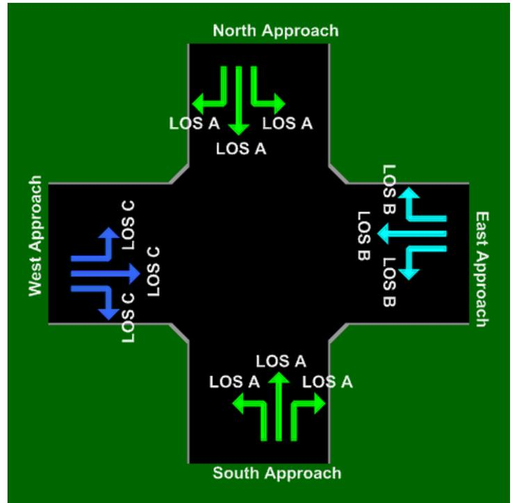
Figure 6-14 Level of Service for the Four Leg Intersection.
