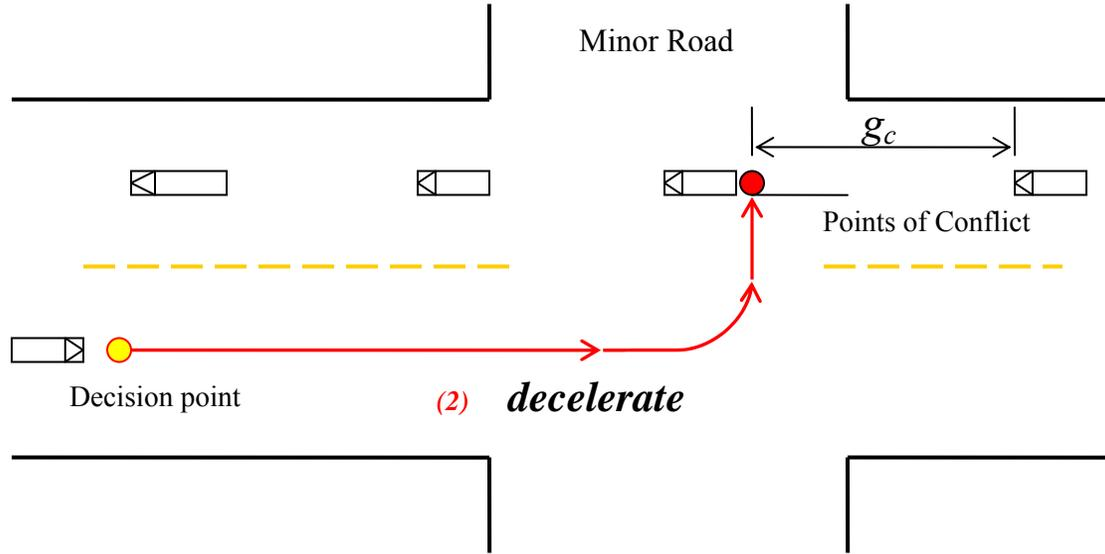
**Figure 5-11(2) Vehicle Decelerates Until a Desirable Gap is Provided.**
