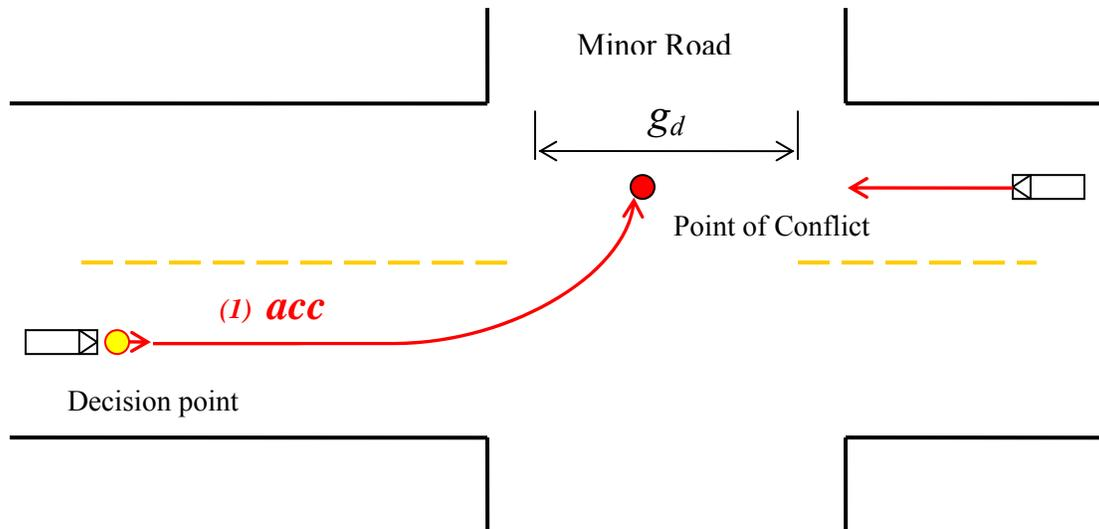
Figure 5-10 (1) Vehicle Accelerates and Enters the Intersection Aggressively.
