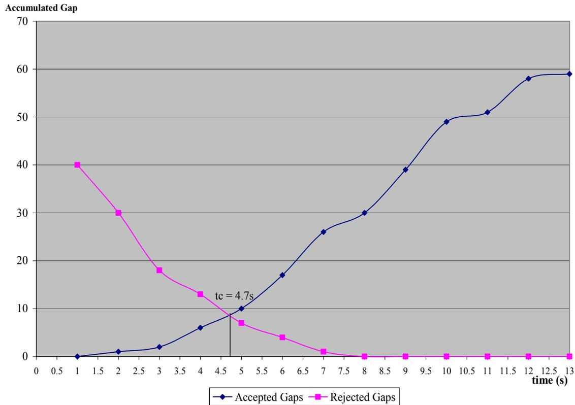
Figure 5-4 Critical Gap for Right Turns from the Minor Road
