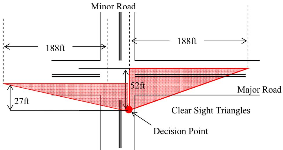
**Figure 5-7 Clear Sight Triangles for Left Turns from the Minor Road at Añasco.**
