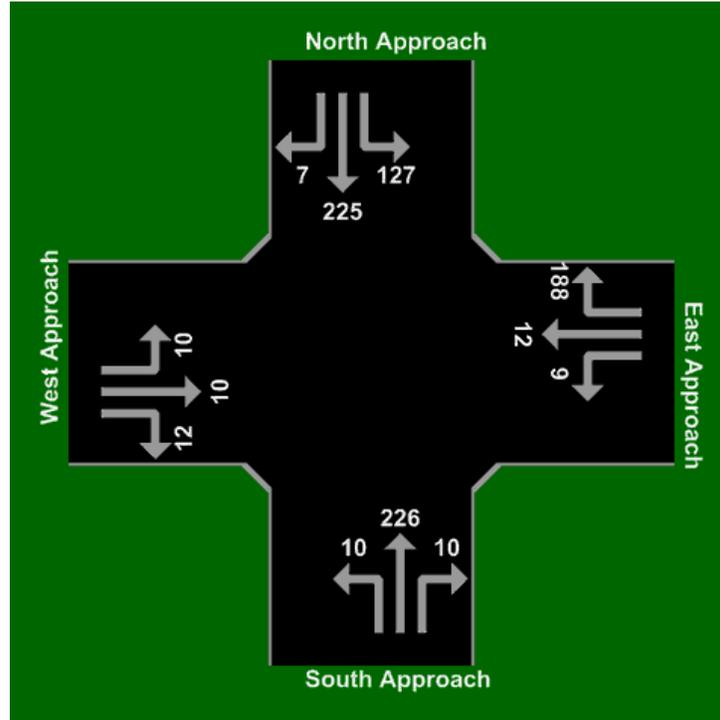
**Figure 6-11 Input Volumes in the Four Leg Intersection.**
