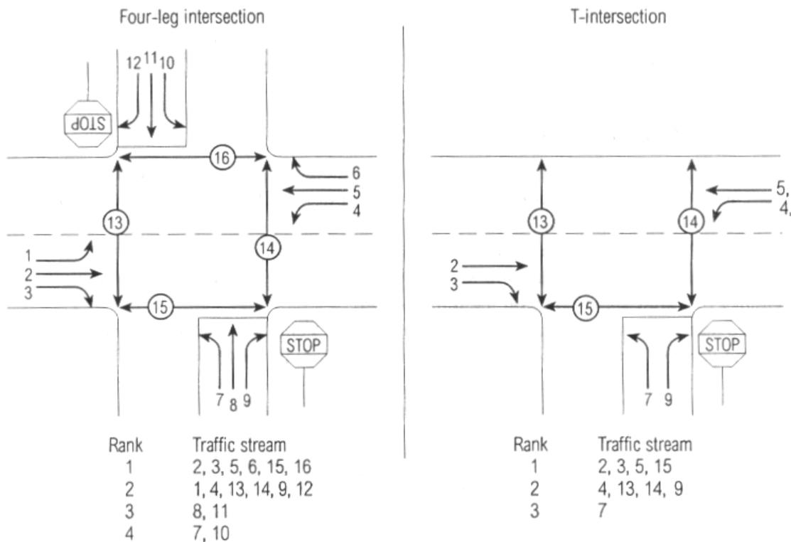
**Figure 2-5 Intersection Priority Diagrams for a TWSC.**
