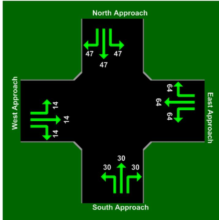
**Figure 6-12 Queue Distance for the Four Leg Intersection.**
