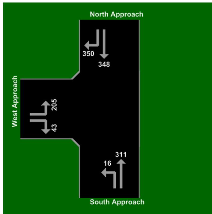
**Figure 6-3 Input Volumes in the Three Leg (T) Intersection.**
