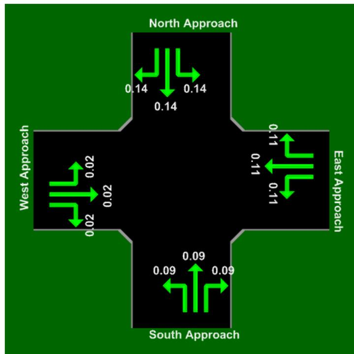
Figure 6-16 Queue Storage Ratio for Critical Gaps Found in the Field.
