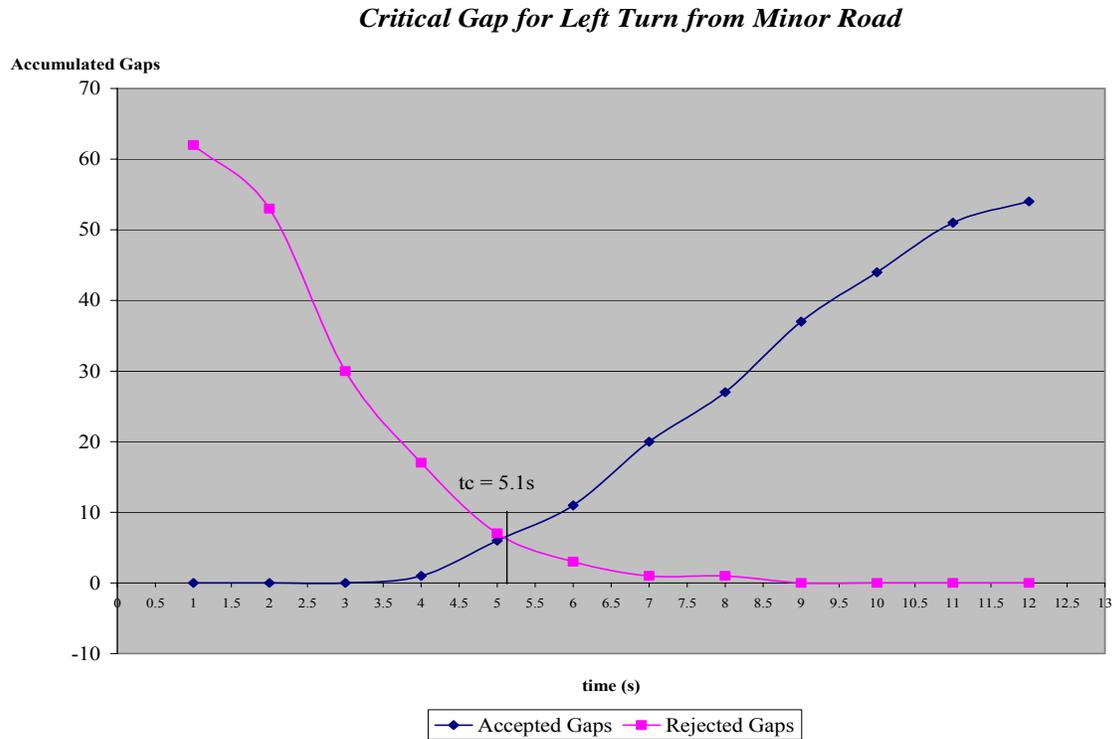
**Figure 5-2 Critical Gap for Left Turns from the Minor Road.**
