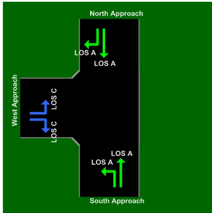
**Figure 6-9 Level of Service for Critical Gaps Found in the Field.**
