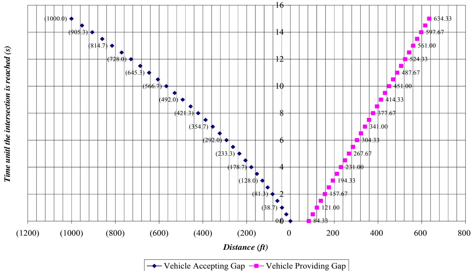
**Figure 5-15 Traveled Distance of vehicles approaching the intersection from opposing streams for a Minimum Gap of 2.3s**
