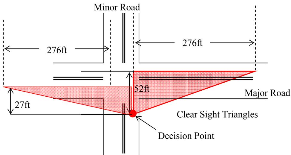
**Figure 4-2 Intersection Sight Triangles for Left Turns from the Minor Road.**
