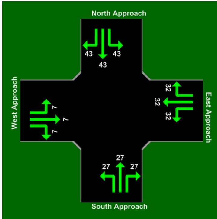
Figure 6-15 Queue Distance for Critical Gaps Found in the Field.
