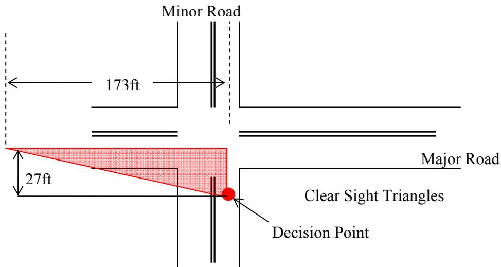
**Figure 5-8 Intersection Sight Triangles for Right Turns from the Minor Road.**
