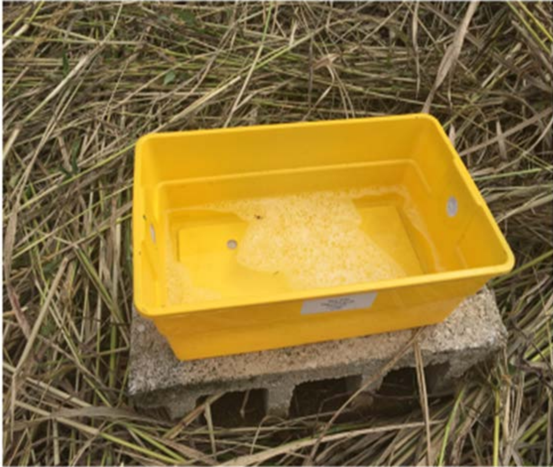
Figure 4. Möericke pan trap used for collecting alate aphid species in AAES and ES. Trap was placed above 0.30m of the ground in a concrete block. Two screened holes (diameter 25mm) were perforated in the two sides of the trap.
