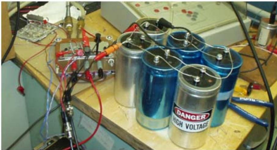
Figure 4.8: IPEM with all connections to the plate and bank of capacitors.
