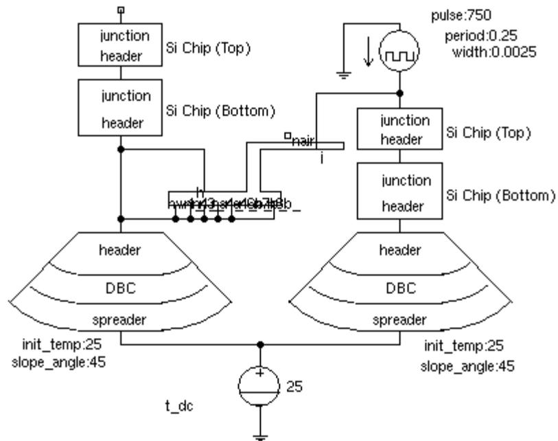
Figure 2.12: SABER double-chip simulation for the fast-transient test.
