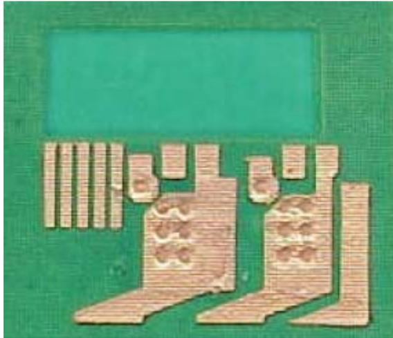
Figure D.5: Top metallization layer layout before any connections are made.
