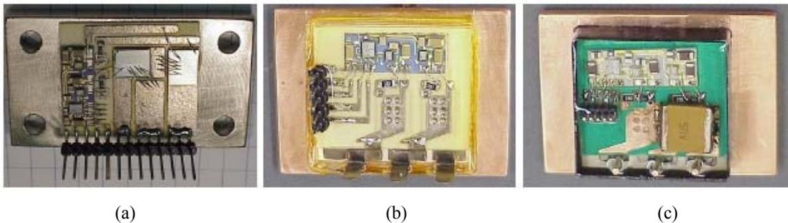
Figure 1.1: Some of the different CPES active IPEM prototypes.
