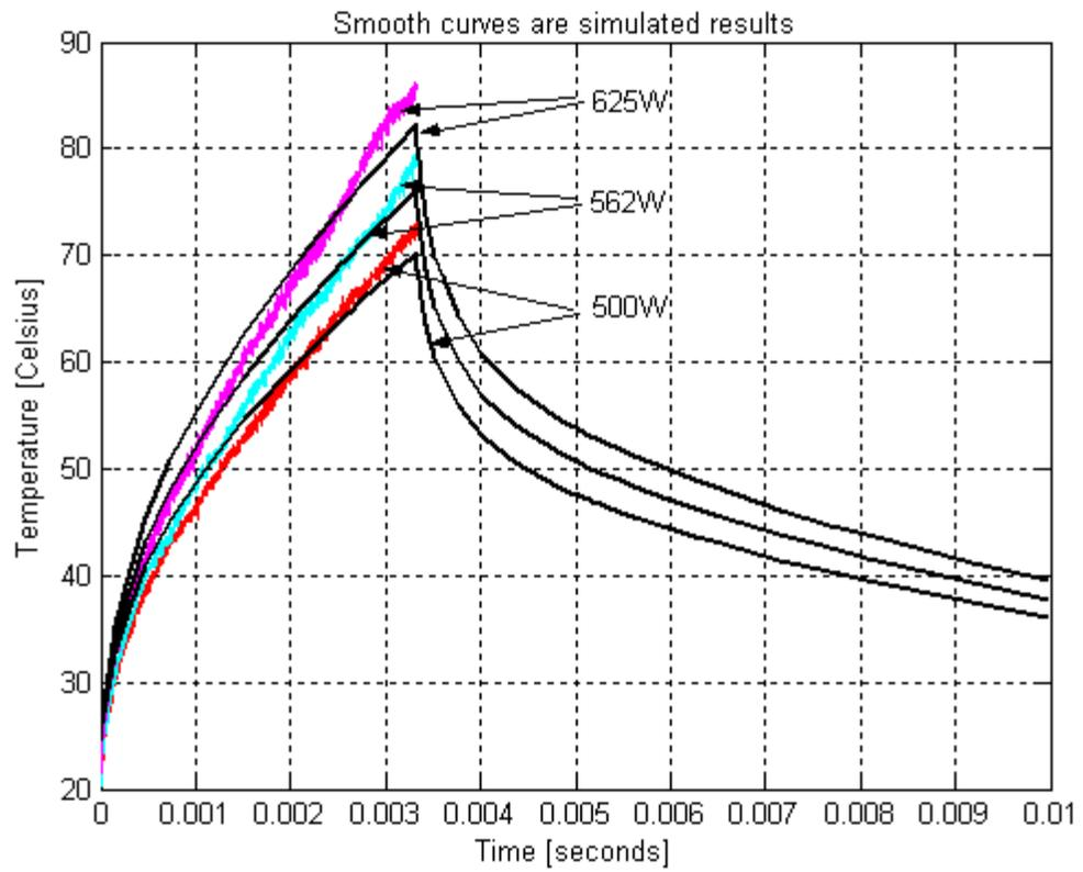
Figure 4.25: Single-chip results for the power levels with 3Hz frequency.
