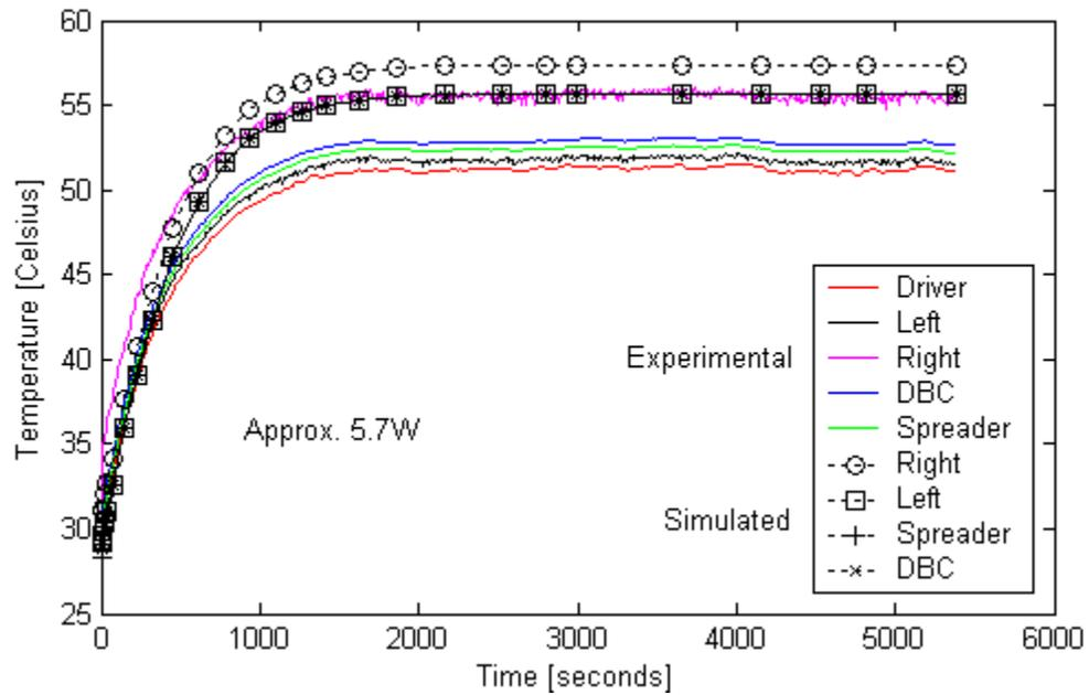
Figure 3.12: Slow-transient simulation results for 5.7W applied at the “right” chip.
