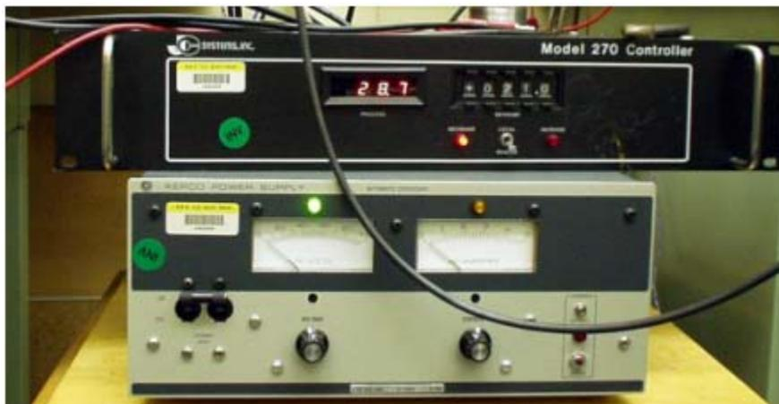
Figure 4.11: Temperature Controller (top) and 100V DC source (bottom) for the heating plate.
