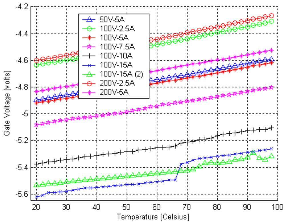
Figure 4.13: Experimental calibration curves for the *right* device at various power levels.
