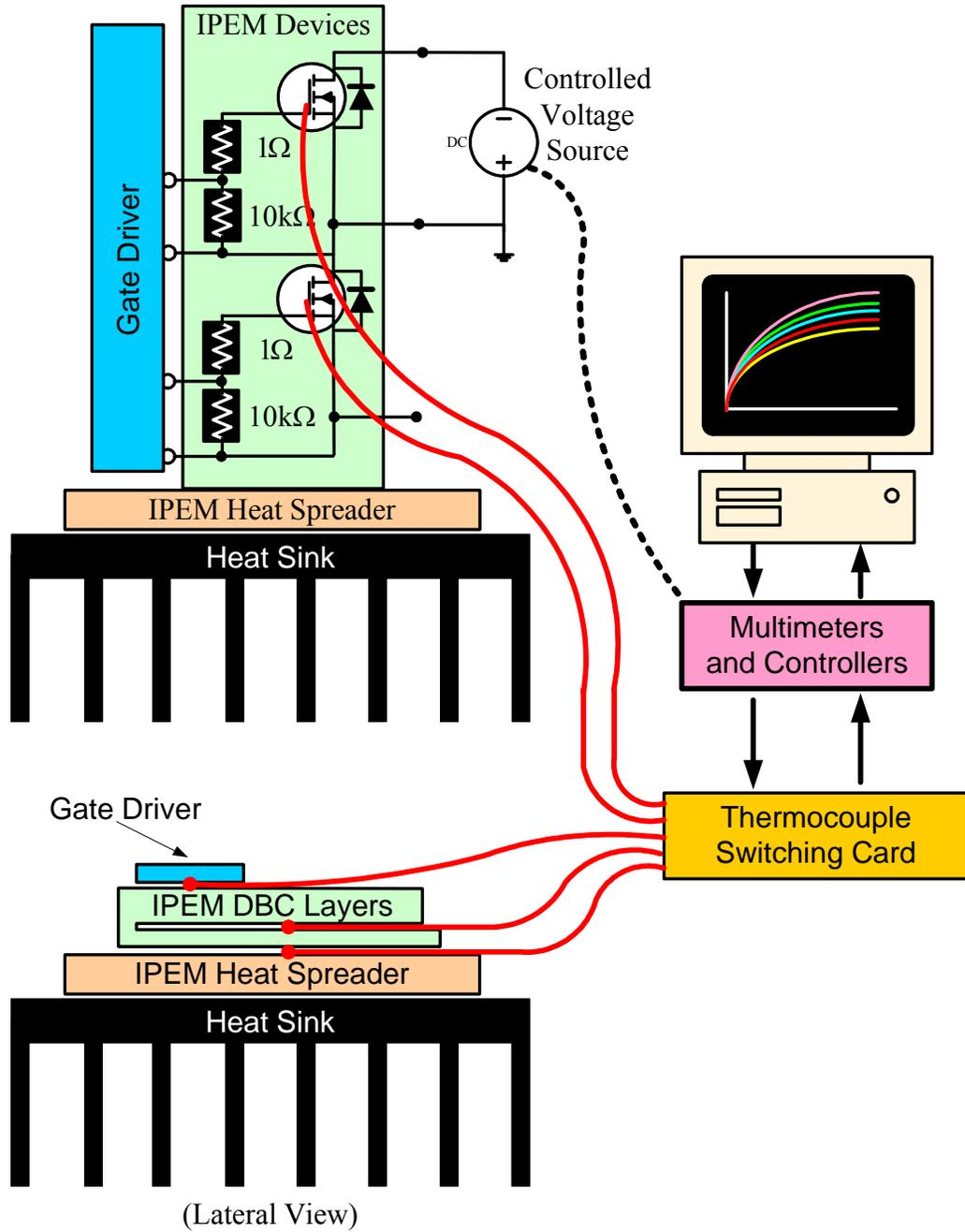
Figure 3.3: Slow-transient UPRM experimental setup.
