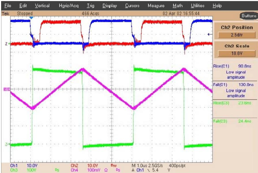
Figure 1.7: Output waveforms generated by the DC/DC converter with IPEMs. [Liang et al., '03]
