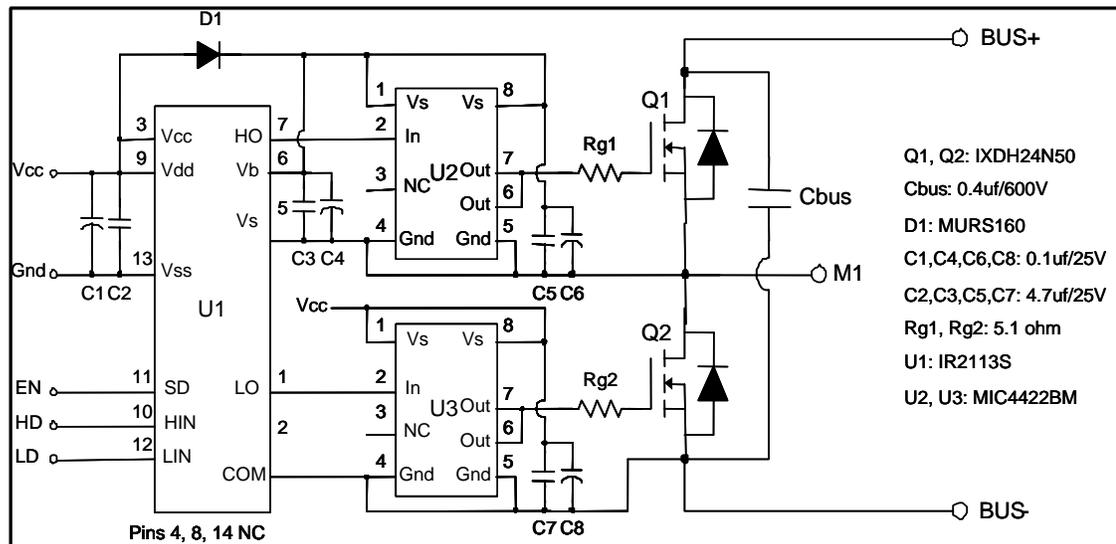
Figure 1.3: Schematic of the active IPEM.
