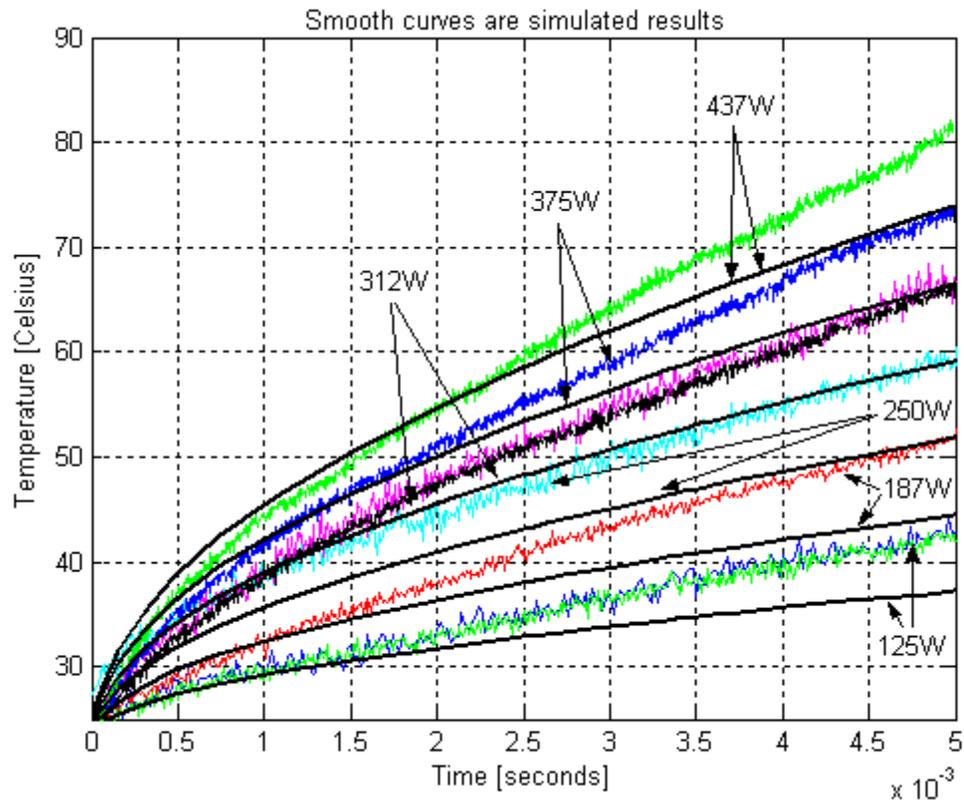
Figure 4.24: Single-chip results for the power levels with 1Hz and 2Hz frequencies.
