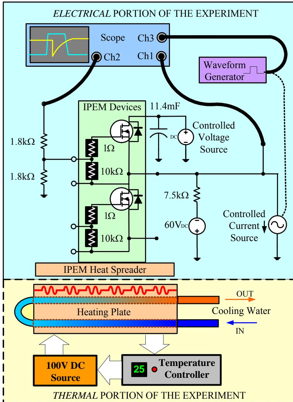
Figure 4.6: Schematic of the NIST experiment for the IPEM.
