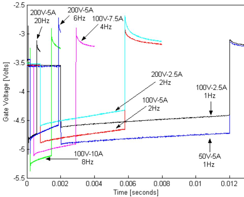
Figure 4.16: Left (top) and Right (bottom) transient voltage curves for various powers and frequencies.
