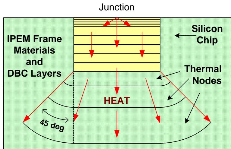
Figure 2.8: Thermal element decomposition of the IPEM into nodes.
