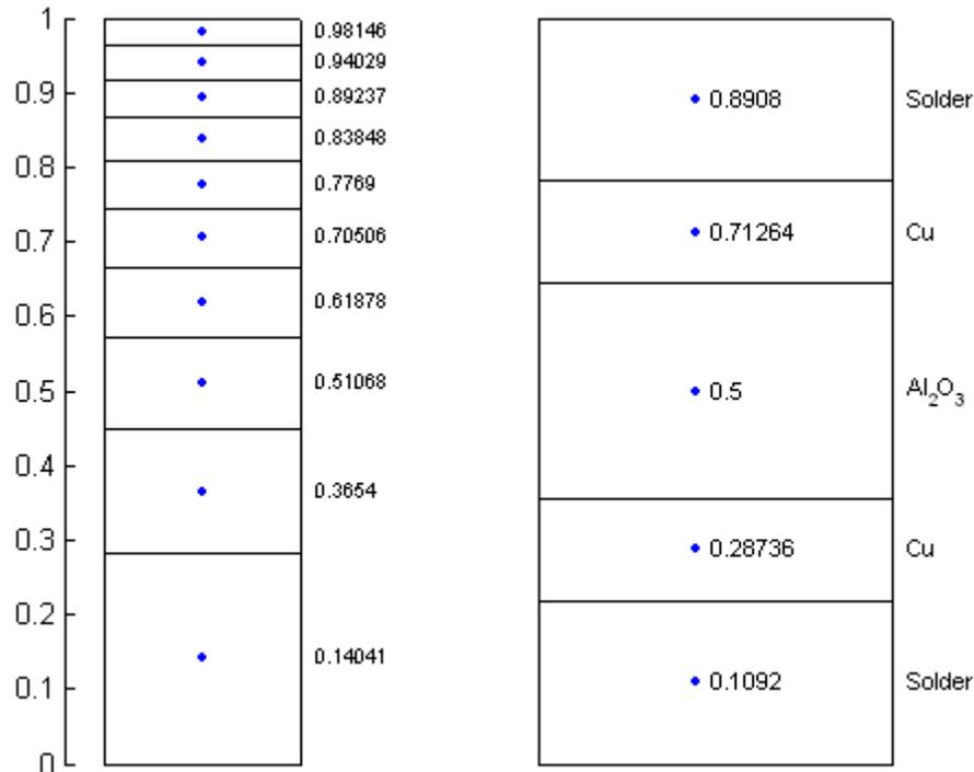
Figure 2.10: Relative location of the thermal components for the layers below the chip.
