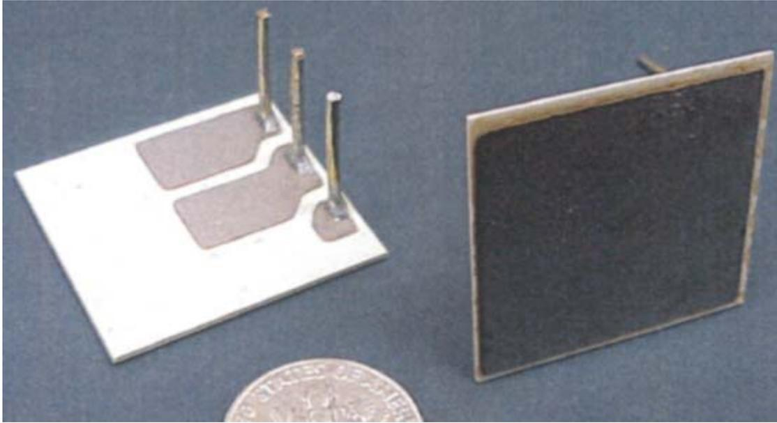
Figure D.1: DBC top metallization (left) and bottom soldering layer (right).
