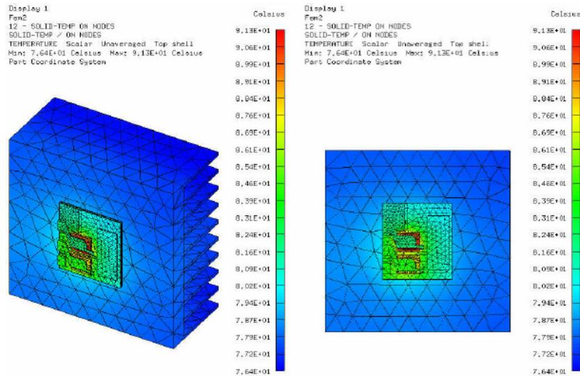
Figure 1.9: 3D temperature distribution at operational conditions simulated in I-DEAS. [Liang et al., '03]
