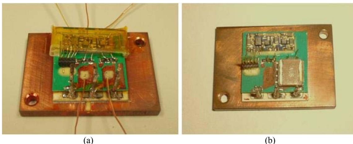
Figure 4.1: The two IPEM prototypes available for the electro-thermal experiments.
