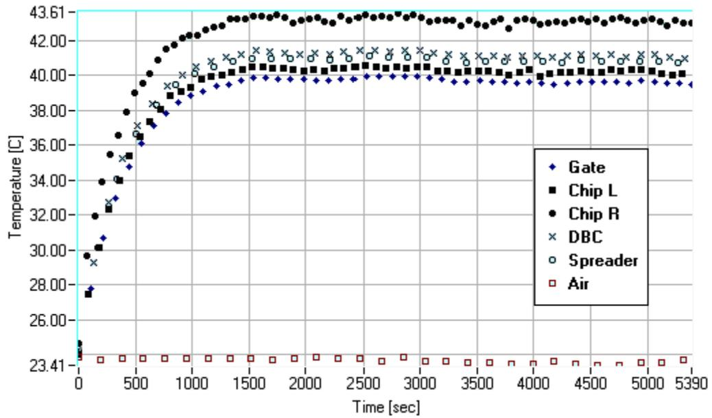
Figure 3.8: Experimental measurements in R with approx. 4.8W, 1.3V, 3.7A.
