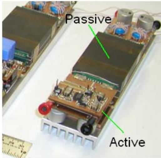
Figure 1.6: AHBC DC/DC converter. [Liang et al., '03]
