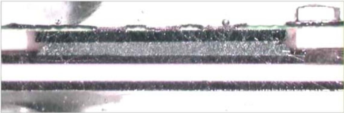
Figure 2.4: Cross-sectional view of the IPEM layers.
