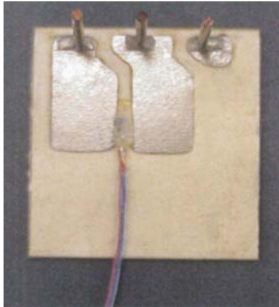
Figure D.3: Thermocouple placement for the DBC between chips.
