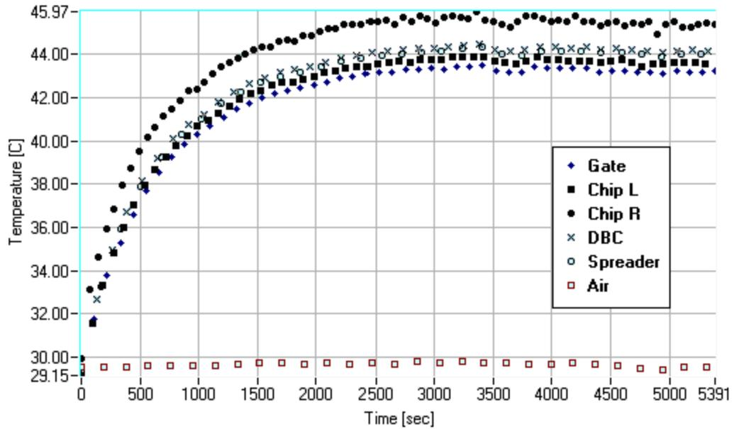
Figure 3.6: Experimental measurements in R with approx. 3.3W, 1.1V, 3A.
