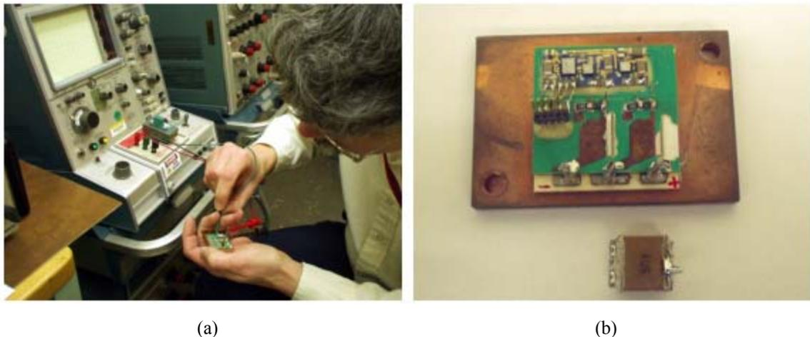
Figure 4.3: Curve tracer analysis (a), and bus capacitor already removed (b) from the IPEM.
