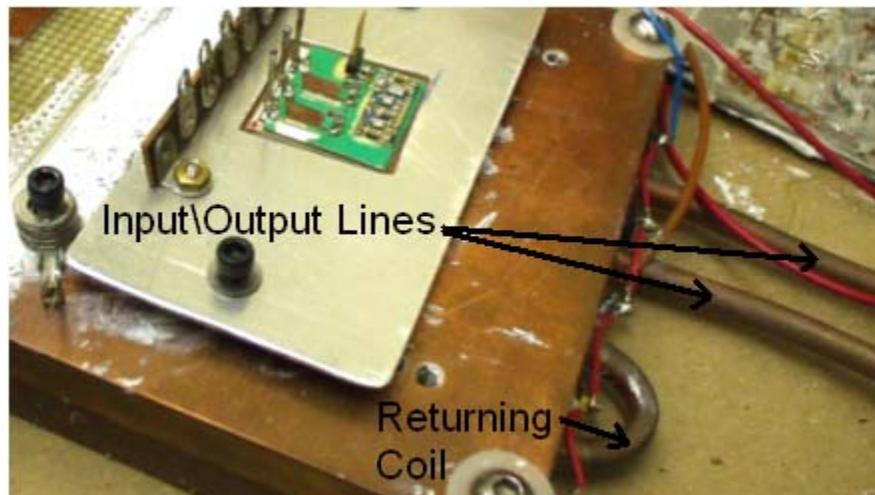
Figure 4.10: IPEM attached to the heat plate, showing part of the cooling pipes (right).
