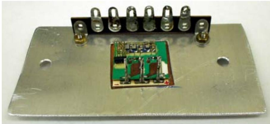
Figure 4.4: Drilled metal plate used as a supporter for more connections and to press down the IPEM.
