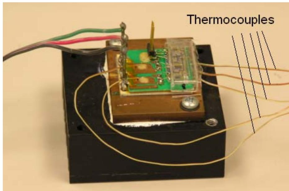
Figure 3.1: UPRM IPEM and heat sink experimental setup.
