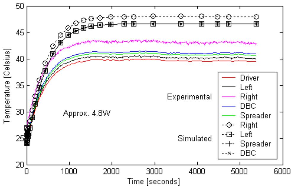
Figure 3.13: Slow-transient simulation results for 4.8W applied at the “right” chip.
