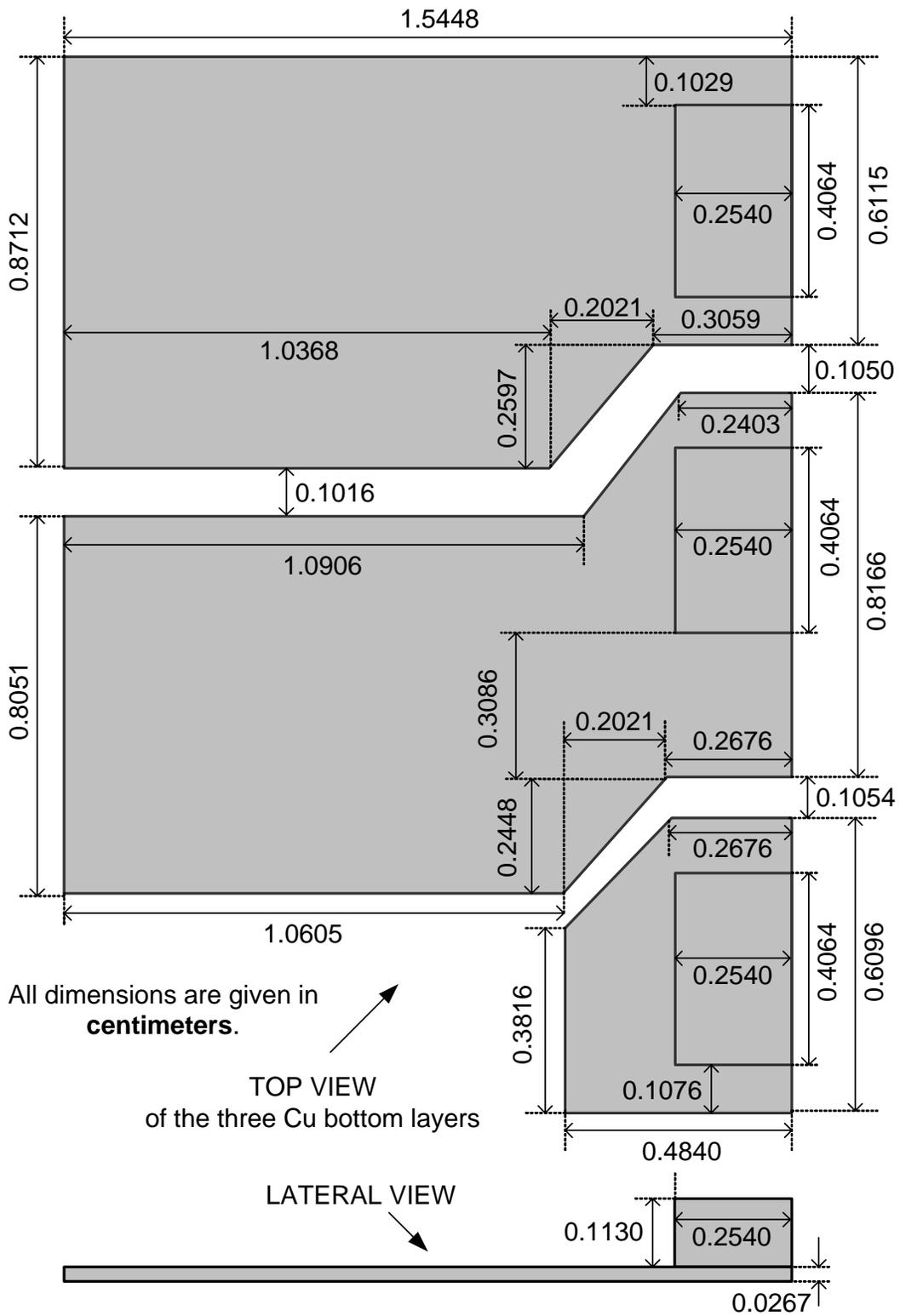
Figure A.5: Top DBC layer and contact leads.
