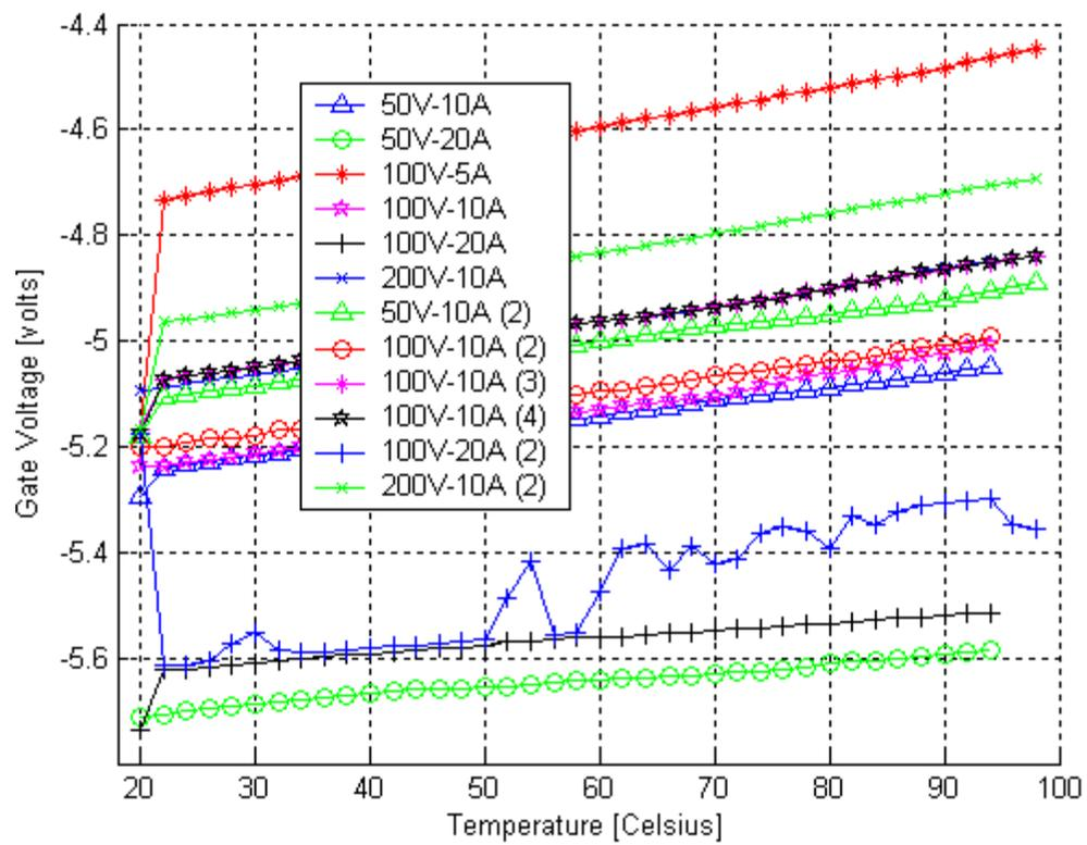
Figure 4.12: Experimental calibration curves for the *left* device at various power levels.
