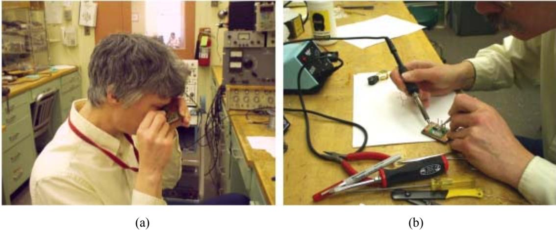
Figure 4.2: Visual inspection of the components (a), and bus capacitor unsoldering (b) for the IPEM.
