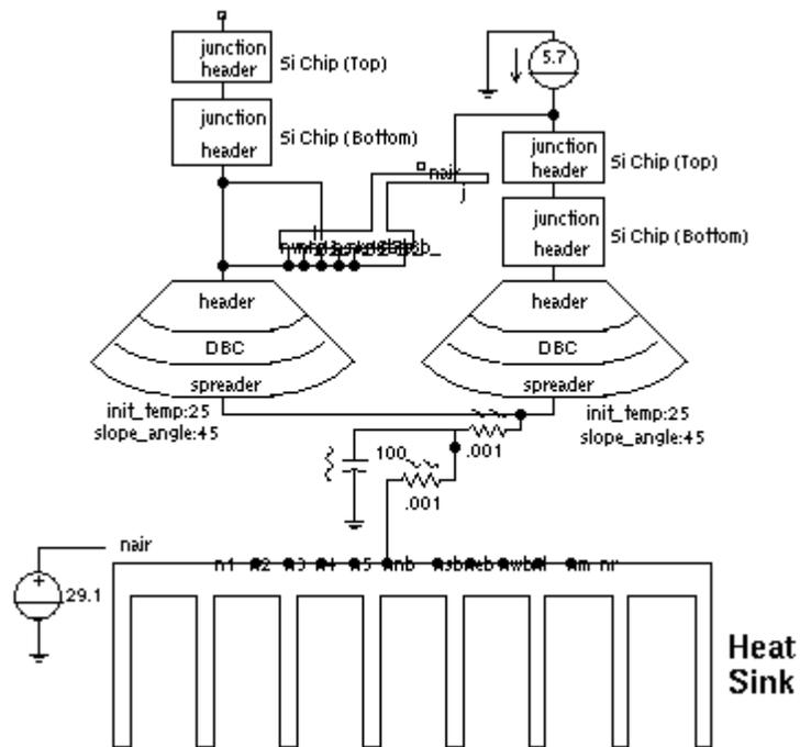
Figure 2.13: SABER simulation for the slow-transient test.
