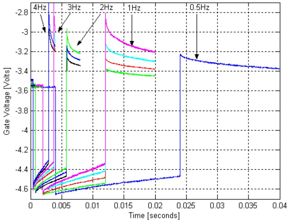
Figure 4.21: Oscilloscope readings for a family of 2.5A pulses at various frequencies.
