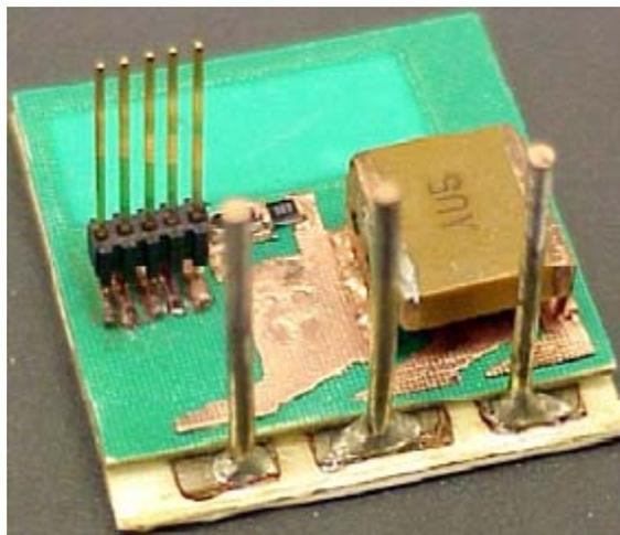
Figure D.4: Bus capacitor placement before gate driver addition.
