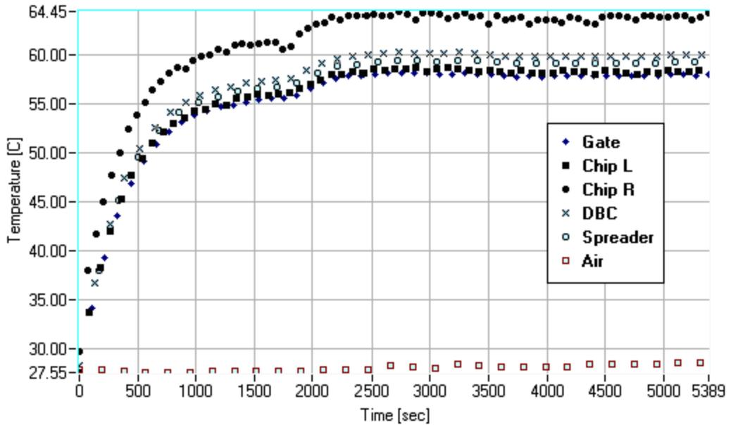
Figure 3.11: Experimental measurements in R with approx. 8~10W, 1.7V, 5.2A.
