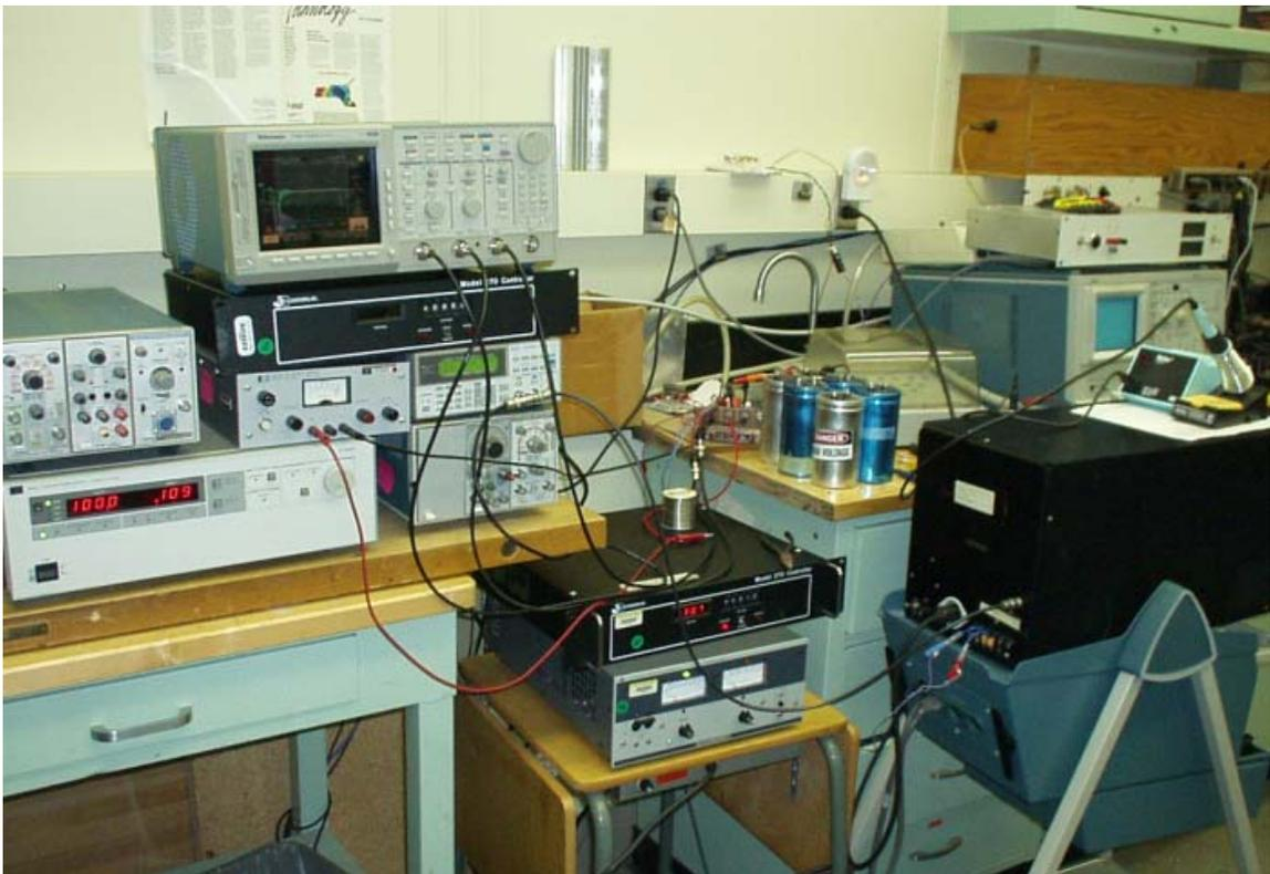
Figure 4.9: View of the complete fast-transient experimental setup at NIST.
