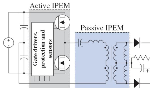
Figure 1.5: Schematic of an AHBC DC/DC converter based on IPEMs.
