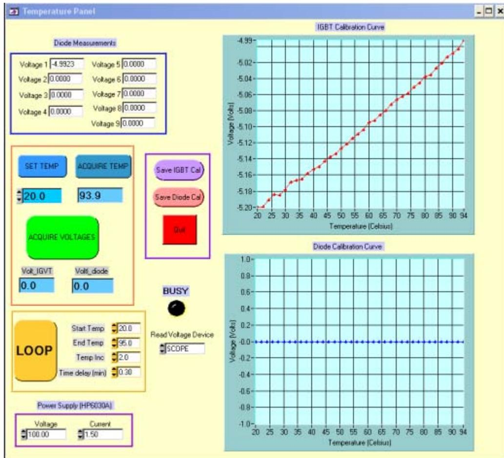
Figure D.7: Calibration curve acquisition tool environment. (For the fast-transient experiment)
