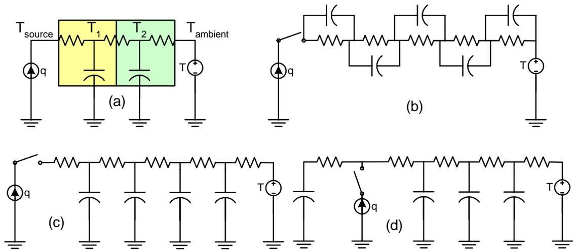
Figure 2.1: Example of one-dimensional thermal networks: (a) general approach; (b) Foster network; (c) Cauer network for a top uncovered device; (d) Cauer network for a top covered device.
