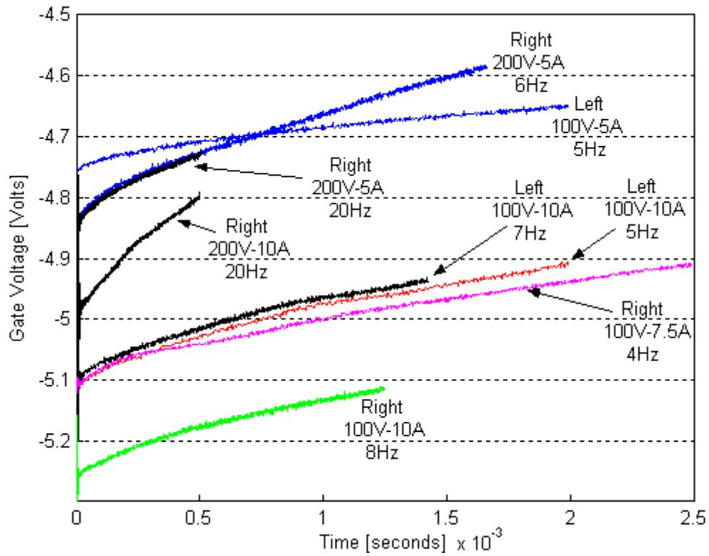
Figure 4.17: Isolated 4, 5, 6, 7, 8, and 20 Hz curvilinear pulse portions of the curves in Figure 4.16.
