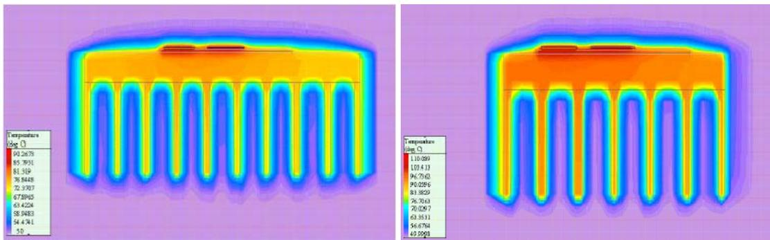
Figure 1.8: Different heat sinks FLOTHERM simulations used to analyze the IPEM thermal behavior. [Chen et al., '00]
