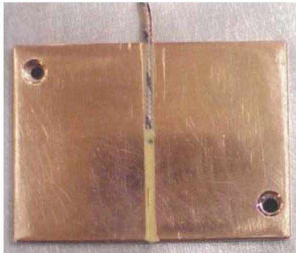
Figure D.2: Thermocouple placement for the heat spreader.
