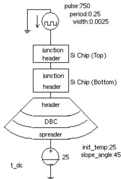
Figure 2.11: SABER single-chip simulation for the fast-transient test.
