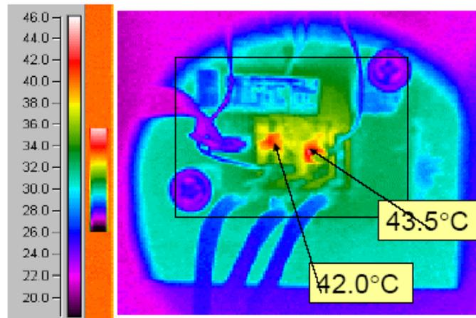
Figure 1.11: Thermal camera readings sample from the fully operational IPEM at VT. [Liang et al., '03]
