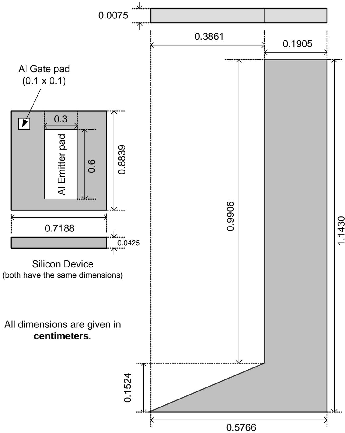
Figure A.4: Top right copper metallization trace and chips dimensions.
