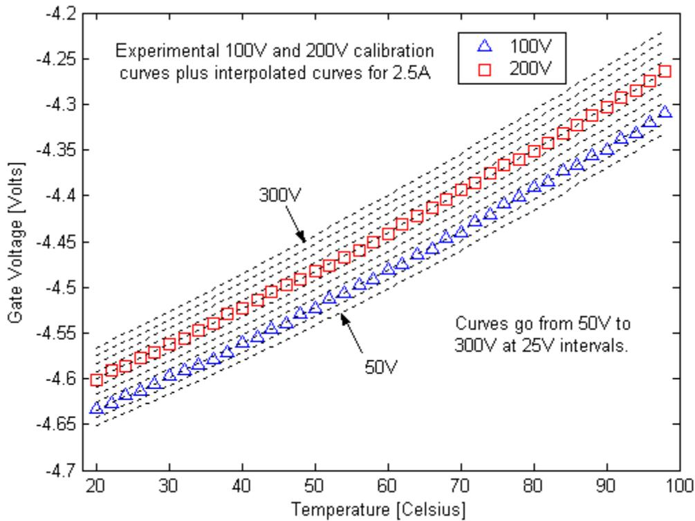
Figure 4.14: Generated family of 2.5A calibration curves for the *right* device.
