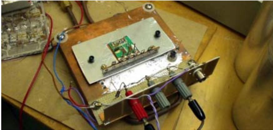
Figure 4.5: IPEM with holding metal sheet firmly positioned against the experimental heating plate.
