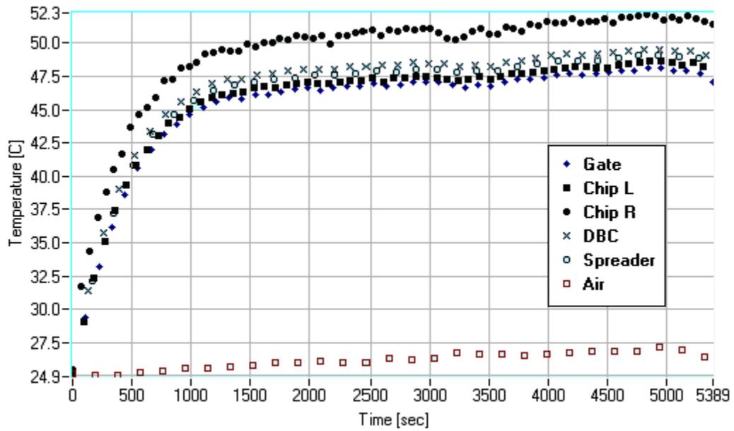
Figure 3.9: Experimental measurements in R with approx. 5.8W, 1.4V, 4.2A.
