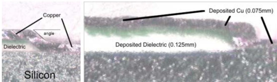
Figure 2.6: Close up of the deposited top copper metallization layer and dielectric.
