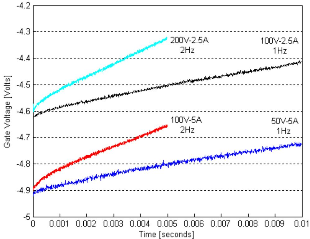
Figure 4.18: Isolated 1 and 2 Hz curvilinear pulse portions of the curves in Figure 4.16.
