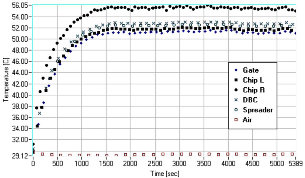
Figure 3.10: Experimental measurements in R with approx. 5.7W, 1.5V, 3.85A.
