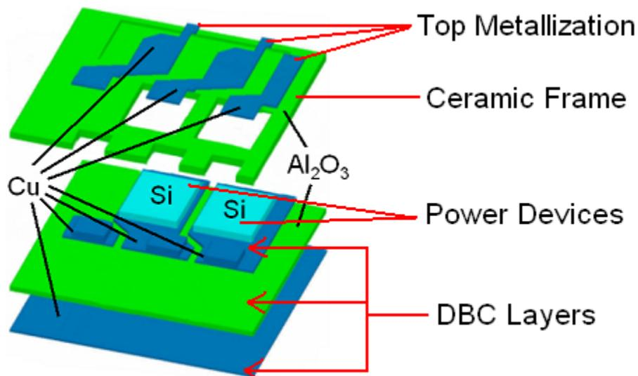
Figure 2.2: Exploded view of the CPES IPEM (Gen. II-C) layers and components.
