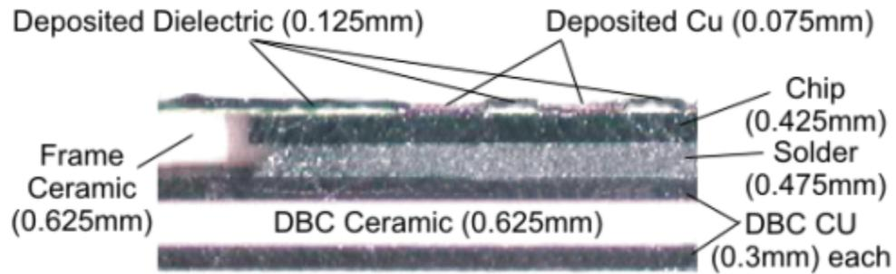
Figure 2.5: Identification of layer materials and thicknesses.
