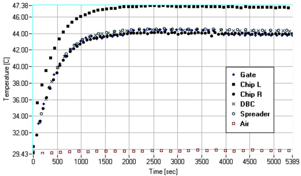
Figure 3.5: Experimental measurements in L with approx. 2.8W, 1.3V, 2.1A.
