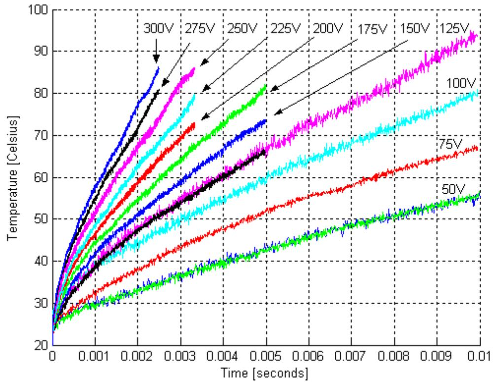
Figure 4.23: Equivalent temperature profiles for the gate voltage curves in Figure 4.22.
