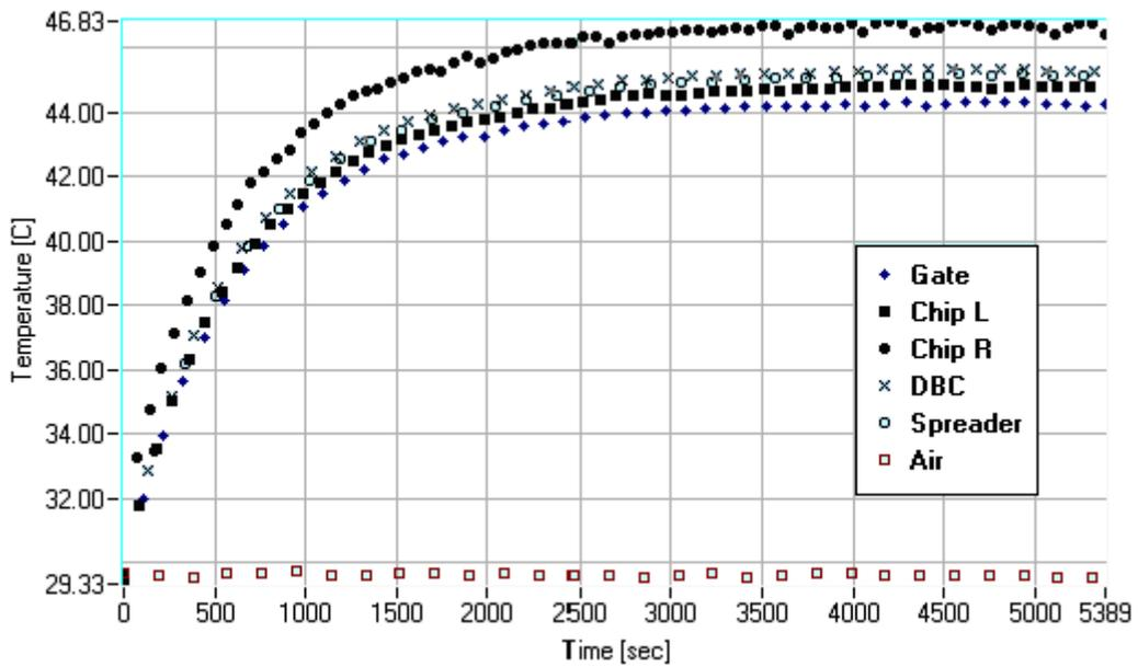
Figure 3.7: Experimental measurements in R with approx. 3.3W, 1.1V, 3A (#2).
