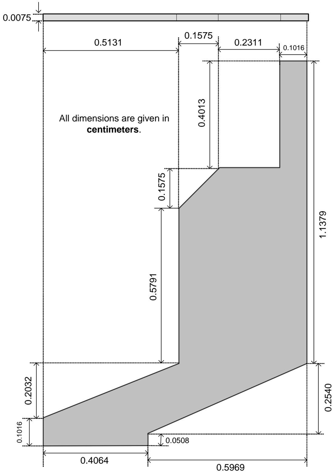
Figure A.3: Top left copper metallization trace.
