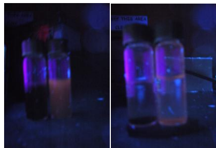
Figure 26: M-H curves for \text{Fe}_3\text{O}_4 (59.87 emu/g) and \text{Fe}_3\text{O}_4/\text{ZnO} (15.64 emu/g) nanoparticles (left) and photographs of the samples obtained by a UV lamp and a permanent magnet: \text{Fe}_3\text{O}_4 (black) and \text{Fe}_3\text{O}_4/\text{ZnO} (brown).
