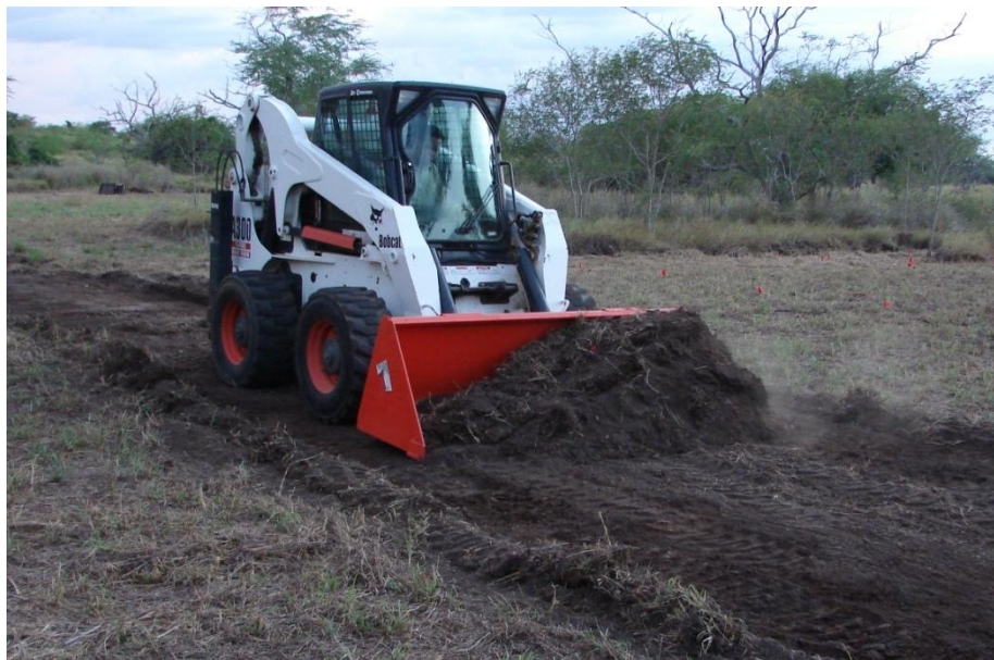
Figure 2.7. Photo of bulldozing effect with a Bobcat (A-300 Turbo). Removed 2-3 inches of soil surface.
