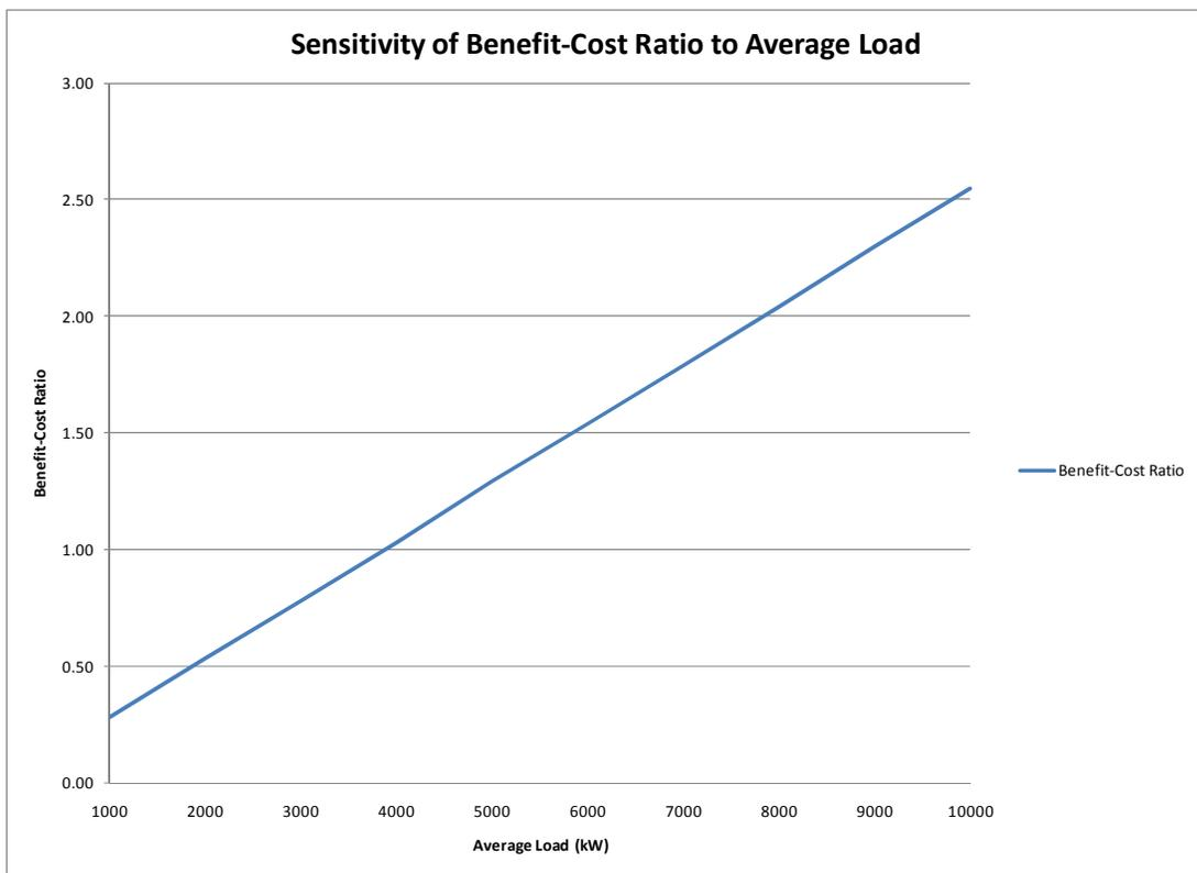
**Figure 4.5 Effect of feeder average load in the benefit-cost ratio**
