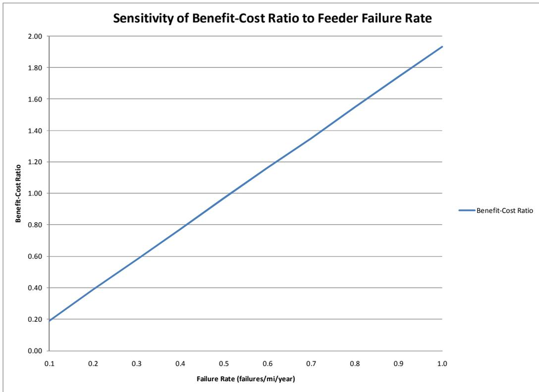
**Figure 4.3 Effect of feeder failure rate in the benefit-cost ratio**
