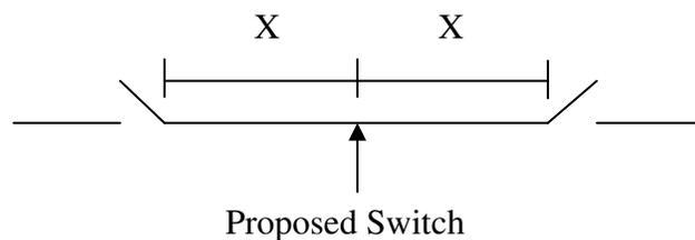
**Figure 3.2 Dividing a feeder into equally-spaced sections**
