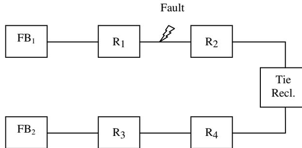
**Figure 2.1 Five-recloser loop sectionalizing scheme at Dominion**
