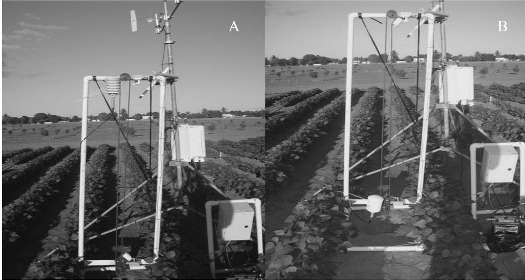
**Figure 5.1.** Automated elevator device developed for moving the Temp/RH sensor between the two vertical positions. **A.** Temp/RH sensor in up position and **B.** Temp/RH sensor in down position.
