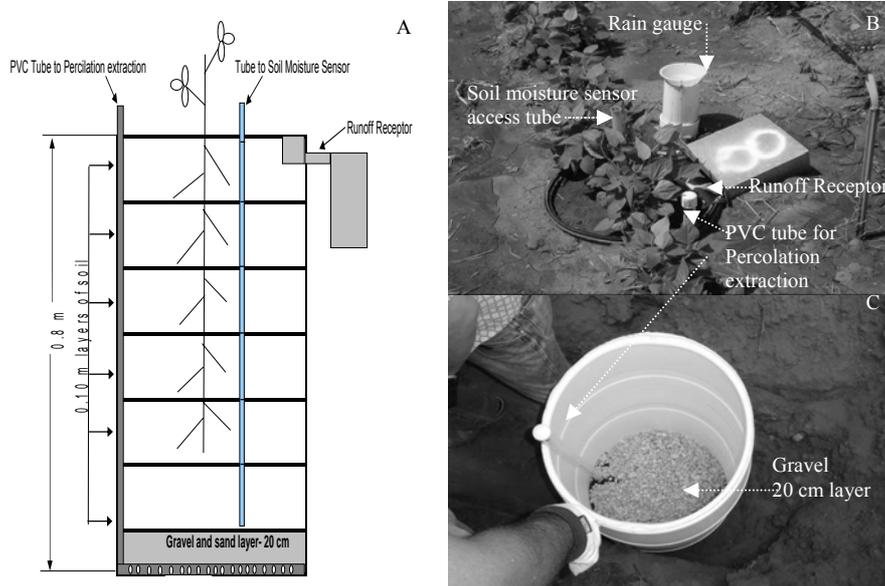
**Figure 4.3.** Drainage lysimeter installation: **A.** Cross section of the lysimeter, **B** runoff collector, soil moisture sensor, rain gauge, and depth percolation collector's overview, **C.** drainage system to depth percolation measurement.
