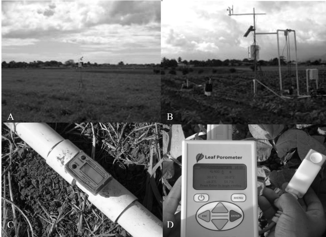
**Figure 4.4** A. Automatic weather station to estimate the reference evapotranspiration, B. ET station equipment and drainage lysimeter for crop evapotranspiration estimation, C. Flow meter in the principal irrigation lines and D. Leaf porometer equipment.
