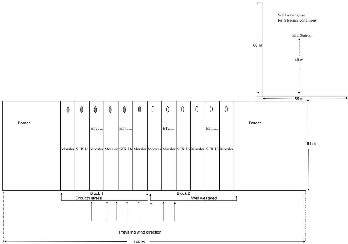
**Figure 4.1.** Experimental plot distribution, evapotranspiration station and lysimeter location. The circles are the lysimeters, arrange for 2006 experiment.
