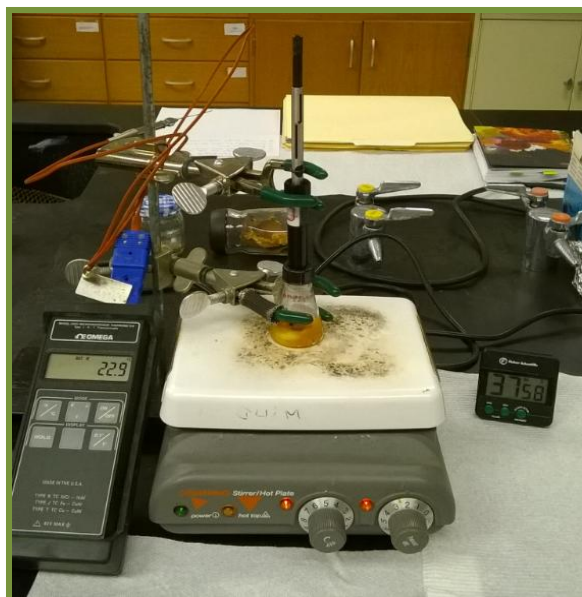
Figure 13. Head Space-Solid Phase Microextraction of the volatile constituents of Mammea Americana L. fruit pulp
