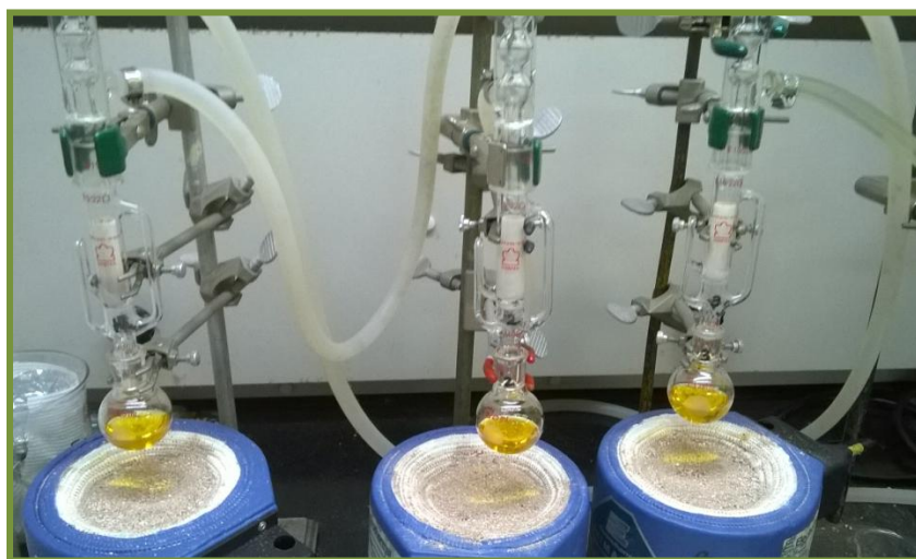
Figure 15. Microscale Soxhlet Extraction of the Essential Oil of Mammea Americana L. fruit pulp
