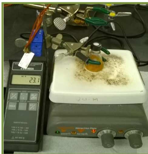
Figure 12. Mammea Americana L. fruit pulp at constant stirring reaching headspace/sample matrix equilibrium
