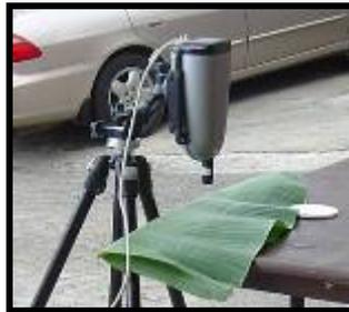
**Figure 3-1 Spectrometer Experiment Setup**
