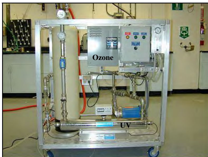
Figure 3-6: Field Unit UV/Ozone Treatment System Package Plant
