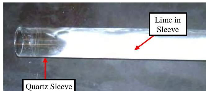
Figure 4-6: Quartz sleeve inside UV system
