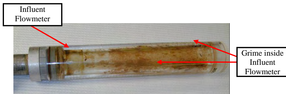
Figure 4-5: AOP plant influent flowmeter
