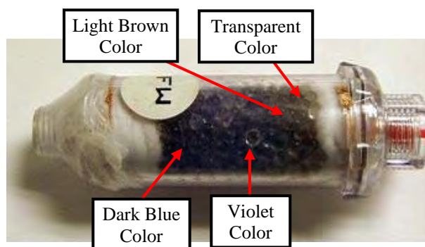
Figure 4-10: Particulate filter inside the ozone generator
