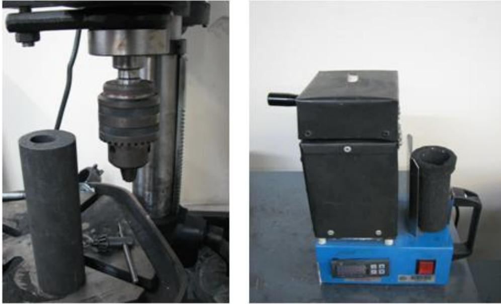
Figure 3–3: Mold, graphite crucible and furnace used for composite manufacturing
