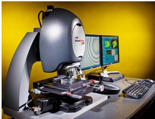
Figure 4-9: 3-D optical Zyo New View 6300 profilometer system
