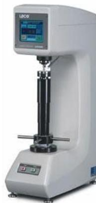
Figure 3-4: LECO LR-50 Rockwell hardness testing system
