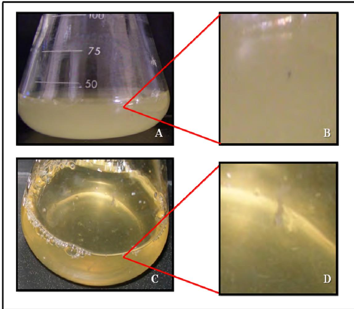
Figure 5.5 Amplification of phages in *E. coli* Rosetta strain. Figures A and B show an active culture of Rosetta strain  $OD_{600}$  of 2.5. Figures C and D correspond to a T7 phage infection culture Rosetta cultured at the same  $OD_{600}$ . When Figure B and D are compared, cellular debris is observed due to phage lysis to the Rosetta cells.
