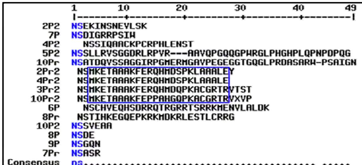
Figure 5.10 Alignment of the recombinant phages from human lung genomic library that were displayed using C77 cells as target. The blue box represents peptides that were displayed in the capsid of the recombinant phage, suggesting the presence of the nectin. Blue letters represent the only parts in which the alignment was the same in all sequences; P represents the isolated recombinant phages of lung; Pr represents the isolated recombinant phages of lungs after a repetition of the assay.
