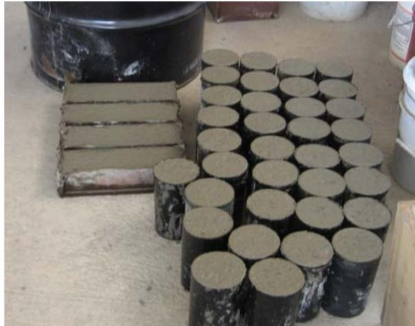
Figure 3-11 Specimens after filled.
