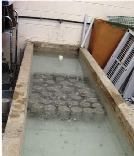
Figure 3-12 Curing tank with concrete specimens.
