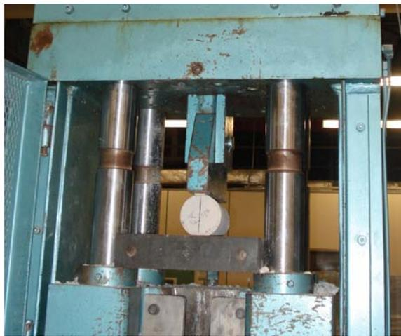
Figure 3-17 Splitting tensile strength test of concrete.
