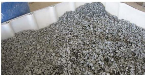
Figure 3-4 Coarse aggregate used.
