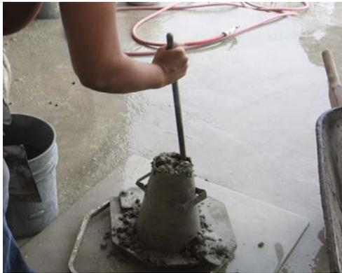
Figure 3-14 Slump test in fresh concrete.
