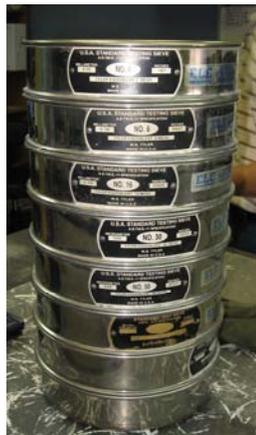
Figure 3-1 Sieves used for sand gradation.
