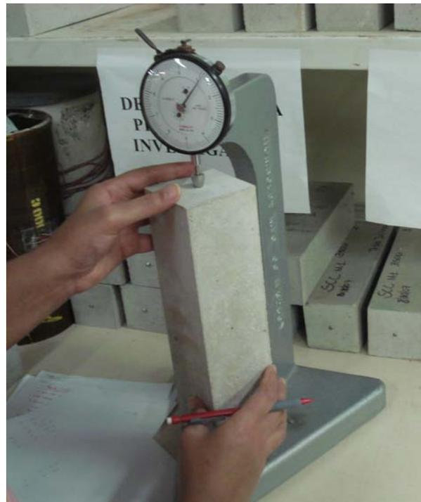
Figure 3-23 Free shrinkage test set up.
