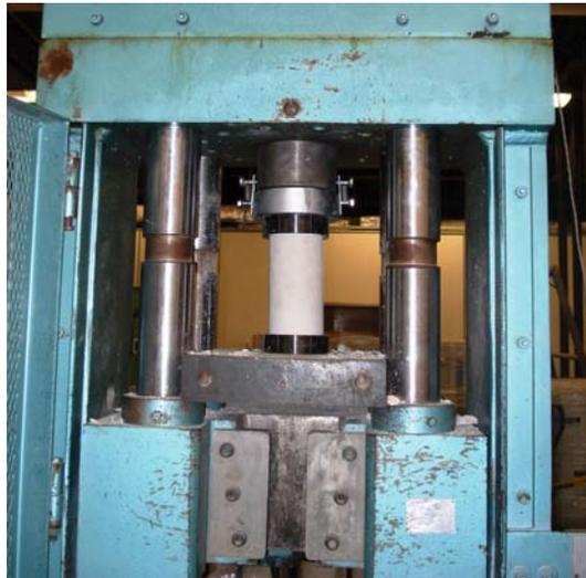
Figure 3-15 Compressive strength test of concrete.
