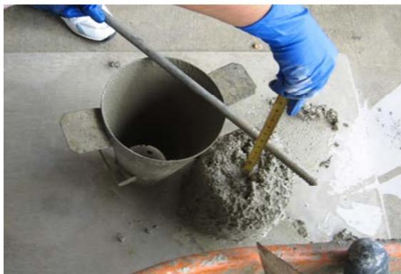
Figure 3-9. Slump test.
