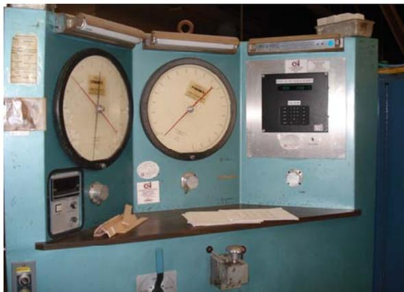
Figure 3-16 Load indicator of the compressive machine.
