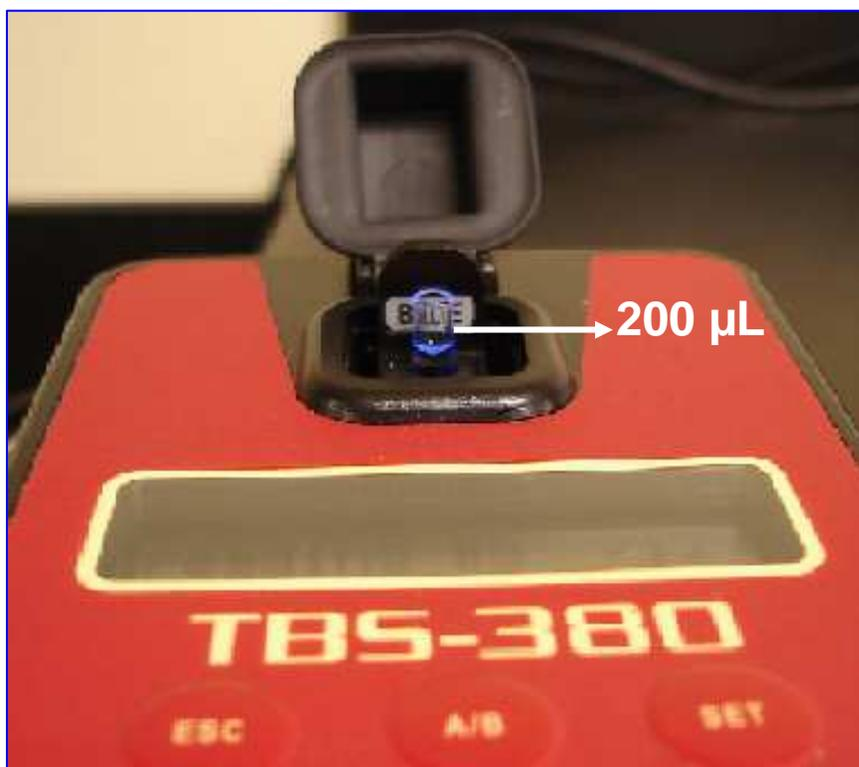
**Figure 3:** Picture showing the fluorometer and the mini borosilicate cell used in the fluorometric assay.
