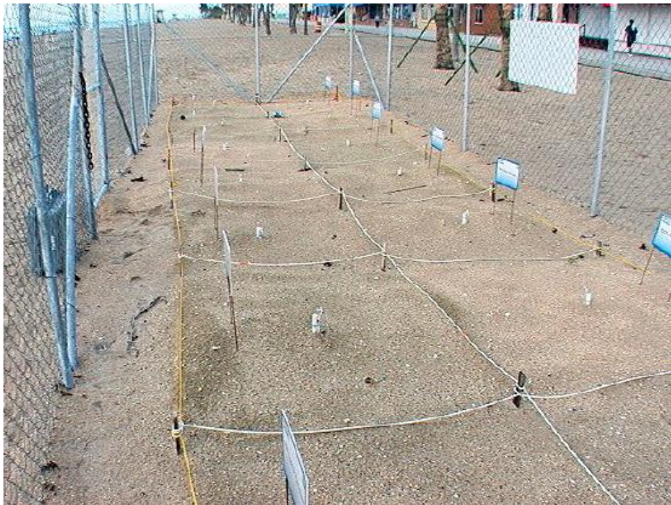
Figure 1.3: A view of tests conducted in 2006 by the City of Hollywood Beach, Broward County, Florida USA demarking varying proportions of glass cullets mixed with native beach sand ( Makowski, et al., 2007 ).
