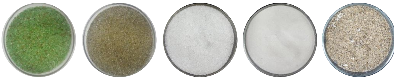
Figure 2.1: Types of crushed glass from Cay Clean Glass Plant (CGG), Ballotini (BL) and Rincón Native Sand (RNS); from left to right: CCG-10-20, CCG-20-40, BL-25-40, BL-50-70 and RNS.
