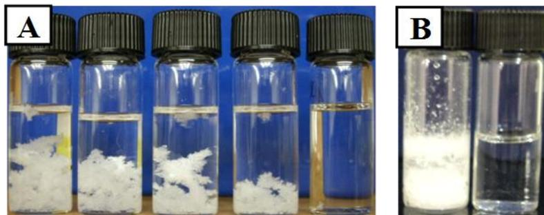
**Figure 2-15.** (a) Visual view of Acetone-Peroxide T-butyl Alcohol Reaction at 5:1, 4:1, 3:1, 2:1 and 1:1 T-butyl Alcohol: acetone ratio. The precipitated TATP is proportional to alcohol amount (b) Acid catalyzed AP-reaction and AP-reaction plus T-alcohol.
