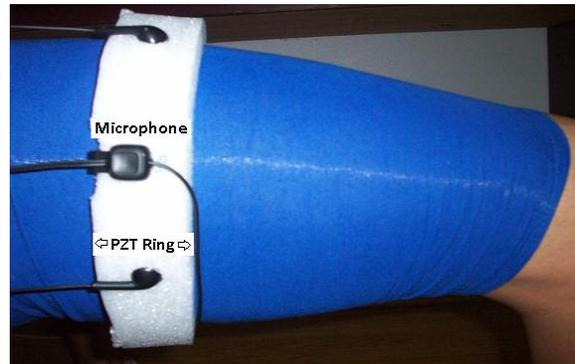
Figure 1-3 (a) Image of the proposed model, including microphone and piezoelectric ring, and general positional schematic (b) [National Institute of Technology and Evaluation, Osaka]
